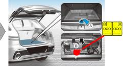
2. remove the clip (A) and release the cover (B)
