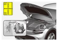
3. Battery in the engine compartment
