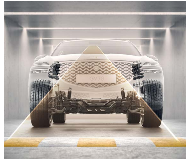
ELECTRONICALLY CONTROLLED SUSPENSION WITH ROAD PREVIEW
