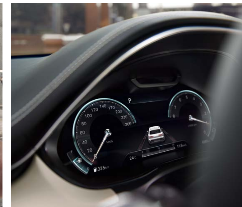
12.3" 3D TFT LCD DIGITAL INSTRUMENT CLUSTER
