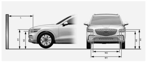
H1: Height between the headlight aiming centre and ground (Low beam)
