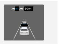
If you depress the accelerator pedal above a certain speed whilst Smart Cruise Control is operating, your vehicle can speed up temporarily without changing the set speed.
