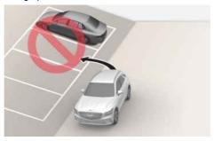
Remote Smart Parking Assist does not work normally on a inclined or curved road surface. Do not park even though the parking space is recognised by the sensor.
