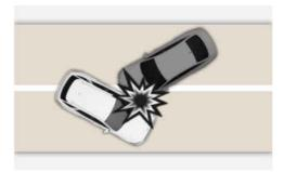
In an angled collision, the force of impact may direct the occupants in a direction where the airbags would not be able to provide any additional benefit, and thus the sensors may not deploy any airbags.
