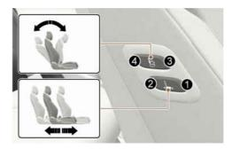
The rear seat passenger may use the switches to control the front passenger seat.
