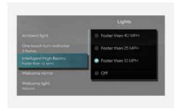
With the Start/Stop button in the DRIVE READY position, select Setup > Vehicle > Lights > Intelligent High Beams from the Settings menu to turn on Intelligent Front-Lighting System and deselect to turn off the system.
