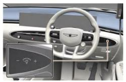
Press the illumination control switch to adjust the brightness of the instrument panel illumination.
