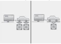
The tongue load is extremely important when setting up your trailer for towing with your vehicle. Excessive tongue load reduces front tyre traction and steering control. For example, too little tongue load can make the trailer unstable, causing the trailer to sway because the weight of the trailer is shifted to the rear.
