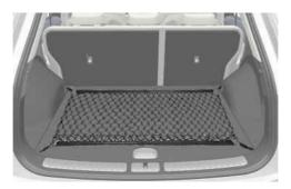
To keep items from shifting in the tailgate, use the 4 holders located in the tailgate side trim to attach the luggage net.
