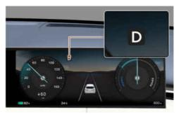
The gear shift indicator in the upper corner of the instrument cluster indicates the current rotary shifter position (D, N, R) or P (Park).
