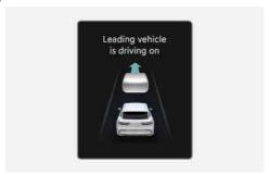
When a detected vehicle in front departs from a stop, Leading Vehicle Departure Alert displays the "Leading vehicle is driving on" message on the instrument cluster and an audible warning sounds.
