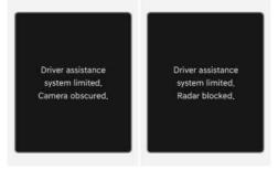
If the front view camera, front radar, bumper, or sensor is covered or blocked by foreign material, such as snow, rain, or dirt, or when a trailer or towbar mounted carrier is installed, the detecting performance may decrease and temporarily limit or disable Forward Collision-Avoidance Assist.
