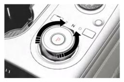
To shift the gear to N (Neutral), rotate the shift dial clockwise from R (Reverse) or counterclockwise from D (Drive) whilst depressing the brake pedal.
