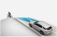
Forward Collision-Avoidance Assist may not detect other vehicles, motorcyclists, pedestrians, or cyclists in front of you whilst driving uphill or downhill, adversely affecting the performance of the sensors. A warning, brake assist, or steering assist (if equipped) may not be activated when needed.
