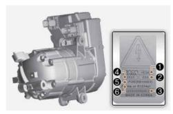
A compressor label informs you the type of compressor your vehicle is equipped with such as model (1), serial number (2), supplier part number (3), lot number (4), refrigerant oil (5) and refrigerant (6).
