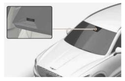
Auto defogging helps reduces the likelihood of fogging up the inside of the windscreen by sensing the moisture on the inside of the windscreen.
