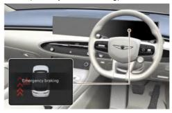
To warn you of a potential collision, the warning light on outside rearview mirror and head-up display (if equipped) may blink, a warning message may appear on the instrument cluster, an audible warning may sound, and the steering wheel may vibrate.
