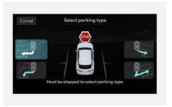
(1) Parking type - Perpendicular reverse (Left/Right), Parallel reverse (Left/Right), Diagonal reverse (Left/Right)
