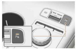
Press and hold the Parking Safety (P™) button more than 2 seconds, to turn the Parking Collision-Avoidance Assist on or off.
