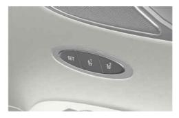
The Integrated Memory System for the seat allows the occupant to store and recall the following memory settings with a simple button operation.
