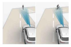
If a vehicle, motorcyclist, pedestrian, or cyclist is detected in the next lane or outside the lane when driving on a curve. Forward Collision-Avoidance Assist may warn you and may brake or steer (if equipped) your vehicle even when not needed.
