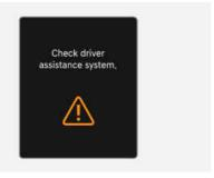
When Lane Keeping Assist is not working properly, the "Check driver assistance system." warning message may appear, and the yellow A warning light may illuminate on the instrument cluster. We recommend that your vehicle be inspected by an authorised retailer of Genesis Branded products.
