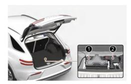
When replacing the battery, disconnect the negative (-) cable (1) and remove the positive (+) battery fuse box (2).
