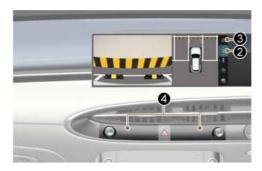
The front view appears on the screen when the gear is in N (Neutral) or D (Drive) to assist parking. The front view has top view, front view, side view, and 3D view.
