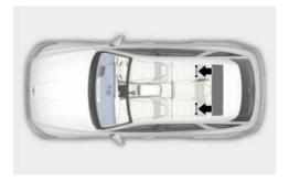
ISOFIX anchorages have been provided in the left and right outboard rear seating positions. Their locations are shown in the illustration. There are no ISOFIX anchorages provided for the centre rear seating position.
