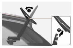
3 Install the new blade assembly by inserting the centre part into the slot in the wiper arm until it clicks into place (3).
