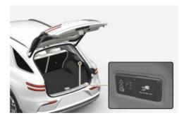
V2L(Vehicle to Load) is installed at the luggage compartment. V2L is a convenient feature which provides enough electricity to use diverse household electrical appliances in the vehicle.
