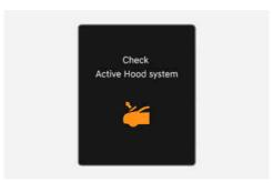
If there is a problem with the system a message will appear on the cluster display. This warning message means that the protection of pedestrians by the active bonnet lift system is not working properly. If the warning message is displayed, we recommend that
