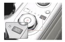
1 With the driver's door, bonnet, and tailgate closed depress the brake pedal and then press the AUTO HOLD button. The white HOLD indicator comes on and the system is in standby.
