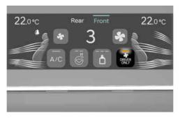
If you press the **DRIVER ONLY** icon (indicator light ON), most of the air flow is directed toward the driver's seat.
