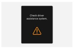
When Forward Collision-Avoidance Assist is not working properly, the "Check driver assistance system." warning message may appear, and the  $\triangle$ ,  $\Leftarrow$ , and  $\approx$  warning lights illuminate on the instrument cluster. We recommend that your vehicle be inspected by an authorised retailer of Genesis Branded products.
