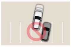
If Remote Smart Parking Assist is used, when parking next to a misaligned vehicle, your vehicle may cross the parking marking on the opposite side of the parked vehicle.
