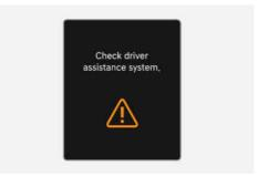
When Highway Driving Assist is not working properly, the "Check driver assistance system." warning message may appear and the \(\text{\Lambda}\) warning light may illuminate on the
