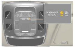
Insert the key or a similar rigid device into the passenger's front airbag ON/OFF switch and turn it to the POWER ON position. The passenger airbag ON (®) indicator will illuminate.
