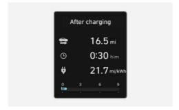
Trip distance, total driving time, average energy consumption, and instant energy consumption after the vehicle has been recharged are displayed.
