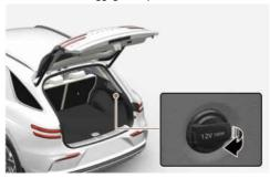
The power outlet is designed to provide power for mobile phones or other devices designed to operate with vehicle electrical systems. The devices should draw less than 180 W with the vehicle running.
