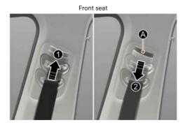
Release the button to lock the anchor in place. Try pushing the height adjuster down to make sure that it is locked in place.
