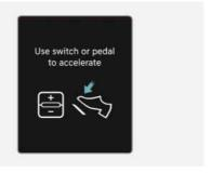
When Highway Driving Assist is operating, your vehicle stops if the vehicle ahead of you stops. Also, if the vehicle ahead of you starts moving within 30 seconds after the stop, your vehicle starts as well. If your vehicle has stopped and 30 seconds have passed, the "Use switch or pedal to accelerate" message appears on the instrument cluster. Depress the accelerator pedal or push the +, - or || $\bigcirc$  switch to accelerate.
