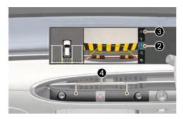
The rear view appears on the screen to assist parking. The rear view has top view, rear view, side view, and 3D view.
