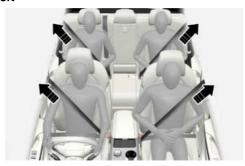
Your vehicle is equipped with driver's, front passenger's and rear passengers' (if equipped, except for the rear centre seat) pretensioner seat belts (retractor pretensioner). The pretensioner makes sure the seat belts fit tightly against your body in certain frontal or side collision(s). The pretensioner seat belts may be activated in some crashes where the frontal or side collision(s) is severe enough, together with the airbags.
