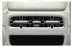
The instrument panel vent air flow can be directed up/down or left/right using the vent adjustment lever.
