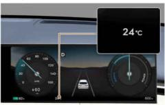
The outside ambient temperature appears in the lower portion of the cluster display. The temperature reads in Celsius or Fahrenheit depending on the units selected from the Settings menu in the infotainment system.
