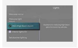
With the Start/Stop button in the DRIVE READY position, select **Setup > Vehicle > Lights > HBA (High Beam Assist)** from the Settings menu to turn on High Beam Assist and deselect to turn off the function.
