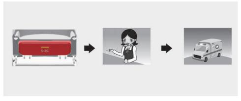
The driver or passenger manually can make an emergency call to the Public Safety Answering Point (PSAP), by pressing SOS button to call the necessary emergency services.
