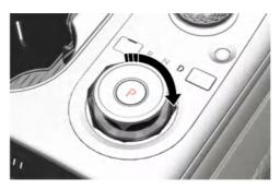
To shift the gear to D (Drive), rotate the shift dial clockwise whilst depressing the brake pedal.
