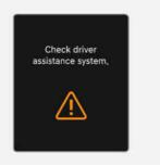
When Safe Exit Warning is not working properly, the "Check driver assistance system." warning message may appear for several seconds, and the  $\triangle$  warning light may illuminate on the instrument cluster. We recommend that your vehicle be inspected by an authorised retailer of Genesis Branded products.
