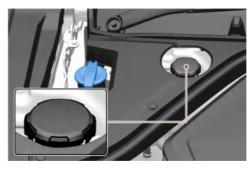
Check the fluid level in the reservoir periodically. The fluid level must be between the MAX (Maximum) and MIN (Minimum) marks on the side of the reservoir.
