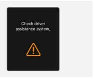
When Intelligent Speed Limit Assist is not working properly, the "Check driver assistance system." warning message may appear on the instrument cluster for several seconds, and the A and warning lights may illuminate on the instrument cluster. We recommend that your vehicle be inspected by an authorised retailer of Genesis Branded products.
