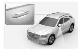
Welcome system helps keep the driver visible by turning on vehicle lights when the driver approaches the vehicle.
