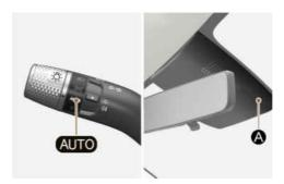
The position light and headlight are turned ON or OFF automatically depending on the amount of daylight as measured by the ambient light sensor [A] at the upper end of the windscreen glass.
