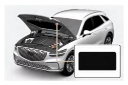
You can find out which air conditioning refrigerant is applied to your vehicle on the label located inside of the bonnet.
