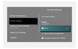
The VGS function artificially adjusts the speedometer which is based on the virtual gear ratio, and then displays the gear stage and virtual rpm on the instrument cluster to let you experience the sense of acceleration as in the internal combustion engine.
