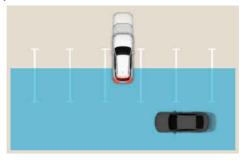
Rear Cross-Traffic Collision-Avoidance Assist may detect vehicles passing by behind you when parking in reverse into a parking space. If this occurs, the function may activate a warning and brake your vehicle even when not needed.
