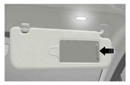
Opening the lid of the vanity mirror. The vanity mirror lamp turns on when the lid is opened and off when the lid is closed.
