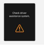
When Rear Cross-Traffic Collision-Avoidance Assist is not working properly, the "Check driver assistance system." warning message may appear for several seconds, and the ∧ warning light may illuminate on the instrument cluster. We recommend that your vehicle be inspected by an authorised retailer of Genesis Branded products.
