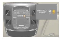
Insert the key or a similar rigid device into the passenger's front airbag ON/OFF switch and turn it to the OFF position. The passenger airbag OFF (%) indicator will illuminate and stay on until the passenger's front airbag is reactivated.
