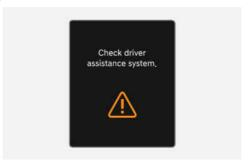
When Intelligent Front-Lighting System does not work properly, the "Check driver assistance system." warning message may appear for a few seconds on the instrument cluster. After the message disappears, the AFS and A warning lights illuminate on the instrument cluster. We recommend that the system be inspected by an authorised retailer of Genesis Branded products.
