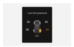
This warning message appears if the tyre pressure is low. The corresponding tyre on the vehicle illuminates.
