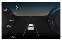
Displays the state of Smart Cruise Control, Lane Following Assist, Lane Keeping Assist, Highway Driving Assist, etc., when Driving Assist view is selected.
