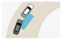
Blind-Spot Collision-Avoidance Assist may detect a vehicle in the same lane when driving on curves and activate a warning and brake your vehicle.
