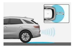
The smart tailgate detecting area extends about 20-40 in. (50-100 cm) behind the vehicle. If you are positioned in the detecting area and are carrying the smart key, the hazard warning lights blink and the chime sounds 6 times before opening.
