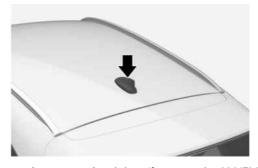
The shark fin antenna receives transmitted data (for example, AM/FM).
