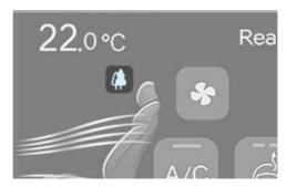
Whilst operating automatic climate control system, the indoor fine dust concentration is measured by the fine dust sensor equipped in the vehicle and the indoor air status is presented on the screen. If needed, it prevents the contaminated external air and the cabin air filter purifies the indoor air by filtering the fine dust to provide fresh air.
