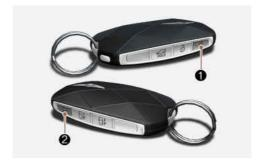
You can start the vehicle using the Remote Start button on the smart key.
