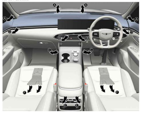
The mode selection icon controls the direction of the air flow through the ventilation system.
