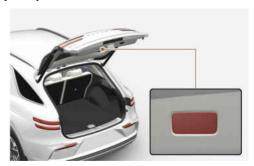
The tailgate emergency lamp turns on when the tailgate is opened.
