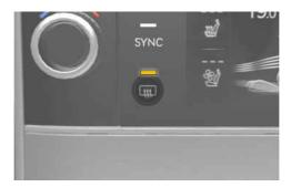
The defroster heats the window to remove frost, fog, and thin ice from the interior and exterior of the rear window, whilst the vehicle is running.
