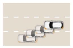
Highway Lane Change Assist function helps change lanes to the direction you operate the turn signal switch if the function judges that lane change is possible.
