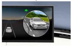
Blind-Spot View Monitor uses the wide-side view cameras to display the rear blind spot areas of your vehicle on the instrument cluster when the turn signal is turned on to help with safe lane changes.
