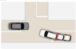
Junction Turning function helps avoid a collision with an oncoming vehicle or motorcyclist in an adjacent lane when turning right at a crossroad with the turn signal on by applying emergency braking.
