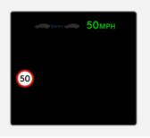
Manual Speed Limit Assist or Smart Cruise Control assists you to adjust the vehicle speed according to the speed limit. When the set speed is same as the speed limit, the set speed automatically changes to the current speed limit if the speed limit changes. The function operates on the road which has a speed limit of 45 mph (70 km/h) or higher. When the function is active, the set speed on the instrument cluster appears in green.
