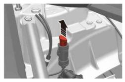
• If the charging connector does not disconnect after pulling the emergency cable, we recommend that your vehicle be inspected by an authorised retailer of Genesis Branded products.
