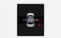
When an approaching vehicle from the rear is detected whilst a door is being opened, the warning light on the side view mirror may blink, the "Collision warning!" warning message may appear on the instrument cluster, and an audible warning may sound.
