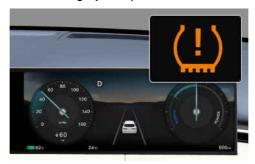
The TPMS Malfunction Indicator will illuminate after it blinks for about one minute when there is a problem with the Tyre Pressure Monitoring System.
