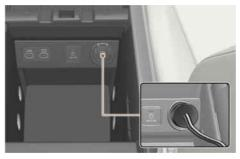
8 With the vehicle is DRIVE READY (READY indicator ON), switch on the compressor and let it run for about 5-7 minutes to fill the sealant up to proper inflation pressure. (Refer to the "Tyres and wheels" section in chapter 2). The inflation pressure of the tyre after filling is unimportant and will be checked/corrected later.
