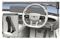
3 Go to the front of the vehicle, raise the bonnet slightly, push up the secondary bonnet release lever (1) inside of the bonnet centre and lift the bonnet (2). After the bonnet has been lifted halfway, it is raised completely by itself.
