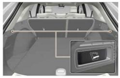
Pull the rear seat back folding lever located in the both sides of the luggage compartment.
