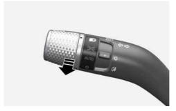
To flash the high beam headlight, pull the lever toward you, then release the lever. The high beams remain ON as long as you hold the lever.
