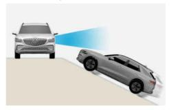
Rear Cross-Traffic Collision-Avoidance Assist may be limited when your vehicle is on a uphill or downhill slope, and may not detect any vehicle approaching from the left or right. If this occurs, the function may activate a warning and brake your vehicle even when not needed.
