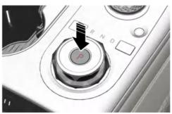
To shift the gear to P (Park), press the P button whilst depressing the brake pedal. If you turn the vehicle off in R (Reverse), N (Neutral) or D (Drive), the gear shifts to P (Park).
