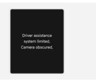
When the front view camera is covered or blocked, the Intelligent Front-Lighting System may temporarily not work properly. The "Driver assistance system limited. Camera **obscured.**" warning message may appear on the instrument cluster.
