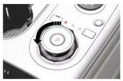
To shift the gear to R (Reverse), rotate the shift dial counterclockwise whilst depressing the brake pedal.
