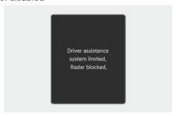
If the front radar is covered or blocked, its detecting performance is reduced, and Smart Cruise Control is temporarily limited or disabled.
