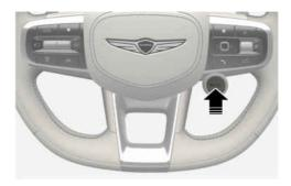
Controls motor to maximum performance when pressing BOOST button on the steering wheel remote control in situations where rapid acceleration is required.
