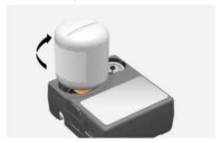
4 Make sure that the valve for reducing tyre inflation pressure is closed.
