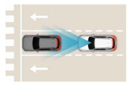
Forward Collision-Avoidance Assist helps detect a vehicle, a motorcyclist, a pedestrian, or a cyclist ahead on the road and may warn you of a possible collision with a warning message on the instrument cluster and a warning sound. Also, Forward Collision-Avoidance Assist may assist with braking your vehicle to help reduce collision speed or help avoid a collision.
