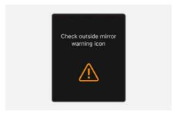
When the outside rearview mirror warning light is not working properly, the "Check outside mirror warning icon" warning message may appear for several seconds, and the  $\triangle$  warning light may illuminate on the instrument cluster. We recommend that your vehicle be inspected by an authorised retailer of Genesis Branded products.
