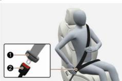
Pull the seat belt out of the retractor and insert the metal tab (1) into the buckle (2). An audible "click" sounds when the tab locks into the buckle. Make sure the seat belt is not twisted.
