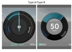
• CHARGE: It shows the charging status of the battery, which is charged by the regenerative brakes, when depressing the brake pedal or decreasing the vehicle speed due to coasting. The more electric energy is charged, the more the gauge level turns counterclockwise.
