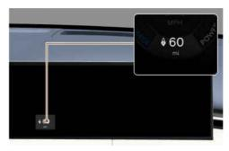
The distance to empty vary depending on many factors such as driving habits. power usage, driving conditions, and high voltage battery. The distance to empty may be increased or decreased than the certified figures as it reflects all the factors comprehensively. Check the distance to empty considering the following:
