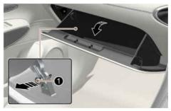
2 Remove the stoppers on both sides to allow the glove box to hang open.
