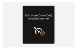
If the Driving Assist button, +, — or ∥⊃ switch is operated when Smart Cruise Control operating conditions are not satisfied, the "SCC (Smart Cruise Ctrl.) conditions not met" message appears on the instrument cluster, and an audible warning sounds.
