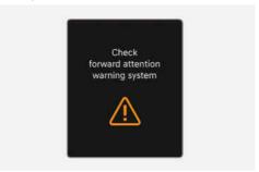
When Forward Attention Warning is not working properly, the "Check forward attention warning system" warning message appears on the instrument cluster for several seconds. the warning light illuminates on the instrument cluster, and an audible warning sounds. We recommend that your vehicle be inspected by an authorised retailer of Genesis Branded products.
