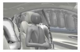
Side airbags are located in each front and outboard second row seats. Additionally, a front centre side airbag is located in the inboard side of the driver seatback.
