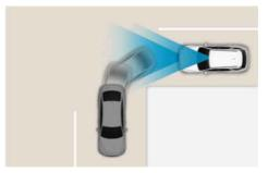
• When a vehicle in front of you merges out of the lane, Smart Cruise Control may not immediately detect a new vehicle that is now in front of your vehicle.
