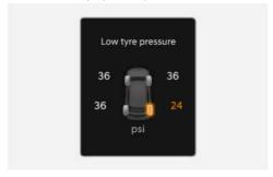
When the tyre pressure monitoring system warning indicators are illuminated and a warning message displayed on the cluster display, one or more of your tyres is significantly under-inflated. The Low Tyre Pressure Position Telltale will indicate which tyre is significantly underinflated by illuminating the corresponding position light.
