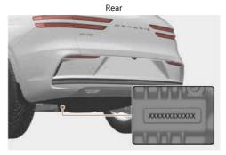
The motor number are stamped as shown in the drawing.
