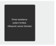
If the ultrasonic sensor is blocked or covered by any foreign material, such as snow, rain, or dirt, the detecting performance may reduce and temporarily limit or disable Parking Distance Warning.
