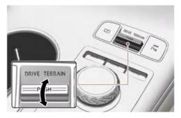
The mode changes, as the following, whenever the driver pushes the **DRIVE/TERRAIN** switch up or down.
