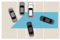
Rear Cross-Traffic Collision-Avoidance Assist may detect vehicles that are parking or pulling out near your vehicle (for example, leaving beside your vehicle, parking or pulling out behind your vehicle, approaching your vehicle making a turn). If this occurs, the function may activate a warning and brake your vehicle even when not needed.
