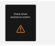
When High Beam Assist is not working properly, the "Check Driver Assistance system." warning message may appear and \( \) warning light may illuminate on the instrument cluster. We recommend that the system be inspected by an authorised retailer of Genesis Branded products.
