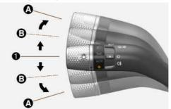
Highway Lane Change Assist function operates, when you push the turn signal lever up or down to the [A] or [B] position whilst the function is in the ready state (indicator is green), and all of the following conditions are met:
