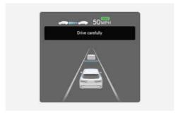
The "Drive carefully" warning message appears if Navigation-based Smart Cruise Control is not able to slow down your vehicle.
