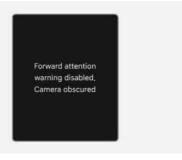
If there is an object right in front of the in-cabin camera or between you and the camera for a certain period of time Forward Attention Warning does not operate properly.
