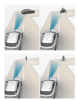
Forward Collision-Avoidance Assist may not detect other vehicles, motorcyclists, pedestrians, or cyclists in front of you when driving on a curve adversely affecting the performance of the sensors. A warning, brake assist, or steering assist (if equipped) may not be activated when needed.
