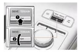
Multi terrain mode may be selected according to the driver's preference or road condition. Press the **DRIVE/TERRAIN** switch (1) to change from Drive mode to Multi terrain mode.
