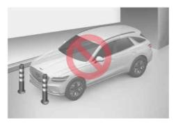
Remote Smart Parking Assist performance may be reduced or collided with an obstacle may occur when there is a narrow object, circular pillar, square pillar, or a pillar surrounded by objects such as a fire extinguisher, etc., near the parking space. Park or exit your vehicle manually.
