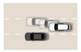
When vehicle speed is above 40 mph (60 km/h), if a detected vehicle around you is driving at a close distance, your vehicle controls the steering in the opposite direction of the vehicle. If a vehicle is detected at both sides of the lane and are driving close to you, the function does not veer to the opposite side of the lane.
