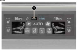
· Touch each air flow direction on the information screen to select the desired flow direction.
