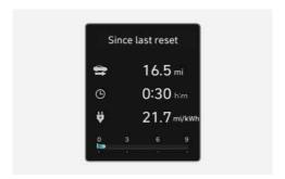
Accumulated trip distance, total driving time, average energy consumption, and instant energy consumption are displayed.
