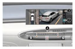
The 3D view shows the image around the vehicle from various angles.
