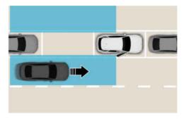
Safe Exit Warning helps detect a vehicle approaching the rear corner of your vehicle, after the vehicle is stopped and a passenger opens a door.
