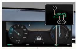
The instrument cluster displays "AUTO" (1) when the smart recuperative system is ON. Depending on the conditions, the system adjusts the regenerative braking level (2). The indicator light (3) illuminates when the vehicle recognises a vehicle.
