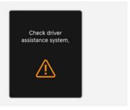
When Blind-Spot Collision-Avoidance Assist is not working properly, the "Check driver assistance system." warning message may appear for several seconds, and the Awarning light may illuminate on the instrument cluster. We recommend that your vehicle be inspected by an authorised retailer of Genesis Branded products.
