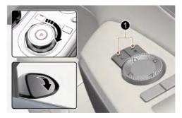
When the gear is shifted to the R (Reverse) position, the outside rearview mirror(s) rotates downward to aid with driving in reverse.
