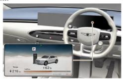
Check the charging state on the instrument cluster to monitor the battery capacity of the high voltage and estimated charging time.
