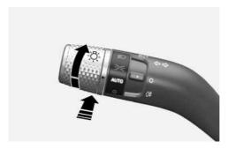
High Beam Assist automatically adjust the headlights between high beam and low beam depending on the light detected from oncoming vehicles or vehicles in front using the front view camera.
