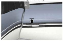
The SRS consists of airbags located in the centre of the steering wheel, in the driver's side lower crash pad below the steering wheel, and the passenger's side front panel pad above the glove box.
