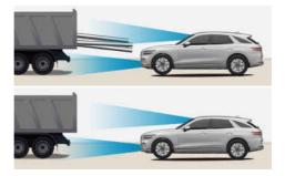
Forward Collision-Avoidance Assist may not be able to detect all potential hazards, like if the vehicle in front of you has cargo that extends rearward past the end of the vehicle or if the vehicle in front of you has higher ground clearance. Always maintain a safe distance from the vehicles ahead. Adjust your vehicle speed or steer your vehicle depending on the road conditions.
