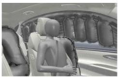
Side and curtain airbags and the front centre side airbag are designed to inflate when an impact is detected by side collision sensors depending on the severity of impact resulting from a side impact collision.
