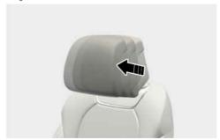
The head restraint may be adjusted forward to 3 different positions by pulling the head restraint forward to the desired detent. To adjust the head restraint to it's furthest rearwards position, pull it fully forward to the farthest position and release it.
