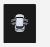
This warning appears if any door, bonnet or tailgate is left open. The warning will indicate which door is open on the cluster display.
