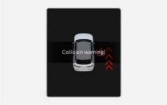
When an approaching vehicle from the rear is detected whilst a door is being opened, the warning light on the corresponding outside rearview mirror may blink, the "Collision warning!" warning message may appear on the instrument cluster, and an audible warning may sound.
