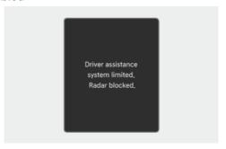
If the rear corner radar is blocked or covered, or when the rear bumper around the rear corner radar or sensor is covered by any foreign material, such as snow, rain, or dirt, or when a trailer or towbar mounted carrier is installed, the detecting performance may decrease and temporarily limit or disable Safe Exit Assist.
