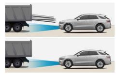
• When the vehicle in front of the foregoing vehicle is at a stop and the foregoing vehicle changes the lane, the front sensors may be unable to recognise the stopped vehicle.
