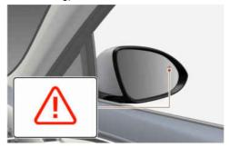
When a vehicle is detected in a blind spot, the warning light on the outside rearview mirror and head-up display (if equipped) may illuminate.
