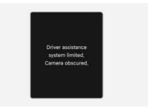
If the front view camera is covered or blocked, its detecting performance is reduced, and Intelligent Speed Limit Assist is temporarily limited or disabled.
