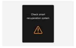
If the smart recuperative system is turned off due to the front radar being covered with foreign substances or due to other causes, the "Check smart recuperation system" warning message appears. Also the regenerative braking level is displayed instead of "AUTO".
