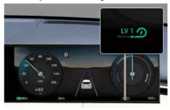
The selected recuperative braking level is displayed on the instrument cluster. When the vehicle is turned off and on again after the recuperative braking level is lowered to 0, the braking level changes to 1.
