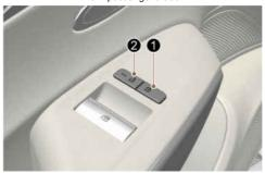
When pressing the ∄ portion (1) on the button, all vehicle doors are locked.
