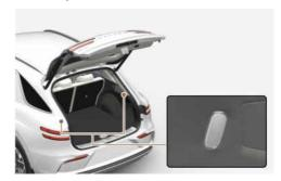
The luggage compartment lamp turns on when the tailgate is opened and off when the tailgate is closed.
