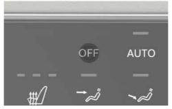
Press the **OFF** icon to turn off the climate control system. You can still operate the mode icons and air intake icons as long as the Start/Stop button is in the DRIVE READY position.
