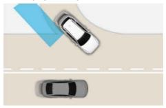
Blind-Spot Collision-Avoidance Assist may not detect a vehicle in an adjacent lane when the road merges or divides, and may not activate a warning or brake your vehicle. Always check road conditions, and if necessary, take appropriate actions to drive safely.
