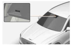
The rain sensor located on the upper end of the windscreen glass senses the amount of rainfall and controls the interval of the wiping cycle.
