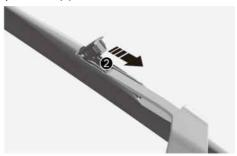
5 Remove the wiper blade from the wiper arm.
