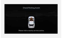
When Remote Smart Parking Assist is not working properly, the "Check Parking Assist" warning message may appear on the infotainment system screen. If the message appears, stop using Remote Smart Parking Assist, and we recommend that your vehicle be inspected by an authorised retailer of Genesis Branded products.
