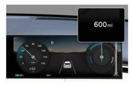
The odometer indicates the total distance that the vehicle has been driven and is used to determine when periodic maintenance should be performed.
