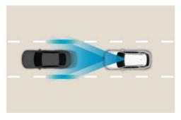
Highway Driving Assist helps maintain distance from the vehicle ahead, maintain the set speed, and centre the vehicle in the lane whilst driving on the highway (or motorway).
