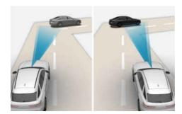
On curves, Smart Cruise Control may not detect a vehicle in the same lane, and may accelerate to the set speed. Your vehicle speed may be reduced if a vehicle is detected in an adjacent lane and your vehicle speed may rapidly decrease when a vehicle ahead is detected suddenly.
