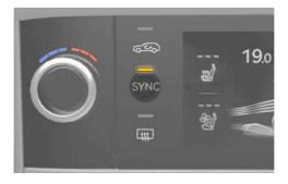
Adjusting the temperature, air flow direction, and fan speed equally Press the **SYNC** icon from the front seat, (indicator light ON), to adjust the driver, front passenger, and rear passenger side temperature, air flow direction, and fan speed equally.
