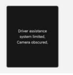
If the front view camera is covered or blocked, its detecting performance is reduced, and Driver Attention Warning may be temporarily limited or disabled.
