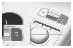
Press the Parking Safety ( $P^{n}$ ) button to turn on Parking Distance Warning. Press the button again to turn off the function.
