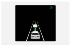
If the both lane markings and/or vehicle ahead are detected and your vehicle speed is below 110 mph (180 km/h), the green  $\odot$  indicator light illuminates on the instrument cluster, and Lane Following Assist helps centre the vehicle in the lane by assisting the steering wheel.
