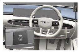
Electronic Stability Control helps stabilize the vehicle during cornering manoeuvres.
