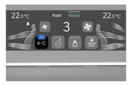
Press the A/C icon to manually turn the air conditioning on (indicator light ON) and off.
