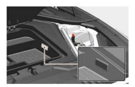
The front boot lamp turns on when the front boot cover is opened and off when the cover is closed.
