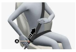
The belt should automatically draw back into the retractor. If this does not happen, check the belt to be sure it is not twisted, then try again.
