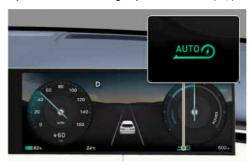
The smart recuperative system is ON and the regenerative braking level is displayed as "AUTO".
