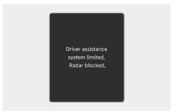
If the rear corner radar is blocked or covered, or when the rear bumper around the rear corner radar or sensor is covered by any foreign material, such as snow, rain, or dirt, or when a trailer or towbar mounted carrier is installed, the detecting performance may reduce and temporarily limit or disable Rear Cross-Traffic Collision-Avoidance Assist.
