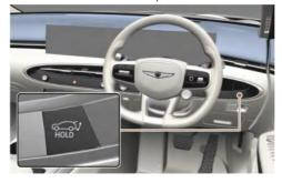
Press the power tailgate open/close button for 1 second. The tailgate opens or closes with a warning sound.
