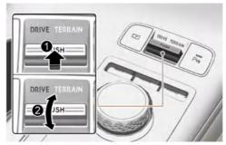
Press the **DRIVE/TERRAIN** switch (1) to change from normal driving mode to multi terrain mode. After the switch is pressed, push the switch up or down (2) within 4 seconds to select **SNOW**, **MUD**, or **SAND**.
