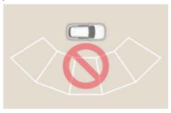
Remote Smart Parking Assist does not work normally when the parking lines are not parallel. Do not park even though the parking space is recognised by the sensor.
