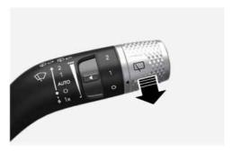
In the O position, pull the lever gently toward you to spray washer fluid on the windscreen and to run the wipers 1-3 cycles. The spray and wiper operation continues until you release the lever. If the washer does not work, you may need to add washer fluid to the washer fluid reservoir.
