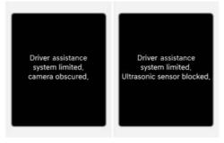
The "Driver assistance system limited. Camera obscured." or "Driver assistance system limited. Ultrasonic sensor blocked." warning message may appear on the instrument cluster if:
