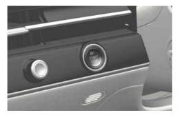
Whenever the front door is opened, the Start/Stop button illuminates and goes off 30 seconds after the door is closed.
