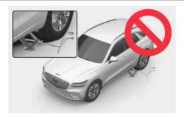
Never start or run the vehicle whilst an AWD vehicle is raised on a jack. The vehicle may slip or roll off of a jack causing serious injury or death.
