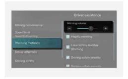
With the vehicle on, select **Setup** > **Vehicle** > **Driver assistance** > **Warning methods** from the Settings menu in the infotainment system to select the following:
