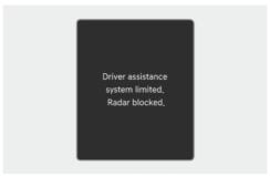
If the rear corner radar is blocked or covered, or when the rear bumper around the rear corner radar or sensor is covered by any foreign material, such as snow, rain, or dirt, or when a trailer or towbar mounted carrier is installed, the detecting performance may reduce and temporarily limit or disable Blind-Spot Collision-Avoidance Assist.
