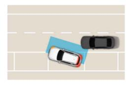
Blind-Spot Collision-Avoidance Assist may brake your vehicle if there is a detected collision risk in the blind spot area when driving forward out of a parking space.
