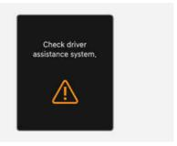
When Lane Following Assist is not working properly, the "Check driver assistance system." warning message may appear for several seconds, and the /\ warning light may illuminate on the instrument cluster. We recommend that your vehicle be inspected by an authorised retailer of Genesis Branded products.
