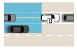
Safe Exist Assist helps detect a vehicle approach the rear corner of your vehicle, after the vehicle is stopped and a passenger opens a door.
