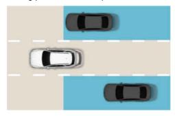
Blind-Spot Collision-Avoidance Assist helps detect and warns you that a vehicle is in the blind spot area.
