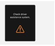
When Smart Cruise Control is not working properly, the "Check driver assistance system." warning message may appear and the \( \underset \) warning light may illuminate on the instrument cluster. We recommend that your vehicle be inspected by an authorised retailer of Genesis Branded products.
