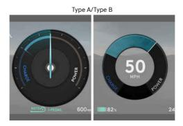
The Charge/Power Gauge shows the energy consumption and recovery status of the electric motor.
