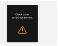
When Safe Exit Assist is not working properly, the "Check driver assistance system." warning message may appear for several seconds, and the <u>A</u> warning light may illuminate on the instrument cluster. We recommend that your vehicle be inspected by an authorised retailer of Genesis Branded products.
