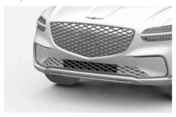
The active air flap system controls the air flap below the front bumper to cool vehicle parts and improve fuel efficiency.
