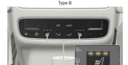
Whilst the vehicle is running, press the button or icon to warm the rear seats.
