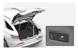
You can connect home appliances or electric devices to the power outlet inside the vehicle and use them conveniently.
