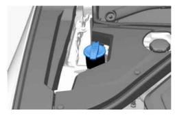
Check the fluid level in the washer fluid reservoir and add fluid if necessary. Plain water can be used if washer fluid is not available. However, use washer fluid with antifreeze in cold climates to prevent freezing.
