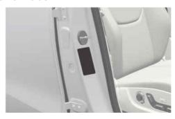
The vehicle certification label attached on the driver's (or front passenger's) side centre pillar gives the vehicle identification number (VIN).
