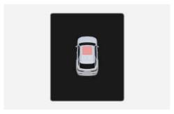
If the driver turns off the engine when the sunroof is not fully closed, the warning chime sounds for several seconds and the sunroof open warning appears on the cluster display. Close the sunroof securely when leaving your vehicle.
