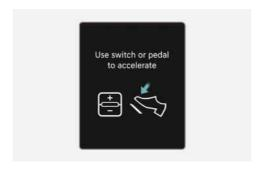
In traffic, your vehicle stops if the vehicle ahead of you stops. Also, if the vehicle ahead of you starts moving, your vehicle starts moving as well. In addition, after your vehicle has stopped and a certain time have passed, the "Use switch or pedal to accelerate" message appears on the instrument cluster. Depress the accelerator pedal or push the +, - or | switch to start driving.
