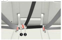
Insert the tongue plate (2) into the buckle (1) until an audible "click" is heard, indicating the latch is locked. Pull the shoulder portion of the belt to snug the belt across your hips and remove slack. Make sure the seat belt is not twisted.
