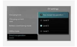
To adjust the recuperative braking level of the smart recuperation system, go to Home screen and select Electric vehicle > **Φ**(EV settings) > Smart recuperation from the infotainment system.
