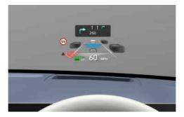
The head-up display is an optional feature that allows the driver to view information projected onto a transparent screen whilst still keeping your eyes safely on the road ahead whilst driving.
