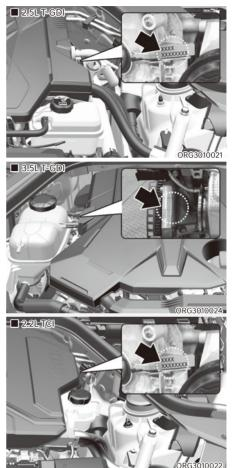
The engine number is stamped on the engine block as shown in the drawing.
