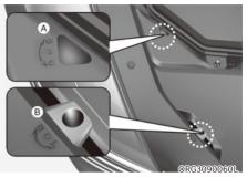
[A] : Low beam and high beam vertical aiming
