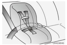
Installing a Child Restraint System with a lap/shoulder belt
