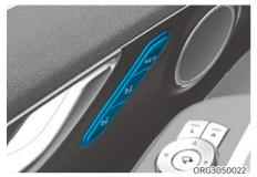
Integrated Memory System for the driver's seat is provided to store and recall the following memory settings with a simple button operation.
