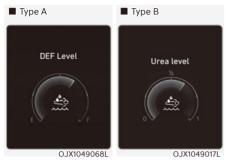
DEF level / Urea level (for diesel engine, if equipped)
