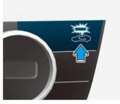
The air intake control button is used to select either Fresh mode (outside air) or Recirculation mode (cabin air).
