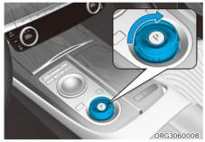
To shift the gear to D (Drive), rotate the shift dial clockwise while depressing the brake pedal.
