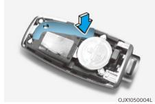
2. Press the mechanical key and remove it from the smart key FOB.
