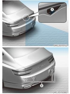
[A]: Rear view camera, [B]: Rear ultrasonic sensors
