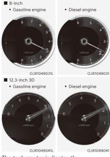
The tachometer indicates the approximate number of engine revolutions per minute (rpm).
