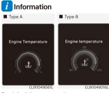
For 8-inch instrument cluster, you can check the engine coolant temperature in the Utility view on the cluster.
