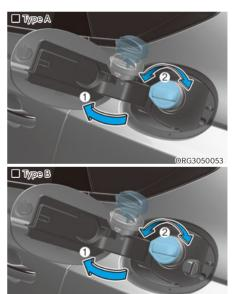
4. Pull the fuel filler door (1) outward to access the fuel tank cap.
