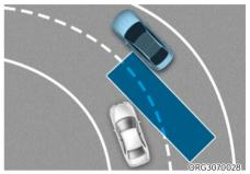
Blind-Spot Safety system may not operate properly when driving on a curved road. The system may not detect the vehicle in the next lane.
