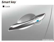
Touch the touch sensor on the front outside door handle (the engraved part) while carrying the Smart Key with you or press the Door Lock button on the Smart Key, all doors will lock.
