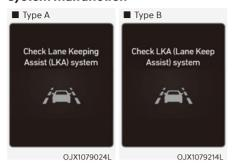
When Lane Keeping Assist is not working properly, the 'Check Lane Keeping Assist (LKA) system' (or 'Check LKA (Lane Keeping Assist) system') warning message will appear and the yellow indicator light will illuminate on the cluster. If this occurs, we recommend that the system be inspected by an authorized retailer of Genesis Branded products.
