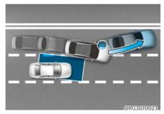
When changing lanes by detecting the lane ahead, if the system judges that there is a collision risk with an approaching vehicle in the blind spot, the system will help avoid collision by applying the brake.
