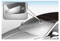
Auto defogging helps reduce the possibility of fogging up the inside of the windshield by automatically sensing the moisture on inside the windshield.
