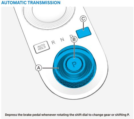
[A] : Rotary shifter (Rotary gear shift dial), [B] : P button, [C] : P release cap
