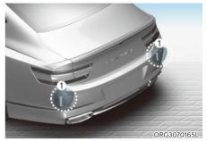
[1] : Rear corner radar Refer to the picture above for the detailed location of the detecting sensor.
