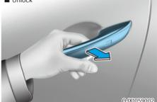
Put your hand in the front outside door handle while carrying the Smart Key with you or press the Door Unlock button on the Smart Key, all doors will unlock.
