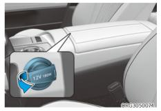
The power outlet is designed to provide power for mobile telephones or other devices designed to operate with vehicle electrical systems. The devices should draw less than 180 W with the engine running.
