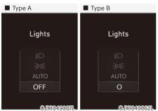
This indicator displays which exterior light is selected using the lighting control.
