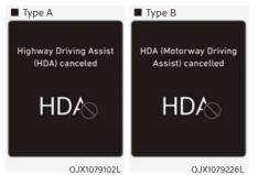
If the driver still does not have their hands on the steering wheel after the hands-off warning, the 'Highway Driving Assist (HDA) canceled' (or 'HDA (Highway Driving Assist) cancelled') warning message will appear and Highway Driving Assist and Lane Change Assist will be automatically canceled.
