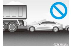
Do not use Remote Smart Parking Assist around vehicles with higher ground clearance, such as a bus, truck, etc. It may lead to an accident. • Parking near a pillar
