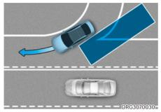
Blind-Spot Safety system may not operate properly when driving where the road merges or divides. The system may not detect the vehicle in the next lane.
