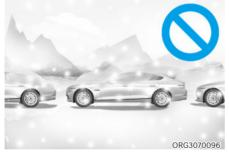
Snow may interfere with sensor operation, or Remote Smart Parking Assist may cancel if the road is slippery while parking. • Parking on uneven road
