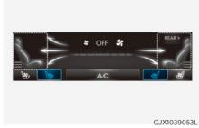
• While the engine is running, touch either of the seat warmer icons to warm the driver's seat or front passenger's seat.
