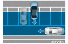
Rear Cross-Traffic Safety system may detect vehicles passing by behind you when parking backwards into a parking space. If this occurs, the system may unnecessarily warn the driver.
