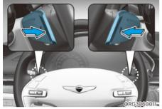
The paddle shifter allows the driver to shift gear without taking one's hands off the steering wheel.
