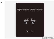
The OK button is pressed on the steering wheel when a message on the cluster inquires whether or not Highway Lane Change Assist function will be used.
