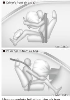
After complete inflation, the air bag immediately starts deflating, enabling the driver to maintain forward visibility and the ability to steer or operate other controls.
