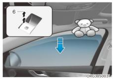
If a window senses any obstacle while it is closing automatically, it will stop and lower approximately 30 cm (12 in.) to allow the object to be cleared.
