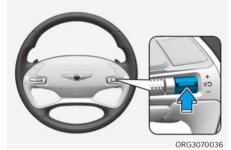
Push the **IIO** switch to temporarily pause the set speed limit. The set speed limit will turn off but the Speed Limit (**O**I IMIT) indicator will stay on.
