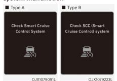
When Smart Cruise Control is not working properly, the 'Check Smart Cruise Control system' (or 'Check SCC (Smart Cruise Control) system') warning message will appear, and the A warning light will illuminate on the cluster. We recommend that the system be inspected by an authorized retailer of Genesis Branded products.
