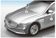
[1], [2]: Surround-side view camera (camera located at bottom of the mirror)
