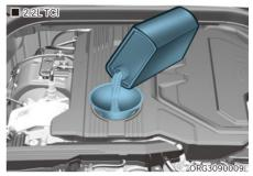
If the level is in the D range, add enough engine oil to bring the level up to the C range.
