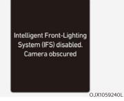
When the front view camera is covered with dirt, snow, or debris, Intelligent Front-Lighting System may temporarily not work properly. If this occurs, a warning message will appear on the cluster.
