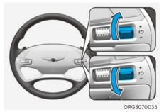
To resume Manual Speed Limit Assist after the system was paused, push the +, -, **IID** switch.
