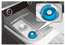
To shift the gear to R (Rear), rotate the shift dial counterclockwise while depressing the brake pedal.
