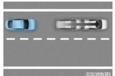
If the vehicle in front abruptly departures, Leading Vehicle Departure Alert may not operate properly. • When a pedestrian or bicycle is between you and the vehicle ahead
