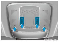
Front map lamp (  $\checkmark$   $\checkmark$ ): Touch either icons to turn the map lamp on or off. This light produces a spot beam for convenient use as a map lamp at night or as a personal lamp for the driver and the front passenger.
