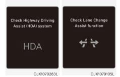
When Highway Driving Assist or Highway Lane Change function is not working properly, the 'Check Highway Driving Assist (HDA) system' or 'Check Lane Change Assist function' warning message will appear, and the A warning light will illuminate on the cluster. We recommend that the system be inspected by an authorized retailer of Genesis Branded products
