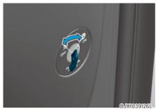
Passenger's front air bag ON/OFF switch (if equipped)
