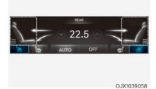
You can also adjust the rear air ventilation seat from the front seats. With the engine running, touch the air ventilation seat icon on the climate control system screen.
