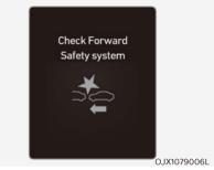
When Forward Collision-Avoidance Assist is not working properly, the 'Check Forward Safety' warning message will appear, and the 🛬 and <u>A</u> warning lights will illuminate on the cluster. We recommend that the system be inspected by an authorized retailer of Genesis Branded products.
