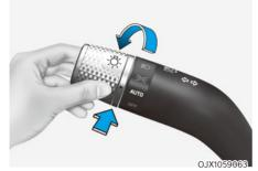
High Beam Assist is a system that automatically adjusts the headlamp range (switches between high beam and low beam) depending on the brightness of detected vehicles and certain road conditions.
