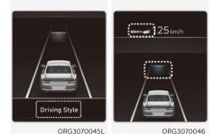
When Based on Driving Style is operating, 'Driving Style' message will appear on the cluster for 2 seconds, and the distance level and target distance will be displayed based on the driving style.
