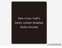
When the rear bumper around the rearside radar or sensor is covered with foreign material, such as snow or rain, or installing a trailer or carrier, it can reduce the detecting performance and temporarily limit or disable Rear Cross-Traffic Safety system.
