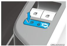
The driver can disable the power window switches on the rear passenger doors by pressing the power window lock button.
