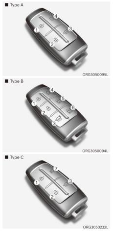
Your Genesis Branded Vehicle uses a Smart Key, which you can use to lock or unlock the driver and passenger doors or the rear trunk.
