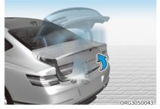
If, during power opening or closing, the trunk is blocked by an object or part of someone's body, the power trunk will detect the resistance and it will stop movement or move to the full open position to allow the object to be cleared.
