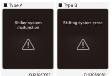
This message is displayed when the transmission or the shift button does not
