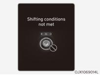
This message is displayed when engine rpm is too high, or when driving speed is too fast to shift the gear.
