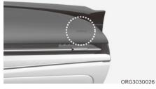
Your vehicle is equipped with a Supplemental Restraint System (SRS) and lap/shoulder belts at both the driver and passenger seating positions. The SRS consists of air bags which are located in the center of the steering wheel, in the driver's side lower crash pad below the steering wheel, and the passenger's side front panel pad above the glove box.
