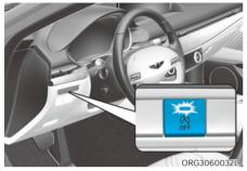
When the system is deactivated, the ISG off button indicator will illuminate and a message 'Auto Stop error. Shift to P or N to start engine manually' appears on the cluster LCD display with a warning sound.
