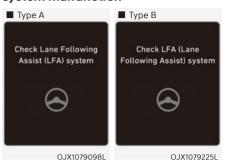
When Lane Following Assist is not working properly, the 'Check Lane Following Assist (LFA) system' (or 'Check LFA (Lane Following Assist) system') warning message will appear on the cluster. If this occurs, we recommend that the system be inspected by an authorized retailer of Genesis Branded products.
