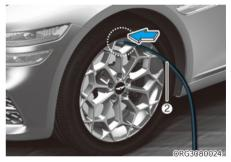
3. Unscrew the valve cap from the valve of the flat tire and screw the filling hose (2) of the sealant bottle onto the valve.
