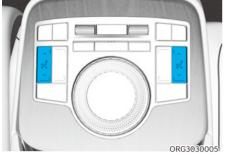
Press the control switch to slide the seat to the desired position. The seatback angle is adjusted automatically along with the seat sliding position.
