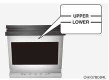
If your vehicle is equipped with a battery marked with LOWER (MIN) and UPPER (MAX) on the side, you should check the electrolyte level.
