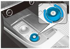
To shift the gear to N (Neutral), rotate the shift dial clockwise from R (Reverse) or counterclockwise from D (Drive) while depressing the brake pedal.
