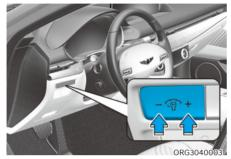
When the vehicle's position lights or headlamps are on, press the illumination control switch to adjust the brightness of the instrument panel illumination.
