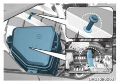
5. Remove the engine compartment fuse box cover.
