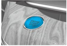
Whenever the front door is opened, the Engine Start/Stop button will illuminate and will go off 30 seconds after the door is closed.
