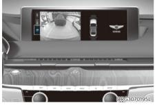
You can change Rear View Monitor settings by pressing the setup icon (♠) on the screen while the system is operating, or select 'Driver Assistance → Parking Safety → Camera Settings' from the Settings menu while the Engine Start/Stop button is in the ON position.
