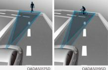
**Forward Collision-Avoidance Assist** may detect a vehicle, pedestrian or cyclist in the next lane or outside the lane when driving on a curved road.
