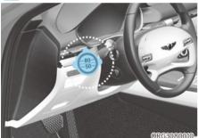
Detach the speed restriction label (1) from the sealant bottle (2), and place it in a highly visible place inside the vehicle such as on the steering wheel to remind the driver not to drive too fast. 1. Shake the sealant bottle (2).
