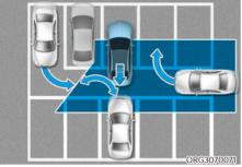
Rear Cross-Traffic Safety system may detect vehicles which are parking or pulling out near your vehicle (for example: a vehicle leaving beside your vehicle, a vehicle parking or pulling out in the rear area, a vehicle approaching your vehicle making a turn, etc.). If this occurs, the system may unnecessarily warn the driver.
