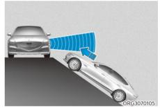
Rear Cross-Traffic Safety system may be limited when the vehicle is on a uphill or downhill slope, or near it, and may not detect the vehicle approaching from the left or right. If this occurs, the system may not warn the driver when necessary.
