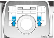
• While the engine is running, press either of the air ventilation switches to cool the seat. • Each time you press the switch, the air flow changes as follows:
