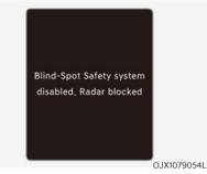
When the rear bumper around the rear corner radar or sensor is covered with foreign material, such as snow or rain, or installing a trailer or carrier, it can reduce the detecting performance and temporarily limit or disable Blind-Spot Safety system.
