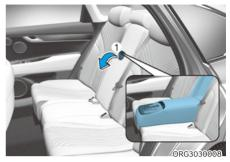
The armrest is located in the center of the rear seat.
