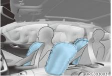
Your vehicle is equipped with a side air bag in each front and outboard second row seat. Additionally, a front center air bag is provided in the inboard side of the driver seatback. The purpose of the air bag is to provide the vehicle's additional protection than that offered by the seat belt alone. The side air bags and front center air bag are designed to deploy during certain side impact collisions, depending on the crash severity.
