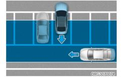
Rear Cross-Traffic Safety system may detect vehicles passing by behind you when parking backwards into a parking space. If this occurs, the system may unnecessarily warn the driver and control the brake.
