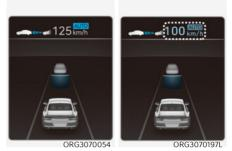
If temporary deceleration is required in the standby state and Navigation-based Smart Cruise Control is operating, the green AUTO symbol will illuminate on the cluster.
