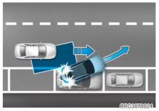
When you are driving forward out of a parking space, if the system judges that there is a collision risk with an approaching vehicle in the blind spot, the system will help avoid collision by applying the brake.
