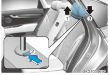
Adjusting the height up and down To raise the headrest:
