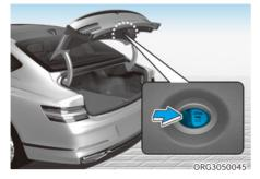
Your vehicle is equipped with an Emergency Trunk Safety Release lever located inside the trunk. When someone is inadvertently locked in the trunk, the trunk can be opened by moving the lever in the direction of the arrow and pushing the trunk open.
