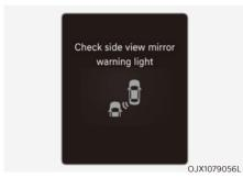
When the outside rearview mirror warning light is not working properly, the 'Check side view mirror warning light' warning message will appear on the cluster. We recommend that the system be inspected by an authorized retailer of Genesis Branded products.
