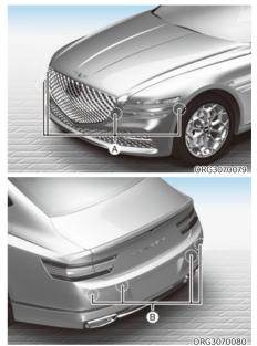
[A] : Front ultrasonic sensors,[B] : Rear ultrasonic sensors
