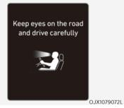
Forward Attention Warning determines whether the driver is focused on the road depending on information, such as the amount of time the driver is looking elsewhere, the amount of time the eyes are closed, how frequently the driver yawns, etc. If the system judges the driver is not focused, the 'Keep eyes on the road and drive careful' warning message will appear on the cluster, and an audible warning will sound.
