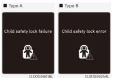
When electronic child safety lock does not work even though the button is pressed, the message will be displayed and an alarm will sound. If this occurs, we recommend that the vehicle be inspected by an authorized retailer Genesis Branded products.
