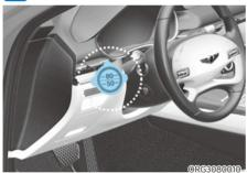
Detach the speed restriction label (0) from the sealant bottle (1), and place it in a highly visible place inside the vehicle such as on the steering wheel to remind the driver not to drive too fast. 1. Shake the sealant bottle (1).
