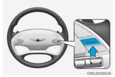
Press the Driving Assist MODE button to turn Cruise Control off. The Cruise (MCRUISE) indicator will go off.
