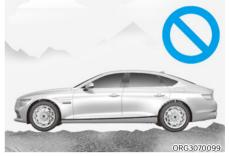
Remote Smart Parking Assist may cancel when the vehicle slips, or the vehicle cannot move due to road conditions such as pebbles or fragmented stones.
