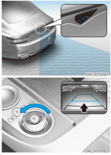
Rear View Monitor will show the area behind the vehicle to assist you when parking or backing up.
