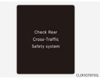
When Rear Cross-Traffic Safety system is not working properly, the 'Check Rear Cross-Traffic Safety system' warning message will appear on the cluster, and the system will turn off automatically or the system will be limited. We recommend that the system be inspected by an authorized retailer of Genesis Branded products.
