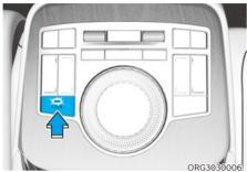
You can activate or deactivate the rear seat control by using the LOCK button on the rear armrest.
