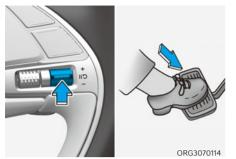
To temporarily cancel the system Press the II'D switch or depress the brake pedal to temporarily cancel Smart Cruise Control.
