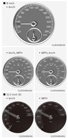
The speedometer indicates the speed of the vehicle and is calibrated in kilometers per hour (km/h) and/or miles per hour (MPH).
