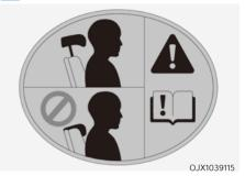
When sitting on the rear seat, do not adjust the height of the headrest to the lowest position.
