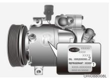
A compressor label informs you the type of compressor your vehicle is equipped with such as model, supplier part number, production number, refrigerant (1) and refrigerant oil (2).
