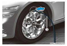
4. Unscrew the valve cap from the valve of the defective wheel and screw the filling hose (3) of the sealant bottle onto the valve.
