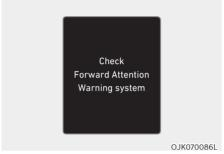
When Forward Attention Warning is not working properly, the 'Check Forward Attention Warning system' warning message will appear on the cluster for several seconds, and the master \( \tilde{\triangle} \) warning light will illuminate on the cluster. If this occurs, we recommend that the vehicle be inspected by an authorized retailer of Genesis Branded products.
