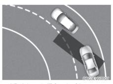
Blind-Spot Collision-Avoidance Assist may not operate properly when driving on a curved road. The function may recognize a vehicle in the same lane.
