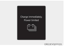
When the high voltage battery level reaches below approximately 6%, this warning message is displayed.
