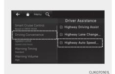
With the vehicle on, select 'Driver Assistance → Driving Assist → Highway Auto Speed Change' from the Settings menu to turn on Navigation-based Smart Cruise Control and deselect to turn off
