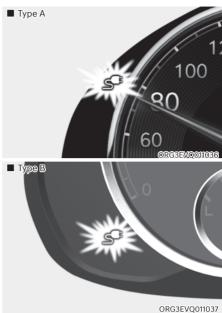
10. Check if the charging indicator light (\$\sigma\$) of the high voltage battery in the instrument cluster is turned ON. Charging is not active when the charging indicator light (\$\sigma\$) is OFF. When the charging connector is not connected properly, reconnect the charging cable to charge it again.
