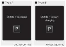
This message is displayed if you connect the charging cable without the gear in the P (Park) position.
