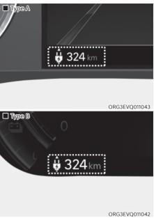
The distance to empty is displayed differently according to the selected drive mode in the Drive Mode Integrated Control System.
