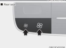
The fan speed can be set to the desired speed touching the st or ficon, or by turning the fan speed control knob. More air is delivered with higher fan speeds.
