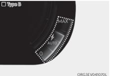
With 'AUTO' for the regenerative braking level displayed on the instrument cluster, the regenerative braking level is controlled automatically when vehicle speed is above 10 km/h and one of the condition below is met.
