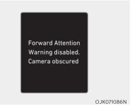
When there is an object right in front of the camera or between the driver and the camera for a certain period of time, Forward Attention Warning will not operate properly, and the 'Forward Attention Warning disabled. Camera obscured' warning message will appear on the cluster.
