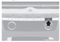
1. Press the SETUP button on the head unit of the infotainment system.
