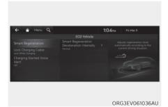
The responsiveness of the smart regenerative braking be adjusted based on the setting of the driver's deceleration style (strong/medium/gentle).
