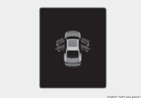
This warning is displayed if any door or hood or trunk is left open. The warning will indicate which door is open in the display.
