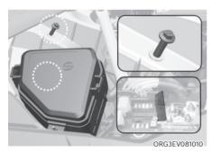
5. Remove the motor compartment fuse box cover.
