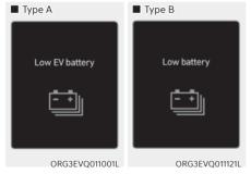
When the high voltage battery level reaches below approximately 12%, this warning message is displayed.
