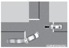
Junction Turning function can help avoid a collision with an oncoming vehicle in an adjacent lane when turning left (lefthand drive) or right (right-hand drive) at a crossroad with the turn signal on by applying emergency braking.
