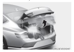
If, during power opening or closing, the trunk is blocked by an object or part of someone's body, the power trunk will detect the resistance and it will stop movement or move to the full open position to allow the object to be cleared.
