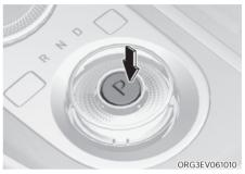
To shift the gear to P (Park), press the P button while depressing the brake pedal. If you turn the vehicle off in R (Reverse), N (Neutral) or D (Drive), the gear will automatically shift to P (Park).
