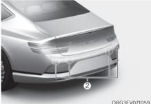
[1]: Rear view camera,[2]: Rear ultrasonic sensors
