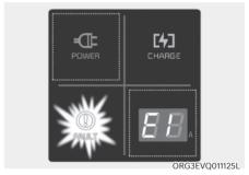
Before plugging charging connector into vehicle (POWER Green ON, FAULT Red blink)
