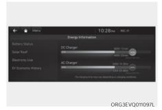
You can check the reachable range, total battery power remaining, and expected charging time for each charge type.
