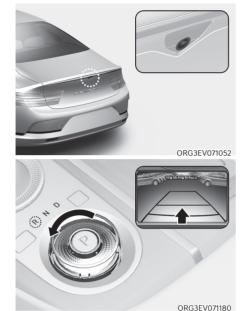
Rear View Monitor shows the area behind the vehicle to assist you when parking or backing up.
