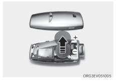
Remove battery cover using a phillips screwdriver.
