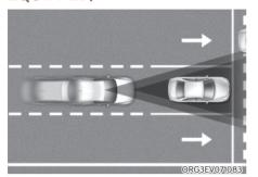
Forward Collision-Avoidance Assist is designed to help detect and monitor the vehicle ahead or help detect a pedestrian or cyclist in the roadway and warn the driver that a collision is imminent with a warning message and warning and apply emergency braking.
