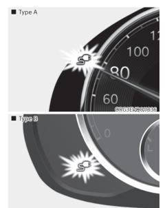
Check if the charging indicator light (\$\( \sigma \) of the high voltage battery in the instrument cluster is turned ON. Charging is not active when the charging indicator light (\$\( \sigma \) is OFF.
