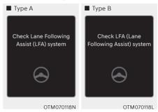
When Lane Following Assist is not working properly, the 'Check Lane Following Assist (LFA) system' (or 'Check LFA (Lane Following Assist) system') warning message will appear for several seconds, and the master (A) warning light will illuminate on the cluster. If this occurs, we recommend that the vehicle be inspected by an authorized retailer of Genesis Branded products.
