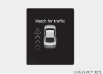
Collision warning when exiting vehicle
