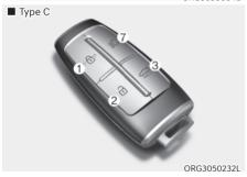
Your Genesis Branded Vehicle uses a Smart Key, which you can use to lock or unlock the driver and passenger doors or the rear trunk.
