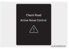
When Active noise control-road is not working properly, this warning message will appear on the cluster LCD display. If this occurs, we recommend that the system be inspected by an authorized retailer of Genesis Branded products.
