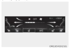
While the vehicle is running, touch the heated steering wheel icon to warm the steering wheel.
