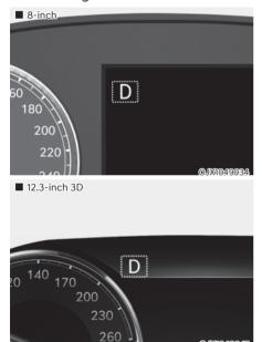
The indicator displays which gear is selected.
