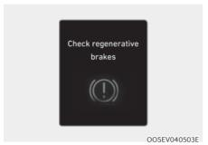
This warning message is displayed when the regenerative brake system does not work properly.
