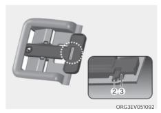
2. With the lever pulled to the end, fix the lever (3) on the projecting part (2).
