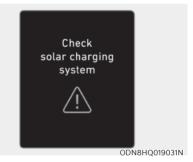
When the solar roof controller is not working properly, the 'Check solar charging system' warning message will appear on the cluster. We recommend to take your vehicle to an authorized retailer of Genesis Branded products and have the system checked.
