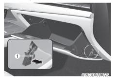
1. Open the glove box and remove the support rod (1).
