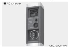
When charging is complete, remove the charging plug from the electrical outlet of the AC charging station.
