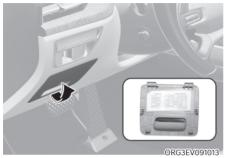
Inside the fuse/relay box cover, you can find the fuse/relay label describing fuse/relay names and ratings.
