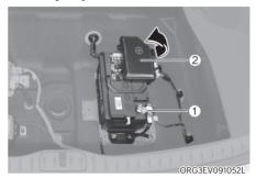
When replacing the battery, disconnect negative (-) cable (1) and remove positive (+) battery fuse box (2). Reassemble in the reverse order of disassembly.
