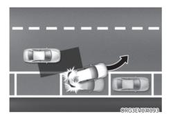
When you are driving forward out of a parking space, if Blind-Spot Collision-Avoidance Assist judges that there is a collision risk with an approaching vehicle in the blind spot, it can help avoid collision by applying the brake.
