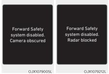
When the front windshield where the front view camera is located, front radar cover, bumper or sensor is covered with foreign material, such as snow or rain, it can reduce the detecting performance and temporarily limit or disable Forward Collision-Avoidance Assist.
