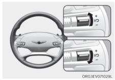
To resume Manual Speed Limit Assist after the function was paused, push the +, -, || \( \) switch.
