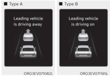
When a detected vehicle in front departs from a stop, Leading Vehicle Departure Alert will inform the driver by displaying the 'Leading vehicle is driving away' (or 'Leading vehicle is driving on') message on the cluster and an audible warning will sound.
