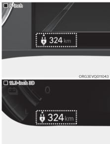
The distance to empty is the estimated distance the vehicle can be driven with the remaining electric energy.
