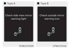
When the outside rearview mirror warning light is not working properly, the 'Check side view mirror warning light' (or 'Check outside mirror warning icon') warning message will appear on the cluster for several seconds, and the master (\(\(\Lambda\)\)) warning light will illuminate on the cluster. If this occurs, we recommend that the vehicle be inspected by an authorized retailer of Genesis Branded products.
