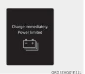
When the high voltage battery level reaches below approximately 6 %, this warning message is displayed.
