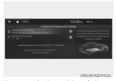
You can set the date and time of when to charge the battery and the climate control temperature. Also, you may select the time to start charging using the off-peak time setting.
