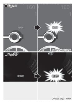
When the ready (READY) indicator is ON, you can drive the vehicle.
