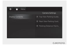
You can change Rear View Monitor 'Display Contents' or 'Display Settings' by touching the setup icon (♠) on the screen while Rear View Monitor is operating, or selecting 'Driver Assistance → Parking Safety → Camera Settings' from the Settings menu while the vehicle is on.
