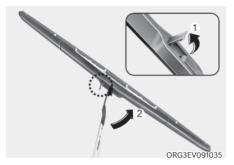
1. Lift up the wiper blade clip (1). Then lift up the wiper blade (2).
