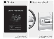
If you do not want to use Rear Occupant Alert, press the OK button on the steering wheel when the first alert is displayed on the cluster. Doing so will deactivate the second alert one time.
