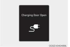
This message is displayed when the vehicle is driven with the charging door opened. Close the charging door and then start driving.
