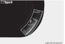
Pulling the paddle-shift ( ) for 1 or more seconds, the smart recuperation system will operate. The indicator of the regenerative braking will be changed to 'AUTO' from the level indicator.
