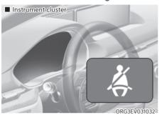
As a reminder to the driver, the seat belt warning light will illuminate for approximately 6 seconds each time the Start/Stop button is in the ON or START position regardless of belt fastening.
