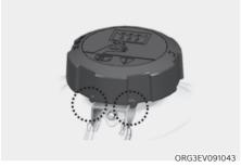
Make sure that the tiny protrusions inside the coolant cap are securely interlocked.
