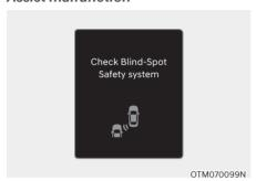
When Blind-Spot Collision-Avoidance Assist is not working properly, the 'Check Blind-Spot Safety system(s)' warning message will appear on the cluster for several seconds, and the master (\(\(\Lambda\)\)) warning light will illuminate on the cluster. If this occurs, we recommend that the vehicle be inspected by an authorized retailer of Genesis Branded products.
