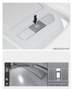
Surround View Monitor will assist in parking by allowing the driver to see around the vehicle.
