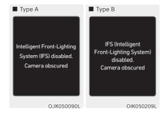
When the front view camera is covered with dirt, snow, or debris, Intelligent Front-Lighting System may temporarily not work properly. If this occurs, a warning message will appear on the cluster.
