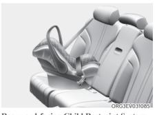
Rearward-facing Child Restraint System A rearward-facing Child Restraint System provides restraint with the seating surface against the back of the child. The harness system holds the child in place, and in an accident, acts to keep the child positioned in the Child Restraint Systems and reduce the stress to the fragile neck and spinal cord.
