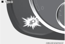
7. Check if the charging indicator light (s) of the high voltage battery in the instrument cluster is turned ON. Charging is not active when the charging indicator light (s) is OFF. When the charging connector is not connected properly, reconnect the charging cable to charge it again. During cold weather, DC charging may not be available to prevent high voltage battery degradation.
