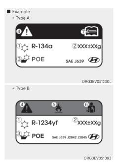
Each symbols and specification on the air conditioning refrigerant label is represented as below:
