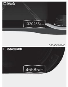
The odometer indicates the total distance that the vehicle has been driven and should be used to determine when periodic maintenance should be performed.
