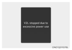
V2L stopped due to excessive power use If you use an electrical appliance that exceeds the maximum power output the vehicle can supply, it will stop working and display a warning message. Make sure that the total power consumption of your electrical appliance exceeds the V2L maximum power output.
