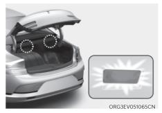
The trunk lamp comes on when the trunk is opened.
