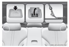
Top-tether anchorages for Child Restraint Systems are located on the package tray.
