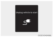
This message is displayed when you start the vehicle without unplugging the charging cable. Unplug the charging cable, and then turn on the vehicle.
