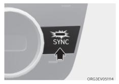
Adjusting the temperature, air flow direction and fan speed equally
