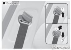
To adjust the height of the seat belt anchor, lower or raise the height adjuster into an appropriate position.
