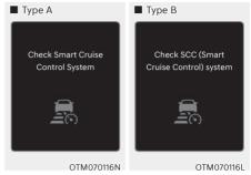
When Smart Cruise Control is not working properly, the 'Check Smart Cruise Control system' (or 'Check SCC (Smart Cruise Control) system') warning message will appear, and the \(\text{N}\) warning light will illuminate on the cluster. If this occurs, we recommend that the vehicle be inspected by an authorized retailer of Genesis Branded products.
