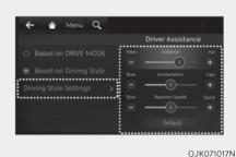
**Driving Style Settings (if equipped)** With the vehicle on, select 'Driver Assistance → Smart Cruise Control → Driving Style Settings' from the Settings menu to check the driver's driving style, and to change each driving style manually.
