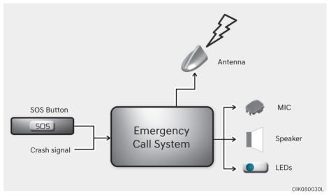
Overview of the 112-based eCall in-vehicle system, its operation and functionalities: refer to this section. The 112-based eCall service is a public service of general interest and is accessible free of charge.
