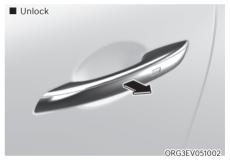
Put your hand in the front outside door handle while carrying the Smart Key with you or press the Door Unlock button on the Smart Key, all doors will unlock.
