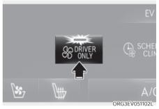
If you press the DRIVER ONLY button (\$\mathbb{G} \text{PRIVER} \text{ only} \text{ and the indicator light illuminates in the infotainment climate control screen, cold air mostly blows in the driver's seat. However, some of the cold air may come out of other seating position ducts to keep indoor air pleasant.
