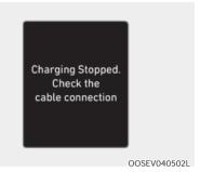
This warning message is displayed when charging is stopped because the charging connector is not correctly connected to the charging inlet
