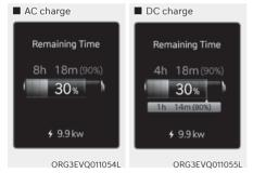
This message is displayed to notify the remaining time to charge the battery to the selected target battery charge level.
