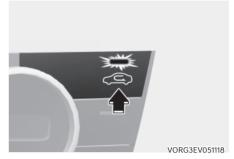
The air intake control button is used to select either Fresh mode (outside air) or Recirculation mode (cabin air).
