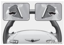
The paddle shifter is used to adjust the regenerative braking level from 0 to 3 during decelerating.
