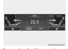
You can also adjust the rear seat warmers from the front seats. With the vehicle running, touch the seat warmer icon on the climate control system screen.
