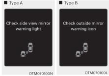
When the outside rearview mirror warning light is not working properly, the 'Check side view mirror warning light' (or 'Check outside mirror warning icon') warning message will appear on the cluster for several seconds, and the master (\(\frac{\(\chi\)}{\(\chi\)}\)) warning light will illuminate on the cluster. If this occurs, we recommend that the vehicle be inspected by an authorized retailer of Genesis Branded products.
