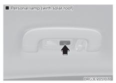
Press the button to turn the lamp on or off.
