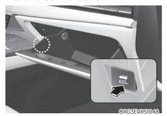
When the trunk lid control button is in the UNLOCK (button not pressed) position, the power trunk can be controlled with the power trunk main control button, power trunk open switch, power trunk close button, and the smart key.
