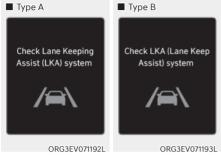
When Lane Keeping Assist is not working properly, the 'Check Lane Keeping Assist (LKA) system' (or 'Check LKA (Lane Keeping Assist) system') warning message will appear and the yellow indicator light will illuminate on the cluster. If this occurs, we recommend that the vehicle be inspected by an authorized retailer of Genesis Branded products.
