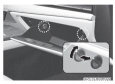
Remove the stoppers on both sides to allow the glove box to hang freely on the hinges.
