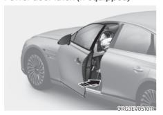
If a door isn't closed completely but is closed to the first detent position, the door will close automatically.
