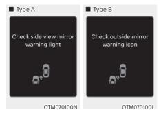
When the outside rearview mirror warning light is not working properly, the 'Check side view mirror warning light' (or 'Check outside mirror warning icon') warning message will appear on the cluster for several seconds, and the master (\(\frac{\Lambda}{\Lambda}\)) warning light will illuminate on the cluster. If this occurs, we recommend that the vehicle be inspected by an authorized retailer of Genesis Branded products.
