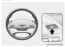
Press the Driving Assist (( ) button to turn Manual Speed Limit Assist off. The Speed Limit (( ) LIMIT) indicator will go off.
