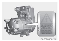
A compressor label informs you the type of compressor your vehicle is equipped with such as model (1), serial number (2), supplier part number (3), lot number (4), refrigerant (4) and refrigerant oil (5).
