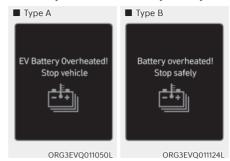
This warning message is displayed to protect battery and electric vehicle system when the high voltage battery temperature is too high.
