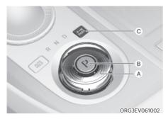
[A]: Rotary shifter(Rotary gear shift dial),
