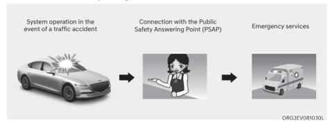
The UAE eCall device automatically makes an emergency call to the Public Safety Answering Point (PSAP) for proper rescuing operations in event of vehicle accident.
