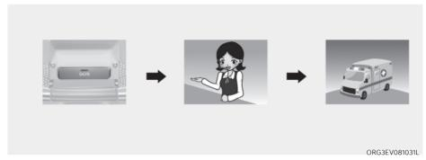
The driver or passenger manually can make an emergency call in the Public Safety Answering Point(PSAP), by pressing SOS button to call the necessary emergency services.
