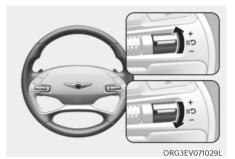
Push the + switch up or - switch down, and release it at the desired speed.
