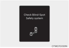
When Safe Exit Assist is not working properly, the 'Check Blind-Spot Safety system(s)' warning message will appear on the cluster for several seconds, and the master (A) warning light will illuminate on the cluster. If this occurs, we recommend that the vehicle be inspected by an authorized retailer of Genesis Branded products.
