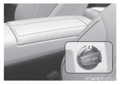
Plug the compressor power cord (4) into the vehicle power outlet.
