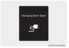
This message is displayed when the vehicle is driven with the charging door opened. Close the charging door and then start driving.
