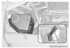
Pull down the yellow lever in the high voltage cut-off switch to shut down high voltage battery.
