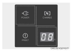
2. Check if the power lamp (green) illuminates on the control box.
