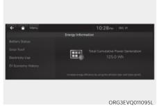
Select 'Solar Roof Info' from the infotainment system menu to check the solar roof's 'Total Cumulative Power Generation'.
