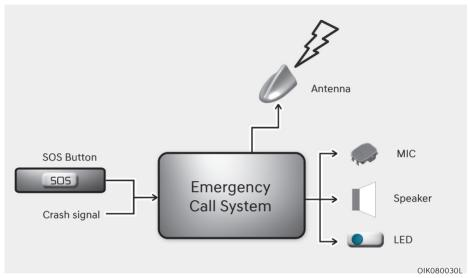
Overview of the 999-based eCall in-vehicle system, its operation and functionalities: refer to this section. The 999-based eCall service is a public service of general interest and is accessible free of charge.
