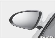
Your vehicle is equipped with both lefthand and right-hand outside rearview mirrors. The mirrors can be adjusted remotely with the remote switch. The outside rearview mirrors can be folded to help prevent damage when going through an automatic car wash or when passing through a narrow street.
