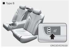
While the vehicle is running, press either of the seat warmer switches to warm the rear seat. Manual temperature control
