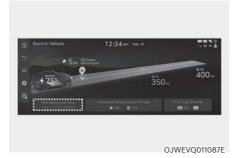
Select 'EV → Next Departure' on the screen. You can set the date and time of when to charge the battery, climate control temperature, and other various functions.
