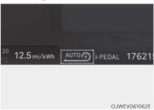
Pulling the paddle-shift (-1) for 1 or more seconds, the smart recuperation system will operate. The indicator of the regenerative braking will be changed to 'AUTO' from the level indicator.
