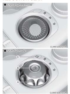
[A]: Rotary shifter(Rotary gear shift dial),
