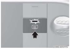
The defroster heats the window to remove frost, fog and thin ice from the interior and exterior of the rear window, whilst the vehicle is running.
