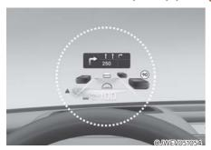
The Head-Up Display is an optional feature that allows the driver to view information projected onto a transparent screen whilst still keeping your eyes safely on the road ahead whilst driving.
