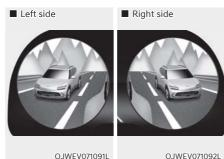
Blind-Spot View Monitor displays the rear blind spot area of the vehicle in the cluster when the turn signal is turned on to help safely change lanes.
