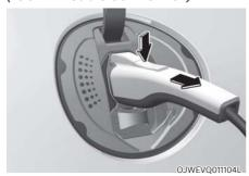
Hold the charging connector handle and pull it out.
