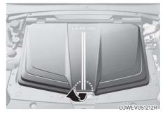
Lift up the front storage compartment cover whilst depressing the front storage compartment lever (1).
