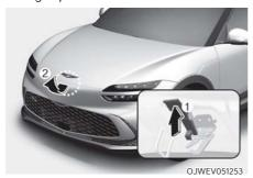
Go to the front of the vehicle, raise the bonnet slightly, push up the secondary latch (1) inside of the bonnet centre and lift the bonnet (2).
