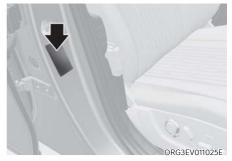
All specifications (sizes and pressures) can be found on a label attached to the driver's side centre pillar.
