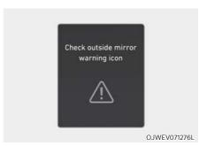
When the outside rearview mirror warning light is not working properly, the 'Check outside mirror warning icon' warning message will appear on the cluster for several seconds, and the master (八) warning light will illuminate on the cluster. If this occurs, we recommend that the vehicle be inspected by an authorised retailer of Genesis Branded products.
