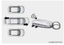
(1) Press and hold one of the Forward (()) or Backward (()) button on the smart key. Remote Smart Parking Assist will automatically control the steering wheel, vehicle speed and gearshift. The vehicle will move in the direction of the button pressed.
