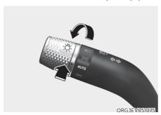
High Beam Assist will automatically switch between high beam and low beam depending on the detected brightness from the lamps of oncoming vehicles or vehicles in front.
