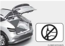
Do not hold on to or try to pull on the tailgate strut. Be aware that the deformation of the tailgate strut may cause vehicle damage and risk of injury.
