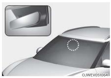
Auto defogging helps reduce the possibility of fogging up the inside of the windscreen by automatically sensing the moisture on inside the windscreen.
