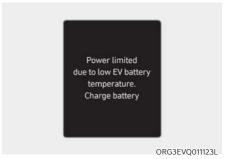
Both warning messages are displayed to protect electric vehicle system when outside temperature is low. If the high voltage battery charging level is low and parked outside in low temperature for a long time, vehicle power could be limited.
