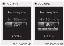
This message displays how much time remains until the battery is charged to the selected target battery charge level.
