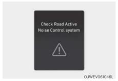
When Active noise control - road is not working properly, this warning message will appear on the cluster LCD display. If this occurs, we recommend that the system be inspected by an authorised retailer of Genesis Branded products.
