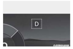
The indicator displays which gear is selected.
