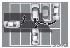
Rear Cross-Traffic Collision-Avoidance Assist may detect vehicles which are parking or pulling out near your vehicle (example, a vehicle leaving beside your vehicle, a vehicle parking or pulling out in the rear area, a vehicle approaching your vehicle making a turn, etc.). If this occurs, the function may unnecessarily warn the driver and control the brake.
