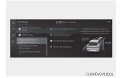
The regenerative braking level can be adjusted based on the driver's deceleration style (Faster/Normal/Slower Deceleration)
