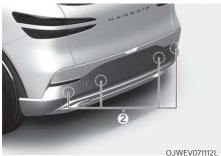
[1]: Front ultrasonic sensors, [2]: Rear ultrasonic sensors
