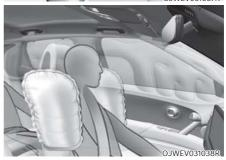
Your vehicle is equipped with a side air bag in each front. Additionally, a front centre side air bag is provided in the inboard side of the driver seatback. The purpose of the air bag is to provide the vehicle's additional protection than that offered by the seat belt alone.
