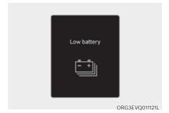
When the high voltage battery level reaches below approximately 12%, this warning message is displayed.
