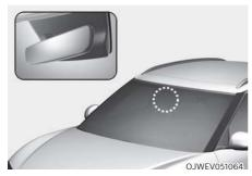
The rain sensor located on the upper end of the windscreen glass senses the amount of rainfall and controls the wiping cycle for the proper interval.
