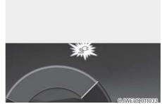
Check if the charging indicator light (s) of the high voltage battery in the instrument cluster is turned ON. Charging is not active when the charging indicator light (s) is OFF.
