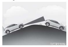
When coasting on an uphill or downhill, the system may not detect the vehicle in your lane and the regenerative braking level will reduce automatically, making you feel that the vehicle is accelerating.
