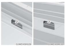
2. Remove the cover by pulling the front storage compartment handle (2).
