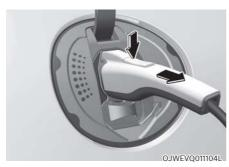
2. Hold the charging connector handle and pull it out.
