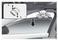
If a window senses any obstacle whilst it is closing automatically, it will stop and lower approximately 12 in. (30 cm) to allow the object to be cleared.
