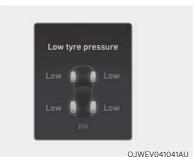
When the tyre pressure monitoring system warning indicators are illuminated and a warning message displayed on the cluster LCD display, one or more of your tyres is significantly under-inflated. The Low Tyre Pressure Position Telltale will indicate which tyre is significantly underinflated by illuminating the corresponding position light.
