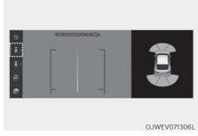
When you touch the icon, the top view is displayed on the screen and shows the distance from the vehicle in the back of your vehicle whilst parking.
