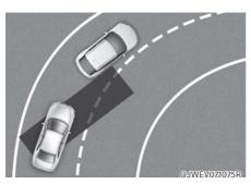
Blind-Spot Collision-Avoidance Assist may not operate properly when driving on a curved road. The function may recognise a vehicle in the same lane.
