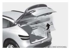
During power opening or closing if the power tailgate senses any obstacle, the power tailgate will stop and move in the opposite direction.
