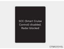
When the front radar cover or sensor is covered with snow, rain, or foreign material, it can reduce the detecting performance and temporarily limit or disable Smart Cruise Control.
