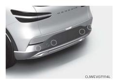
The rear ultrasonic sensors are located inside the rear bumper to detect objects in the rear area. If the sensors are covered with foreign material, such as snow or rain, it may adversely affect sensor performance and Reverse Parking Collision-Avoidance Assist may not operate properly. Always keep the rear bumper clean.
