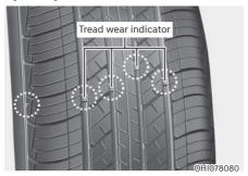
If the tyre is worn evenly, a tread wear indicator will appear as a solid band across the tread. This shows there is less than 1/16 in. (1.6 mm) of tread left on the tyre. Replace the tyre when this happens. Do not wait for the band to appear across the entire tread before replacing the tyre.
