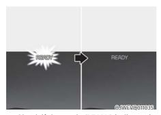
5. Check if the ready (READY) indicator is turned OFF on the instrument cluster. When the ready (READY) indicator is ON and the gear is in a position other than P (Park), the driver can accidently depress the accelerator pedal, causing the vehicle to move unexpectedly.
