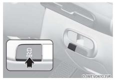
Electronic Stability Control helps to stabilize the vehicle during cornering manoeuvres.
