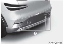
[1]: Rear view camera,[2]: Rear ultrasonic sensors
