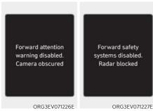
When the front windscreen where the front view camera is located, front radar cover, bumper or sensor is covered with foreign material, such as snow or rain, it can reduce the detecting performance and temporarily limit or disable Forward Collision-Avoidance Assist.
