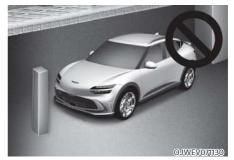
Remote Smart Parking Assist performance may reduce or collision with an obstacle may occur when there is a narrow object, circular pillar, square pillar, or a pillar surrounded by objects such as a fire extinguisher, etc., near the parking space. The driver should park the vehicle properly.
