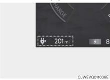
The distance to empty is displayed differently according to the selected drive mode in the Drive Mode Integrated Control System.
