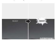
When the ready (READY) indicator is ON, you can drive the vehicle.
