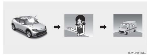
The Pan-European eCall device automatically makes an emergency call to the Public Safety Answering Point (PSAP) for proper rescuing operations in event of vehicle accident.
