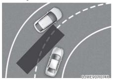
Blind-Spot Collision-Avoidance Assist may not operate properly when driving on a curved road. The function may not detect the vehicle in the next lane.
