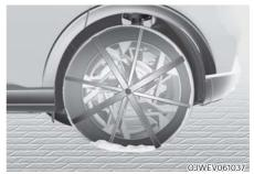
Since the sidewalls of radial tyres are thinner, they can be damaged by mounting some types of snow chains on them. Therefore, the use of snow tyres is recommended instead of snow chains.
