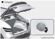
The power outlet is designed to provide power for mobile telephones or other devices designed to operate with vehicle electrical systems. The devices should draw less than 180 W with the vehicle running.
