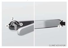
Press the front part (1) of the door handle to pull out the rear part of the door handle. Whilst keep pressing the front part of the door handle, insert (2) the mechanical key to the lock.
