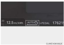
When pull and hold the right side paddle shifter for 1 second or more, Smart Recuperation System is On. When Smart Recuperation System is On, 'AUTO' for the regenerative braking level is displayed on the cluster.
