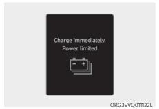
When the high voltage battery level reaches below approximately 6%, this
