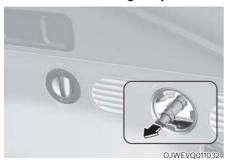
If the charging connector does not disconnect from the charging inlet due to battery discharge and failure of electric wires, open the tailgate and slightly pull the emergency cable located on the right side of the cargo area. The charging connector will be disconnected from the charging inlet.
