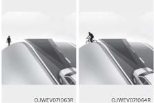
Forward Collision-Avoidance Assist may not detect other vehicles, pedestrians or cyclists in front of you whilst driving uphill or downhill, adversely affecting the performance of the sensors.
