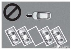
Remote Smart Parking Assist does not provide diagonal parking. Even if your vehicle was able to enter the parking space, do not use Remote Smart Parking Assist because the function cannot operate properly.
