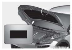
You can find out which air conditioning refrigerant is applied to your vehicle on the label located inside of the bonnet.
