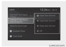
With the Start/Stop button in the ON position, select 'Lights → Intelligent High Beams (or Smart High Beam)' from the Settings menu to turn on Intelligent Front-Lighting System and deselect to turn off the system.
