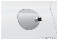
5. Push the charging door where the triangle symbol (1) is located to open. The charging door opens only when the vehicle is unlocked.
