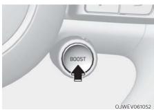
Controls motor to maximum performance when pressing BOOST button on the steering wheel remote control in situations where rapid acceleration is required.
