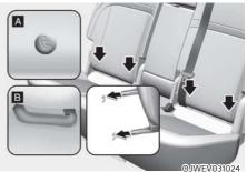
[A]: ISOFIX Anchorage Position Indicator (Type A- ( ,Type B- ), [B]: ISOFIX Anchorage
