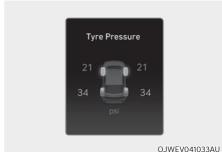
Tyre pressure / Tyre pressure The tyre pressure of each tyre is displayed.
