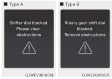
This message is displayed when motion is not possible due to obstacles around the shift dial. We recommend that you have to clean obstruction around the shift dial.
