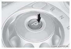
To shift the gear to P (Park), press the P button whilst depressing the brake pedal. If you turn the vehicle off in R (Reverse), N (Neutral) or D (Drive), the gear will automatically shift to P (Park).
