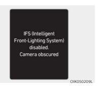
When the front view camera is covered with dirt, snow, or debris, Intelligent Front-Lighting System may temporarily not work properly. If this occurs, a warning message will appear on the cluster.
