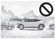
Snow may interfere with sensor operation, or Remote Smart Parking Assist may cancel if the road is slippery whilst parking.
