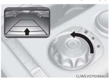
Rear View Monitor shows the area behind the vehicle to assist you when parking or backing up.
