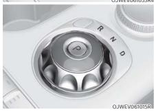
If the drivable indicator (READY) is on and it cannot rotate normally in 'shift dial mode', try restarting the vehicle by pressing the start button. If the same phenomenon repeats after restarting, pull the upper surface of the crystal sphere strongly toward the rear of the vehicle with your palm and rotate it until the shift dial is fully visible. At this time, you may hear a normal 'click' sound, which releases the restraint of the instrument.
