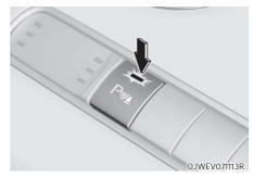
If Parking Safety (P™) button is pressed more than 2 seconds, 'Rear Active Assist' or 'Rear Warning Only' can be turned on or off.
