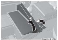
5. Remove the fastener (1) located inside of the front trunk after then remove the battery cover (2).
