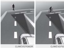
Forward Collision-Avoidance Assist may detect a vehicle, pedestrian or cyclist in the next lane or outside the lane when driving on a curved road.
