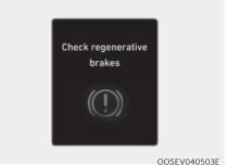
These warning messages are displayed when the regenerative brake system does not work properly.
