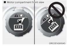
Check if the coolant cap label is straight in front.
