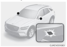
When all doors (and tailgate) are closed and locked, the puddle lamp will turn on for 15 seconds if the door is unlocked by the smart key or when you put your hand in the outside door handle with the smart key in possession.
