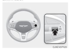
Press the [] Switch to temporarily pause the set speed limit. The set speed limit will turn off but the Speed Limit (©] [IMIT] indicator will stay on.
