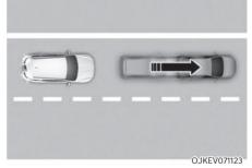
If the vehicle in front abruptly departures, Leading Vehicle Departure Alert may not operate properly.
