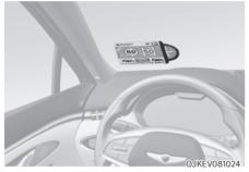
Detach the speed restriction label from the sealant bottle (2), and place it in a highly visible place inside the vehicle to remind the driver not to drive too fast.
