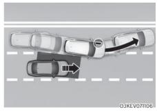
When changing lanes by detecting the lane ahead, if Blind-Spot Collision-Avoidance Assist detects that there is a collision risk with an approaching vehicle in the blind spot, it can help avoid collision by applying the brake.
