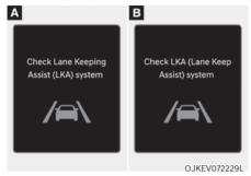
When Lane Keeping Assist is not working properly, the 'Check Lane Keeping Assist (LKA) systems' (or 'Check LKA (Lane Keep Assist) system') warning message will appear and the yellow indicator light will illuminate on the cluster. If this occurs, we recommend that the vehicle be inspected by an authorized retailer of Genesis Branded products.
