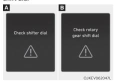
This message is displayed when there is a malfunction with the rotary gear shift dial.
