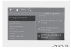
With the vehicle on, select 'Driver assistance → Driving convenience → Motorway Auto Speed Change (Highway Auto Speed Change)' from the Settings menu to turn on Navigation-based Smart Cruise Control and deselect to turn off
