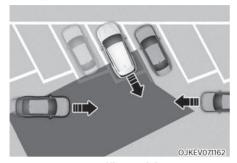
Rear Cross-Traffic Collision-Avoidance Assist may be limited when backing up diagonally, and may not detect the vehicle approaching from the left or right. If this occurs, the function may not warn the driver or control the brakes when necessary.
