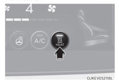
Touch CLIMATE icon in the climate control panel. The climate information screen will appear on the infotainment screen. Touch the HEAT icon in the infotainment screen to turn the heater on (indicator light will illuminate).
