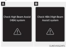
When High Beam Assist is not working properly, the 'Check High Beam Assist (HBA) system' (or 'Check HBA (High Beam Assist) system) warning message will appear and A warning light will illuminate on the cluster. We recommend that the function be inspected by an authorized retailer of Genesis Branded products.
