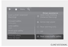
With the vehicle on, select 'Driver assistance → parking safety → Rear crosstraffic safety' from the Settings menu to turn on Rear Cross-Traffic Collision-Avoidance Assist and deselect to turn off the function.
