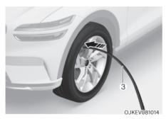
5. Unscrew the valve cap from the valve of the defective wheel and screw the filling hose (3) of the sealant bottle onto the valve.
