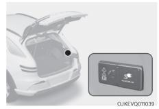
Connect to the power outlet located on the lower right side of the tailgate with the Vehicle Stop/Start button in the ON position.
