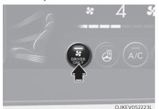
If you touch the DRIVER ONLY icon (\$\mathbb{S}^{\text{DRIVER}})\$ and the indicator light illuminates in the infotainment climate control screen, cold air mostly blows in the driver's seat. However, some of the cold air may come out of other seating position ducts to keep indoor air pleasant.
