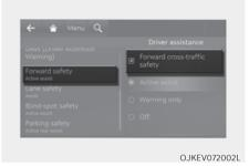
With the vehicle on, select 'Driver assistance → Forward safety → Forward cross-traffic safety' from the Settings menu to turn on Junction Crossing function and deselect to turn off the function.
