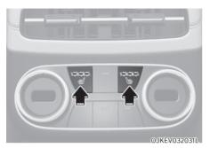
With the READY indicator on, press the seat warmer button on the center console to select the desired temperature level.
