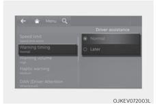
With the vehicle on, select 'Driver assistance → Warning timing' from the Settings menu to change the initial warning activation time for Forward Collision-Avoidance Assist. The warning time can be set to either 'Normal (Standard)' or 'Later'.
