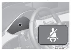
As a reminder to the driver, the seat belt warning light will illuminate for approximately 6 seconds each time the Start/Stop button is in the ON position regardless of belt fastening.
