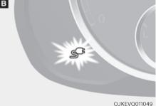
9. Check if the charging indicator light (\$\( \sigma^\* \)) of the high voltage battery in the instrument cluster is turned ON. Charging is not active when the charging indicator light (\$\( \sigma^\* \)) is OFF. When charging cable is not connected properly to inlet, press release button, remove charging cable and reconnect again.
