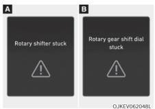
This message is displayed when the rotary gear shift dial does not return back to it's normal position after rotating it.
