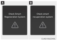
If the smart recuperation system is turned off due to the front sensors being covered with the foreign substances or due to other causes, the above warning message is displayed. Also the regenerative braking level is displayed instead of 'AUTO'.
