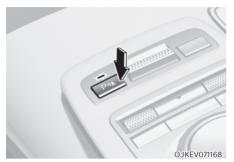
Press and hold the Parking Safety (P™) button more than 2 seconds, 'Active rear assist' or to turn the Parking Collision-Avoidance Assist on or off.
