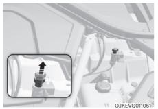
If the charging connector does not disconnect from the charging inlet due to battery discharge and failure of electric wires, open the hood and slightly pull the emergency cable. The charging connector will be disconnected from the charging inlet.
