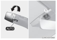
The position lamp and headlamp will be turned ON or OFF automatically depending on the amount of daylight as measured by the ambient light sensor (1) at the upper end of the windshield glass.
