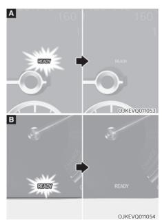
5. Check if the ready (READY) indicator is turned OFF on the instrument cluster. When the ready (READY) indicator is ON and the gear is in a position other than P (Park), the driver can accidently depress the accelerator pedal, causing the vehicle to move unexpectedly.
