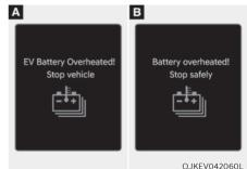
This warning message is displayed to protect battery and electric vehicle system when the high voltage battery temperature is too high.
