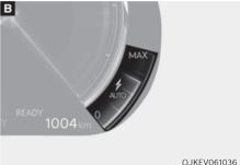
The smart recuperation system is ON and the regenerative braking level is displayed as AUTO.
