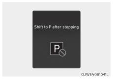
This message is displayed when the gear is shifted to P (Park) while the vehicle is moving.
