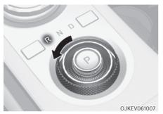
To shift the gear to R (Reverse), rotate the rotary gear shift dial to R (Reverse) while depressing the brake pedal.
