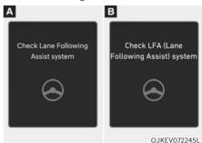
When Lane Following Assist is not working properly, the 'Check LFA (Lane Following Assist) system' (or 'Check Lane Following Assist system') warning message will appear for several seconds, and the master (A) warning light will illuminate on the cluster. If this occurs, we recommend that the vehicle be inspected by an authorized retailer of Genesis Branded products.
