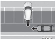
Rear Cross-Traffic Collision-Avoidance Assist may detect vehicles passing by behind you when parking in reverse into a parking space. If this occurs, the function may unnecessarily warn the driver and control the brake.
