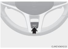
Boost mode will maximize motor performance for up to 10 seconds for rapid acceleration.
