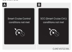
If the Driving Assist button, + switch, - switch or II > switch is operated when Smart Cruise Control operating conditions are not satisfied, the 'Smart Cruise Control conditions not met' (or 'SCC (Smart Cruise Ctrl.) conditions not met') will appear on the cluster, and an audible warning will sound.
