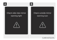
When the outside rearview mirror warning light is not working properly, the 'Check side view mirror warning light' (or 'Check outside mirror warning icon') warning message will appear on the cluster for several seconds, and the master (\(\beta\)) warning light will illuminate on the cluster. If this occurs, we recommend that the vehicle be inspected by an authorized retailer of Genesis Branded products.
