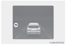
When driving at a speed higher than the displayed speed limit, the speed limit is displayed in red.
