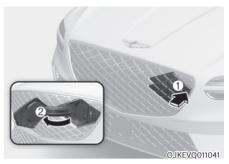
Push the charging door where the triangle symbol (1) is located to open. The charging door opens only when the vehicle is unlocked.
