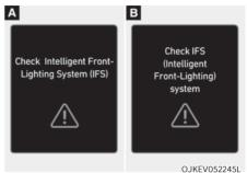
When Intelligent Front-Lighting System is not working properly, the 'Check Intelligent Front-Lighting System (IFS)' (or 'Check IFS (Intelligent Front-Lighting) system) warning message will come on for a few second on the cluster. After the message disappears, AFS and \( \text{\text{\text{\text{Marning} lights will illuminate on the cluster.} \) We recommend that the system be inspected by an authorized retailer of Genesis Branded products.
