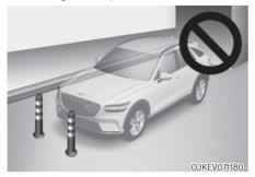
Remote Smart Parking Assist performance may reduce or collision with an obstacle may occur when there is a narrow object, circular pillar, square pillar, or a pillar surrounded by objects such as a fire extinguisher, etc., near the parking space. The driver should park the vehicle properly.
