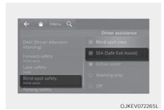
With the vehicle on, select 'Driver assistance → Blind-spot safety → SEA (Safe Exit Assist)' from the Settings menu to turn on Safe Exit Assist and deselect to turn off the function.
