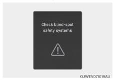
When Safe Exit Warning is not working properly, the 'Check blind-spot safety system(s)' warning message will appear on the cluster for several seconds, and the master ((\frac{1}{2}\)) warning light will illuminate on the cluster. If this occurs, we recommend that the vehicle be inspected by an authorized retailer of Genesis Branded products.
