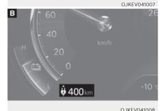
The distance to empty range displayed will vary depending upon which drive mode is selected in Drive Mode Integrated Control System.
