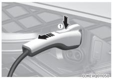
2. Press release button (1), then remove charging connector from the vehicle inlet.
