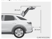
Make sure that there are no people or objects in the path of the power tailgate or smart tailgate prior to use. Serious injury, damage to the vehicle or damage to surrounding objects (for example, walls, ceilings, vehicles, etc.) may result if contact with the tailgate occurs.
