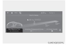
Select 'EV → Next departure time' on the screen. You can set the date and time of when to charge the battery, climate control temperature, and other various functions.
