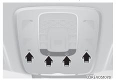
Touch either icons to turn the map lamp on or off. This light produces a spot beam for convenient use as a map lamp at night or as a personal lamp for the driver and the front passenger.
