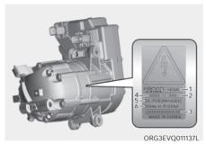
A compressor label informs you the type of compressor your vehicle is equipped with such as model (1), serial number (2), supplier part number (3), lot number (4), refrigerant (5) and refrigerant oil (6).
