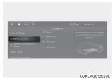
You can adjust the charging current for an AC charger. Select an
