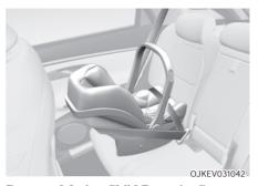
Rearward-facing Child Restraint System A rearward-facing Child Restraint System provides restraint with the seating surface against the back of the child. The harness system holds the child in place, and in an accident, acts to keep the child positioned in the Child Restraint Systems and reduce the stress to the fragile neck and spinal cord.
