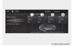
In order to check the current energy consumption for each system of the vehicle, select 'EV → Energy information' on the screen.
