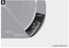
The selected regenerative braking level is displayed on the instrument cluster. When the vehicle is turned off and on again after the regenerative braking level is lowered to 0 or i-PEDAL, the braking level will change to 1.
