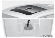
Push the sunroof switch rearward to the first detent position, the sunroof glass opens. However, if the power sunshade is closed, the power sunshade will open first.
