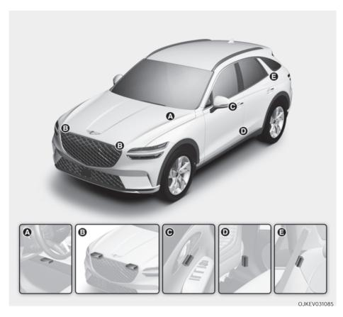
(A): SRS control module/Rollover sensor
