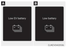
When the high voltage battery level reaches below approximately 10%, this warning message is displayed.
