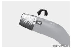
The position lamp, license plate lamp and instrument panel lamp are turned ON.
