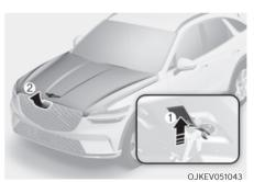
3. Go to the front of the vehicle, raise the hood slightly, push up the secondary latch (1) inside of the hood center and lift the hood (2).
