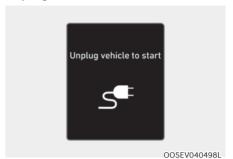
This message is displayed when you start the vehicle without unplugging the charging cable. Unplug the charging cable, and then turn on the vehicle.
