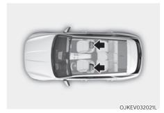
The driver's and front passenger's seats are equipped with adjustable headrests for the passengers safety and comfort.
