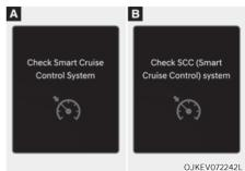
When Smart Cruise Control is not working properly, the 'Check Smart Cruise Control System' (or 'Check SCC (Smart Cruise Control) system') warning message will appear, and the \(\textit{N}\) warning light will illuminate on the cluster. If this occurs, we recommend that the vehicle be inspected by an authorized retailer of Genesis Branded products.
