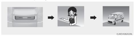
The driver or passenger manually can make an emergency call in the Public Safety Answering Point (PSAP), by pressing SOS button to call the necessary emergency services.
