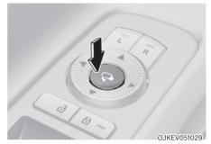
The rearview mirrors can be folded or unfolded by pressing the button.
