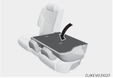
4. Pull up the seatback folding lever, then fold the seat toward the front of the vehicle. When you return the seatback to its upright position, always be sure it has locked into position by pushing on the top of the seatback.
