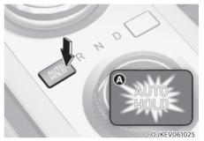
With the driver's door and hood closed, depress the brake pedal and then press the AUTO HOLD switch. The white AUTO HOLD indicator will come on and the system will be in the standby position.
