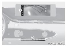
The front image is displayed on the screen when the gear is in N (Neutral) or D (Drive) to assist in parking. Using the view button (2) you may select top view, front view, side view and 3D view.
