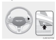
Press the Driving Assist button to turn Smart Cruise Control off.
