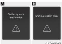
This message is displayed when the shift gear does not properly operate in the P (Park) position.
