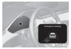
To warn the driver of a collision, the warning light on the outside rearview mirror will blink and a warning message will appear on the cluster. At the same time, an audible warning will sound, warning light on the headup display will blink and the steering wheel will vibrate.
