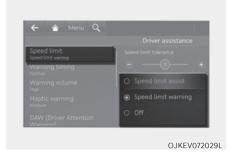
With the vehicle on, select or deselect 'Driver assistance → Speed limit' from the Settings menu to set whether to use each function.
