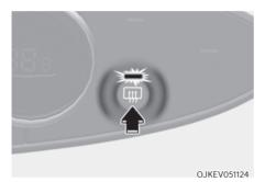
The defroster heats the window to remove frost, fog and thin ice from the interior and exterior of the rear window, while the READY indicator is on.
