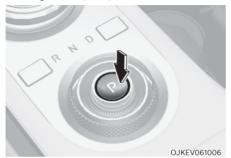
To shift the gear to P (Park), press the P button while depressing the brake pedal. If you turn the vehicle off in R (Reverse), N (Neutral) or D (Drive), the gear will automatically shift to P (Park).
