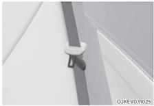
Route the seat belt webbing through the rear seat belt guides to prevent the belts from being trapped behind or under the seats.
