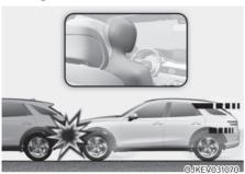
In certain low-speed collisions the air bags may not deploy. The air bags are designed not to deploy in such cases because they may not provide benefits beyond the protection of the seat belts.
