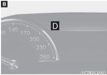
The indicator displays which gear is selected.
