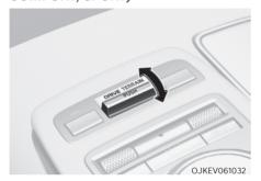
The mode changes whenever the driver pushes the DRIVE MODE switch up or down.
