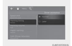
With the vehicle on, select 'Driver assistance → Warning timing' from the Settings menu to change the initial
