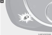
8. Check if the charging indicator light (⑤) of the high voltage battery on the instrument cluster is turned ON. Charging is not active when the charging indicator light (⑤) is OFF. If the charging cable is not connected to the vehicle side inlet properly, charging may not start. In this case, try reconnecting charging cable to the vehicle inlet again.
