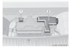
When replacing the battery, disconnect negative (-) cable (1) and remove positive (+) battery fuse box (2). Reassemble in the reverse order of disassembly.
