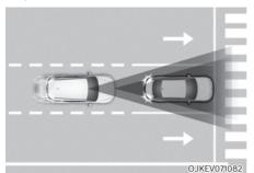
Forward Collision-Avoidance Assist is designed to help detect and monitor the vehicle ahead or help detect a pedestrian or cyclist in the roadway and warn the driver that a collision is imminent with a warning message and warning and application of emergency braking.
