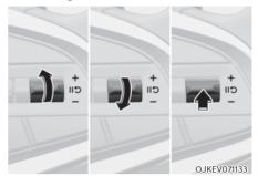
To resume Smart Cruise Control after the function was cancelled, operate the +, - or II  $\Sigma$  switch.
