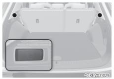
Pull the rear seat back folding switch located in the both sides of the cargo area.
