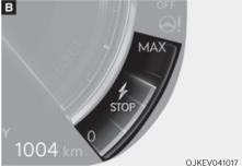
The regenerative brake indicates the level of the regenerative braking that you set. And it also indicates Smart regenerative system's operation status. For more details, refer to "Regenerative Braking System" in chapter 6.
