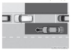
After the vehicle stops, when an approaching vehicle from the rear area is detected after a passenger opens the door, Safe Exit Warning will warn the driver with a warning message and an audible warning to help prevent a collision.
