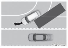
Blind-Spot Collision-Avoidance Assist may not operate properly when driving where the road merges or divides. The function may not detect the vehicle in the next lane.
