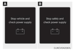
This warning message is displayed when a failure occurs in the power supply system.
