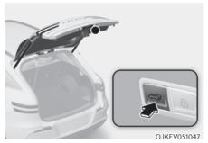
Press the power tailgate open/close button. The tailgate opens or closes with a warning sound.
