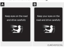
Forward Attention Warning determines whether the driver is focused on the road depending on information, such as the amount of time the driver is looking elsewhere, the amount of time the eyes are closed, how frequently the driver yawns, etc. If Forward Attention Warning judges the driver is not focused, the 'Keep your eyes on the road and drive carefully' (or 'Keep eyes on the road and drive carefully') warning message will appear on the cluster, and an audible warning will sound.
