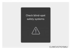
When Blind-Spot Collision-Avoidance Assist is not working properly, the 'Check blind-spot Safety system(s)' warning message will appear on the cluster for several seconds, and the master (\(\(\underline{\Lambda}\)) warning light will illuminate on the cluster. If this occurs, we recommend that the vehicle be inspected by an authorized retailer of Genesis Branded products.
