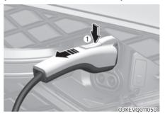
Press release button (1), then remove charging connector from the vehicle inlet
