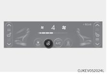
While the READY indicator is on touch the heated steering wheel icon to warm the steering wheel.
