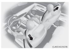
Your vehicle is equipped with driver's and front passenger's and rear passengers Pre-tensioner Seat Belts (Retractor Pre-tensioner). The purpose of the pre-tensioner is to make sure the seat belts fit tightly against the occupant's body in certain frontal or side collision(s). The pre-tensioner seat belts may be activated in crashes where the frontal or side collision(s) is severe enough, together with the air bags.
