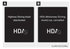
If the driver still does not have their hands on the steering wheel after the hands-off warning, 'HDA( Motorway Driving Assist) sys. cancelled' (or 'Highway Driving Assist deactivated') warning message will appear and Highway Driving Assist and Lane Change Assist will be automatically cancelled.
