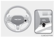
With the vehicle on, shortly press the Lane Driving Assist button located on the steering wheel to turn on Lane Following Assist. The grey or green (a) indicator light will illuminate on the cluster.
