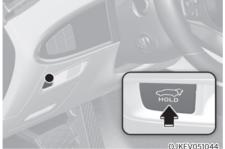
Press the power tailgate open/close button for 1 second. The tailgate opens or closes with a warning sound.
