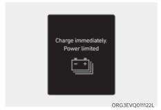
When the high voltage battery level reaches below approximately 5%, this warning message is displayed.
