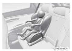
Forward-facing Child Restraint System A forward-facing Child Restraint System provides restraint for the child's body with a harness. Keep children in a forward-facing Child Restraint System with a harness until they reach the top height or weight limit allowed by your Child Restraint System's manufacturer.
