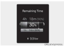
After charging has started, the estimated charging time is displayed on the instrument cluster for about 1 minute.
