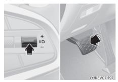
Press the **|| 1** switch or depress the brake pedal to temporarily cancel Smart Cruise Control.
