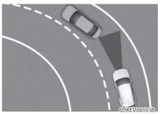
The front sensors may be unable to recognize the foregoing vehicle if you are coasting on a curve. The regenerative braking intensity may automatically be lowered, which may accelerate the vehicle.
