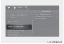
To adjust the regenerative braking level of the smart recuperation system, go to Settings  $\rightarrow$  EV  $\rightarrow$  Smart recuperation from the infotainment system.
