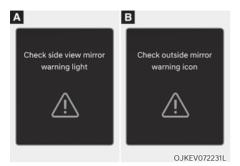
When the outside rearview mirror warning light is not working properly, the 'Check outside mirror warning icon' (or 'Check side view mirror warning light') warning message will appear on the cluster for several seconds, and the master (A) warning light will illuminate on the cluster. If this occurs, we recommend that the vehicle be inspected by an authorized retailer of Genesis Branded products.
