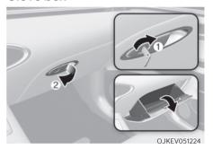
The glove box can be locked and unlocked with the mechanical key (1).
