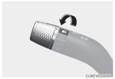
The headlamp, position lamp, license plate lamp and instrument panel lamp are turned ON.
