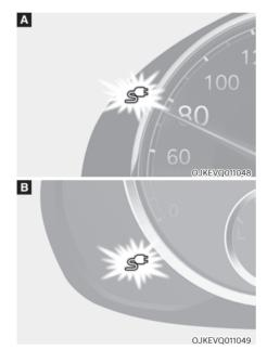
Check if the charging indicator light (s) of the high voltage battery in the instrument cluster is turned ON. Charging is not active when the charging indicator light (s) is OFF.
