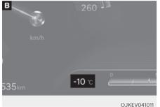
Gauge accuracy for outside air temperature is 1°C (1°F).
