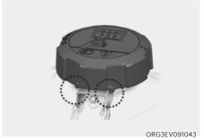
Make sure that the tiny protrusions inside the coolant cap are securely interlocked.
