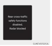
When the rear bumper around the rearside radar or sensor is covered with foreign material, such as snow or rain, or installing a trailer or carrier, it can reduce the detecting performance and temporarily limit or disable Rear Cross-
