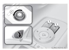
When the gear is shifted to the R (Reverse) position, the outside rearview mirror(s) will rotate downwards to aid with driving in reverse.
