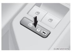
In addition, when the electronic child safety lock button is in the LOCK position and an approaching vehicle from the rear area is detected, the electronic child safety lock button will not unlock even if the driver presses the button to prevent the rear doors from opening.
