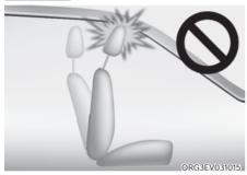
If you recline the seatback towards the front with the headrest and seat cushion raised, the headrest may come in contact with the sunvisor or other parts of the vehicle.
