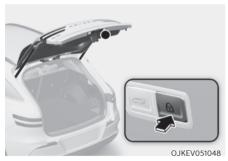
Press the power tailgate lock button while carrying the smart key. The tailgate closes and locks with a warning sound. Additionally, all doors will lock.
