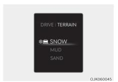
Push (1) the DRIVE/TERRAIN switch to change from Drive mode to Multi terrain mode. After the switch is pushed, push the DRIVE/TERRAIN switch up or down (2) within 4 seconds to select SNOW, MUD or SAND. When the DRIVE/TERRAIN switch is pushed again, the previous Drive mode will be reselected. For more details on Terrain mode, refer to "All Wheel Drive" section in this chapter.
