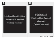
When the front view camera is covered with dirt, snow, or debris, Intelligent Front-Lighting System may temporarily not work properly. If this occurs, the 'Intelligent Front-Lighting System (IFS) disabled. Camera obscured' (or 'IFS (Intelligent Front-Lighting System) disabled. Camera obscured') warning message will appear on the cluster.
