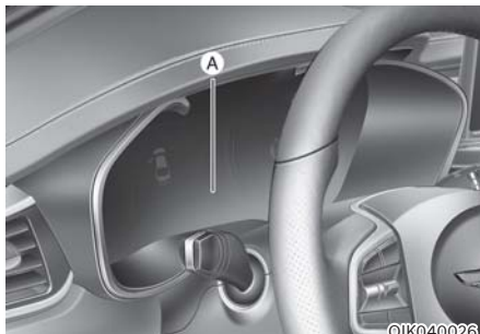
[A] : Interior view camera
