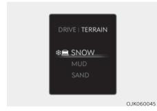
Push (1) the DRIVE/TERRAIN switch to change from Drive mode to Multi terrain mode. After the switch is pushed, push the DRIVE/TERRAIN switch up or down (2) within 4 seconds to select SNOW, MUD or SAND. When the DRIVE/ TERRAIN switch is pushed again, the previous Drive mode will be reselected.
