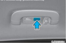
Press the button to turn the lamp on or off.
