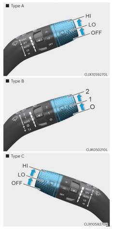
The rear window wiper and washer switch is located at the end of the wiper and washer switch lever. Turn the switch to the desired position to operate the rear wiper and washer.
