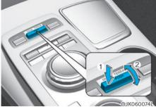
Push (1) the DRIVE/TERRAIN switch to change from normal driving mode to multi terrain mode. Push the switch up or down (2) within 4 seconds to select SNOW, MUD or SAND.
