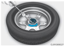
If it is hard to loosen the tire hold-down wing bolt by hand, you can loosen it easily using the wheel lug wrench (1). Turn the tire hold-down wing bolt counterclockwise with the wheel lug wrench.
