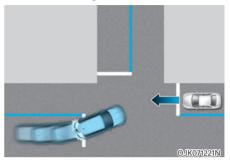
Junction Turning function helps avoid a collision with an oncoming vehicle in an adjacent lane when turning left (lefthand drive) or right (right-hand drive) at a crossroad with the turn signal on by applying emergency braking.
