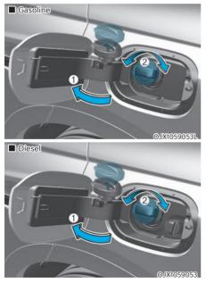
4. Pull the fuel filler door (1) outward to access the fuel tank cap.
