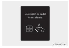
In traffic, your vehicle will stop if the vehicle ahead of you stops. Also, if the vehicle ahead of you starts moving, your vehicle will start as well. In addition, after the vehicle has stopped and a certain time have passed, the 'Use switch or pedal to accelerate' message will appear on the cluster. Depress the accelerator pedal or operate the + switch, - switch or II° switch to start driving.
