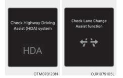
When Highway Driving Assist or Highway Lane Change function is not working properly, the 'Check Highway Driving Assist (HDA) system' or 'Check Lane Change Assist function' warning message will appear, and the A warning light will illuminate on the cluster. We recommend that the vehicle be inspected by an authorized retailer of Genesis Branded products
