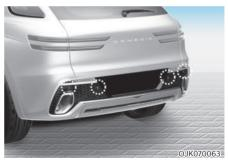
The rear ultrasonic sensors are located inside the rear bumper to detect objects in the rear area. If the sensors are covered with foreign material, such as snow or rain, it may adversely affect sensor performance and Reverse Parking Collision-Avoidance Assist may not operate normally. Always keep the rear bumper clean.
