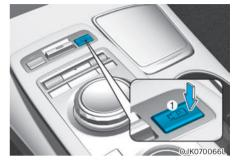
**Parking/View button** Press the Parking/View button (1) to turn on Rear View Monitor.
