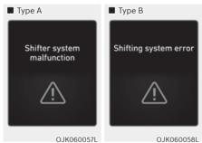
This message is displayed when the transmission or the shift button does not properly operate in the P (Park) position.
