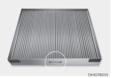
Install a new cabin air filter in the correct direction with the arrow symbol (↓) facing downwards, to prevent noise and reduce effectiveness.
