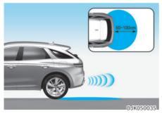
The smart tailgate detecting area extends approximately 50-100 cm (20-40 in.) behind the vehicle. If you are positioned in the detecting area and are carrying the smart key, the hazard warning lights will blink and the chime will sound for about 3 seconds to alert you that the tailgate will open. • The alert stops once the smart key is moved outside of the detecting area within the 3 second period.
