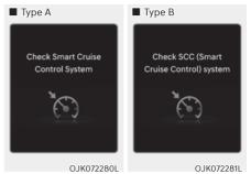
When Smart Cruise Control is not working properly, the 'Check Smart Cruise Control system' (or 'Check SCC (Smart Cruise Control) system') warning message will appear, and the A warning light will illuminate on the cluster. We recommend that the vehicle be inspected by an authorized retailer of Genesis Branded products.
