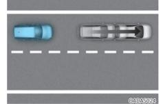
If the vehicle in front abruptly departures, Leading Vehicle Departure Alert may not operate properly. • When a pedestrian or bicycle is between you and the vehicle ahead
