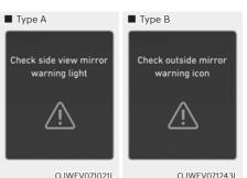
When the outside rearview mirror warning light is not working properly, the 'Check side view mirror warning light' (or 'Check outside mirror warning icon') warning message will appear on the cluster for several seconds, and the master (A) warning light will illuminate on the cluster. If this occurs, we recommend that the vehicle be inspected by an authorized retailer of Genesis Branded products.
