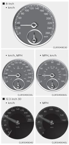
The speedometer indicates the speed of the vehicle and is calibrated in kilometers per hour (km/h) and/or miles per hour (MPH).
