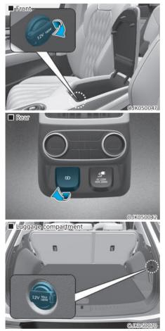
The power outlet is designed to provide power for mobile telephones or other devices designed to operate with vehicle electrical systems. The devices should draw less than 180 watts with the engine running.
