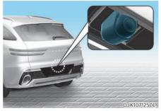
The wide-rear view camera is used as a detecting sensor to detect pedestrians. If the camera lens is covered with foreign material, such as snow or rain, it may adversely affect camera performance and Reverse Parking Collision-Avoidance Assist may not operate normally. Always keep the camera lens clean.
