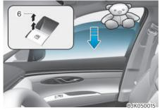
If a window senses any obstacle while it is closing automatically, it will stop and lower approximately 30 cm (12 in.) to allow the object to be cleared.
