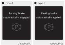
Parking brake automatically engaged / Parking brake automatically applied When EPB is applied while Auto Hold is activated, a warning will sound and a message will appear.
