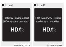
If the driver still does not have their hands on the steering wheel after the hands-off warning, the 'Highway Driving Assist (HDA) canceled' (or 'HDA (Highway Driving Assist) cancelled') warning message will appear and Highway Driving Assist and Lane Change Assist will be automatically canceled.
