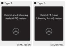
When Lane Following Assist is not working properly, the 'Check Lane Following Assist (LFA) system' (or 'Check LFA (Lane Following Assist) system') warning message will appear on the cluster for several seconds, and the master (A) warning light illuminates on the cluster. If this occurs, we recommend that the vehicle be inspected by an authorized retailer of Genesis Branded products.
