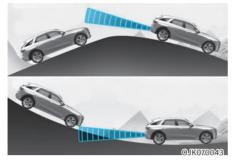
Blind-Spot Collision-Avoidance Assist may not operate properly when driving on a slope. The function may not detect the vehicle in the next lane or may incorrectly detect the ground or structure.
