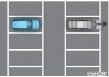
If a vehicle parked in front drives away from you, Leading Vehicle Departure Alert may alert you that the parked vehicle is driving away. • When driving at a tollgate or intersection, etc.
