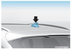
The shark fin antenna will receive AM, FM broadcast signals and transmit data.
