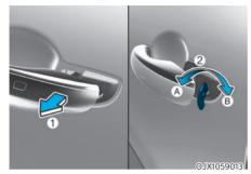
After pulling the door handle (1), turn the key (2) toward the front of the vehicle to lock (A) or turn the key toward the rear of the vehicle to unlock (B).
