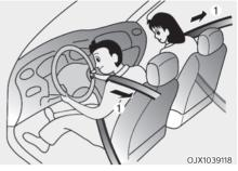
[1] : Retractor pre-tensioner seat belt Front seat and rear outboard seat (if equipped)
