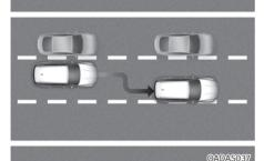
When vehicle speed is above 60 km/h (40 mph), if a vehicle around you is driving at a close distance, your vehicle will control steering in the opposite direction of the vehicle to assist in safe driving.
