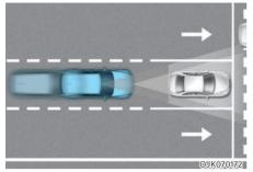
Forward Collision-Avoidance Assist is designed to help detect and monitor the vehicle ahead or help detect a pedestrian or cyclist in the roadway and warn the driver that a collision is imminent with a warning message and an audible warning, and application of emergency braking.
