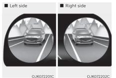
Blind-Spot View Monitor displays the rear blind spot area of the vehicle in the cluster when the turn signal is turned on to help safely change lanes.
