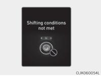
This message is displayed when engine RPM is too high, or when driving speed is too fast to shift the gear.
