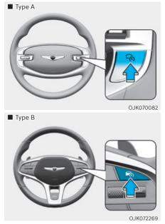
To turn off Smart Cruise Control Press the Driving Assist (5) button to turn Smart Cruise Control off.
