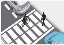
If there is a pedestrian(s) or bicycle(s) in between you and the vehicle in front, Leading Vehicle Departure Alert may not operate properly.
