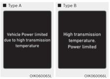
This message is displayed when the transmission oil temperature is high.
