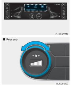
The fan speed can be set to the desired speed by touching the **S** or **S** icon, or by turning the fan speed control knob.
