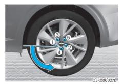
Loosen the wheel bolts counterclockwise one turn each in the order shown above, but do not remove any wheel bolts until the tire has been raised off of the ground.
