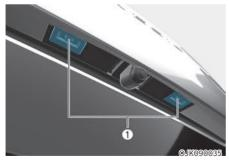
If the LED lamp (1) does not operate, we recommend that the system be inspected by an authorized retailer of Genesis Branded products. The LED lamps cannot be replaced as a single unit because it is an integrated unit. The LED lamps has to be replaced with the unit.
