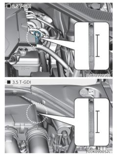
6. Pull the dipstick out again and check the level. The level should be between F (Full) and L (Low).
