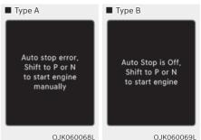
Auto stop error. Shift to P or N to start engine manually / Auto Stop is Off. Shift to P or N to start engine
