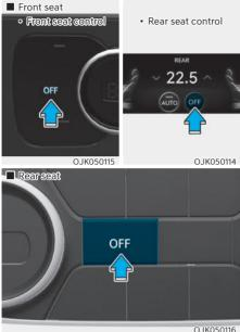
Touch the OFF icon or press the OFF button to turn the climate control system off. You can still operate mode selection and air intake control as long as the Engine Start/Stop button is in the ON position.
