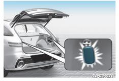
The lamp turns on when the tailgate is opened.
