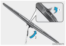
3. Lift up the wiper blade clip (1). Then lift up the wiper blade (2).
