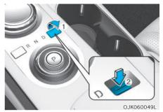
Remove the cap-cover (1) and press the button (2) while depressing the brake pedal.
