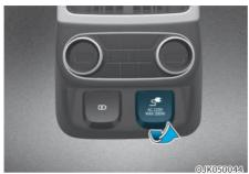
The AC inverter supplies 220 volts/200 watts electric power to operate electric accessories or equipment.
