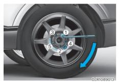
16. Use the wheel lug wrench to tighten the wheel bolts in the order shown. Double-check each wheel bolts until they are tight. After changing tires, we recommend that an authorized retailer of Genesis Branded products tighten the wheel bolts to their proper torque as soon as possible. The wheel bolt should be tightened to 14~16 kgf.m (101~116 lbf.ft).
