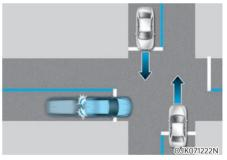
Junction Crossing function helps avoid a collision with oncoming vehicles on the left or right side when crossing an intersection by applying emergency braking.
