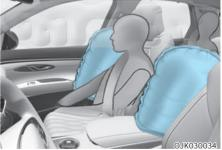
Your vehicle is equipped with a side air bag in each front seat. Additionally, a front center side air bag is provided in the inboard side of the driver seatback. The purpose of the air bag is to provide the vehicle's additional protection than that offered by the seat belt alone. The side air bags and front center side air bag are designed to deploy during certain side impact collisions, depending on the crash severity.
