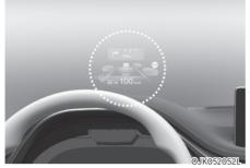
The Head-Up Display is an optional feature that allows the driver to view information projected onto a transparent screen while still keeping your eyes safely on the road ahead while driving.
