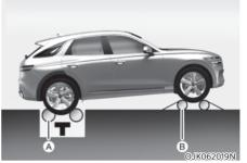
[A]: Roll tester (Speedometer),[B]: Temporary free roller
