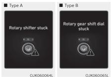
This message is displayed when the shift dial does not return back to it's normal position after rotating it.
