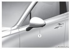
If the LED lamp (1) does not operate, we recommend that the system be inspected by an authorized retailer of Genesis Branded products.
