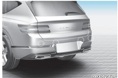
The rear ultrasonic sensors are located inside the rear bumper to detect objects in the rear area. If the sensors are covered with foreign material, such as snow or rain, it may adversely affect sensor performance and Reverse Parking Collision-Avoidance Assist may not operate properly. Always keep the rear bumper clean.
