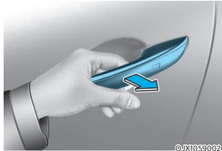
To unlock your vehicle using the door handle touch sensor or the Smart Key:
