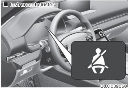
As a reminder to the driver, the seat belt warning light will illuminate for approximately 6 seconds each time the Engine Start/Stop button is in the ON position regardless of belt fastening.
