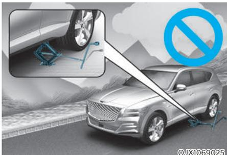
**Never start or run the engine while an AWD vehicle is raised on a jack. The vehicle can slip or roll off of a jack causing serious injury or death to you or those nearby.**
