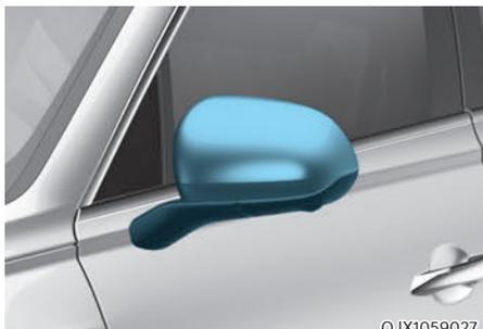
Your vehicle is equipped with both left-hand and right-hand outside rearview mirrors. The mirrors can be adjusted remotely with the mirror adjustment control switch. The outside rearview mirrors can be folded to help prevent damage when going through an automatic car wash or when passing through a narrow street.
