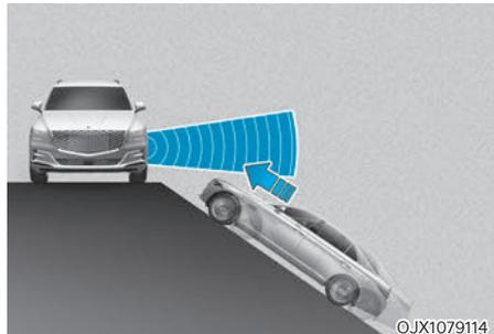
**Rear Cross-Traffic Collision Warning** may be limited when the vehicle is on an uphill or downhill slope, or near it, and may not detect the vehicle approaching from the left or right. If this occurs, the function may not warn the driver when necessary. Always check your surroundings while backing up.
