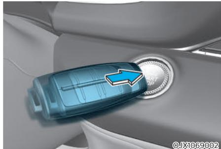
If the smart key battery is weak or the smart key does not work correctly, you can start the vehicle by pressing the Engine Start/Stop button with the smart key in the direction of the picture above.
