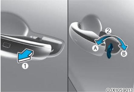
After pulling the door handle (1), turn the key (2) toward the front of the vehicle to lock (A) or turn the key toward the rear of the vehicle to unlock (B).
