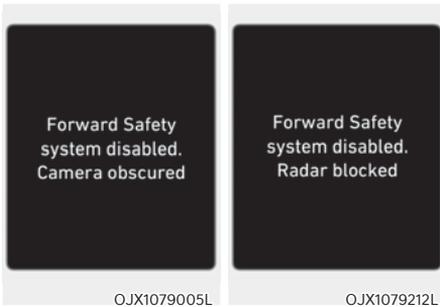
When the front windshield where the front view camera is located, front radar cover, bumper or sensor is covered with foreign material, such as snow or rain, it can reduce the detecting performance and temporarily limit or disable Forward Collision-Avoidance Assist.
