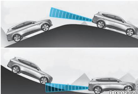
Blind-Spot Collision Warning may not operate properly when driving on a slope. The function may not detect the vehicle in the next lane or may incorrectly detect the ground or structure.
