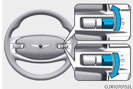
To resume Manual Speed Limit Assist after the function was paused, operate the +, -,
