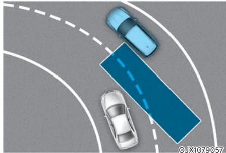
**Blind-Spot Collision Warning may not operate properly when driving on a curved road. The function may not detect the vehicle in the next lane.**
