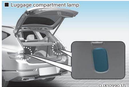
If the LED lamp does not operate, we recommend that the system be inspected by an authorized retailer of Genesis Branded products.
