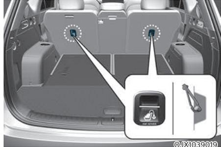
Top-tether anchorages for Child Restraint Systems are located on the rear of the seatbacks.
