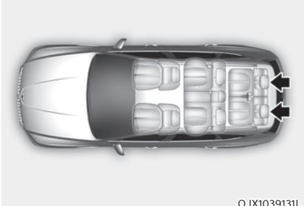
The third row seats are equipped with headrests in all the seating positions for the passenger's safety and comfort.
