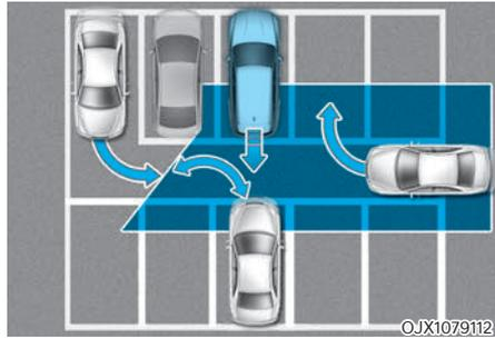
Rear Cross-Traffic Collision-Avoidance Assist may detect vehicles which are parking or pulling out near your vehicle (example, a vehicle leaving beside your vehicle, a vehicle parking or pulling out in the rear area, a vehicle approaching your vehicle making a turn, etc.). If this occurs, the function may unnecessarily warn the driver and control the brake.
