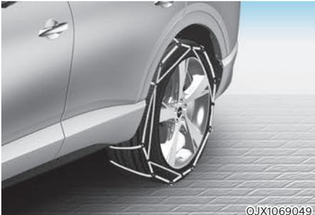
Since the sidewalls of radial tires are thinner than other types of tires, they may be damaged by mounting some types of tire chains on them. Therefore, the use of snow tires is recommended instead of tire chains. If tire chains must be used, use genuine Genesis/Hyundai parts and install the tire chain after reviewing the instructions provided with the tire chains. Damage to your vehicle caused by improper tire chain use is not covered by your vehicle manufacturer's warranty.
