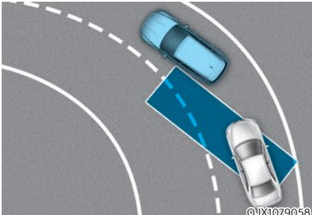
**Blind-Spot Collision-Avoidance Assist** may not operate properly when driving on a curved road. The function may recognize a vehicle in the same lane.
