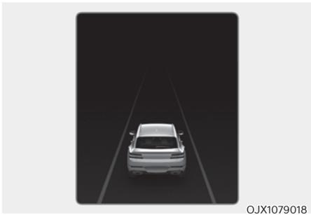
The status of Smart Cruise Control, Lane Following Assist, Highway Driving Assist, etc., is displayed when Driving Assist view mode is selected.
