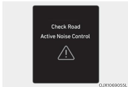
When Road Active Noise Control is not working properly, this warning message will appear on the cluster LCD display. If this occurs, we recommend that the system be inspected by an authorized retailer of Genesis Branded products.
