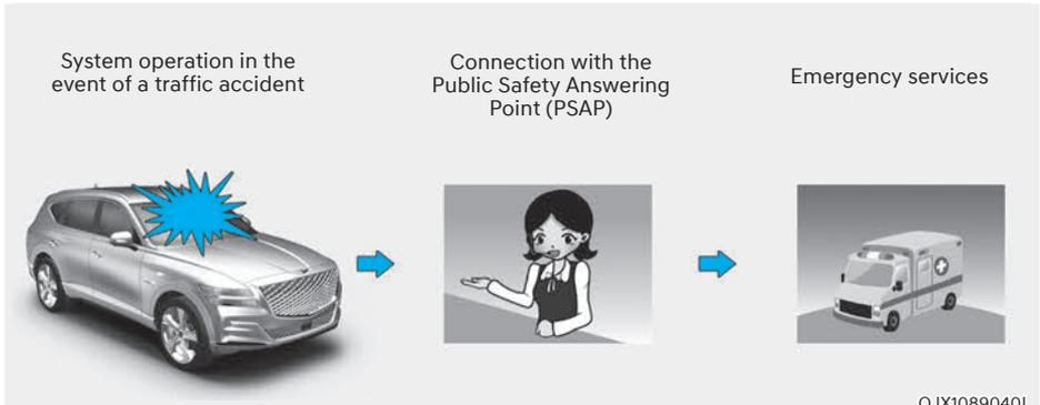
The Pan-European eCall device automatically makes an emergency call to the Public Safety Answering Point (PSAP) for proper rescuing operations in event of vehicle accident.
