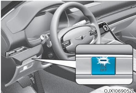
When the system is deactivated, the ISG off button indicator will illuminate and a message 'Auto Stop error. Shift to P or N to start engine manually' appears on the cluster LCD display with a warning sound.
