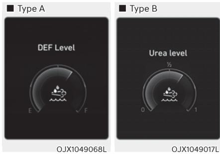
DEF (Diesel Exhaust Fluid) level gauge display shows the approximate amount of remaining urea solution inside the urea solution tank.
