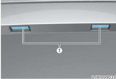
If the LED lamp (1) does not operate, we recommend that the system be inspected by an authorized retailer of Genesis Branded products.
