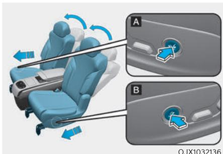
If you push down the back of the onetouch switch more than 0.5 seconds with the premium relax mode activated, the seat will be slightly adjusted to the previous position.
