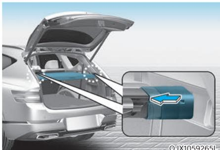
1. Push one side of the cargo screen inward to compress the spring and release the screen from the vehicle.
