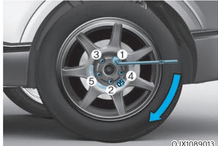
16. Use the wheel lug wrench to tighten the wheel bolts in the order shown. Double-check each wheel bolts until they are tight. After changing tires, we recommend that an authorized retailer of Genesis Branded products tighten the wheel bolts to their proper torque as soon as possible. **The wheel bolt should be tightened to 14~16 kgf.m (101~116 lbf.ft).**
