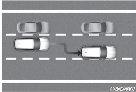
When vehicle speed is above 60 km/h (40 mph), if a vehicle around you is driving at a close distance, your vehicle will control steering in the opposite direction of the vehicle to assist in safe driving.
