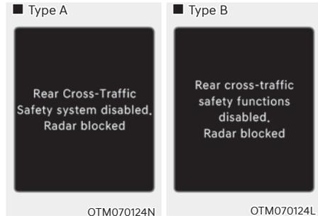
When the rear bumper around the rear corner radar or sensor is covered with foreign material, such as snow or rain, or installing a trailer or carrier, it can reduce the detecting performance and temporarily limit or disable Rear Cross-Traffic Collision Warning.
