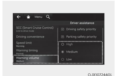
With the vehicle on, select 'Driver Assistance → Warning Volume' from the Settings menu to change the Warning Volume to 'High', 'Medium', 'Low' or 'Off' for Forward/Reverse Parking Distance Warning.
