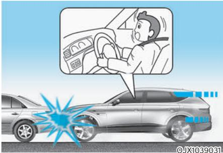
In certain low-speed collisions the air bags may not deploy. The air bags are designed not to deploy in such cases because they may not provide benefits beyond the protection of the seat belts.
