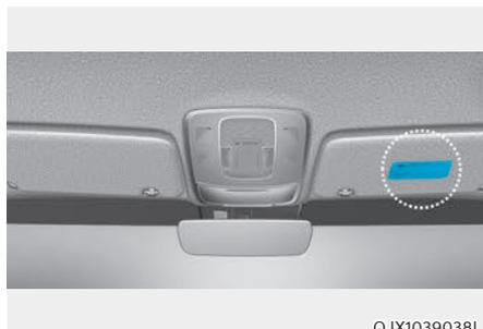
Air bag warning labels are attached to alert the passengers of potential risks of the air bag system.
