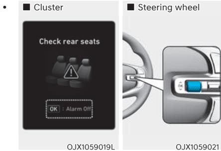
If you do not want to use Rear Occupant Alert, press the OK button on the steering wheel when the first alert is displayed on the cluster. Doing so will deactivate the second alert one time.
