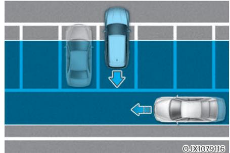
**Rear Cross-Traffic Collision Warning** may detect vehicles passing by behind you when parking backwards into a parking space. If this occurs, the function may unnecessarily warn the driver.
