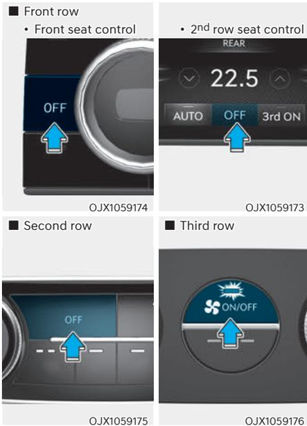
Touch the OFF icon or press the OFF button to turn the climate control system off. You can still operate the mode and air intake buttons as long as the Engine Start/Stop button is in the ON position.
