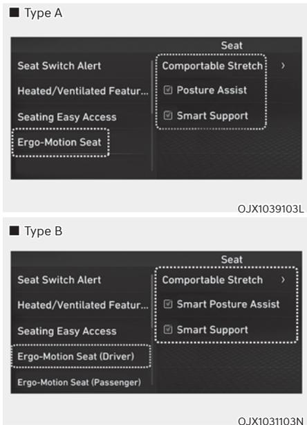
Select 'Ergo-Motion Seat' from the infotainment system's Settings menu to select and set up supplemental functions.
