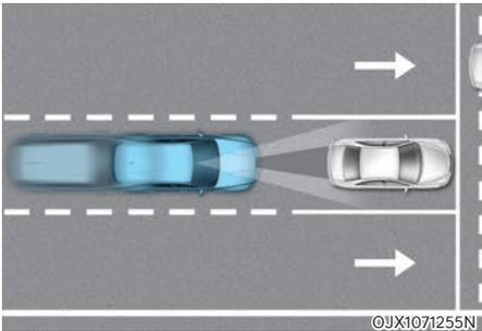
Forward Collision-Avoidance Assist is designed to help detect and monitor the vehicle ahead or help detect a pedestrian or cyclist in the roadway and warn the driver that a collision is imminent with a warning message, an audible warning and application of emergency braking.
