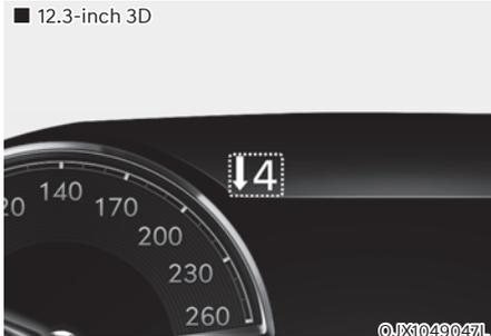
In the Manual Shift mode, this indicator informs which gear is recommended while driving, to save fuel.
