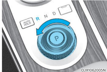
To shift the gear to R (Reverse), rotate the shift dial counterclockwise while depressing the brake pedal.
