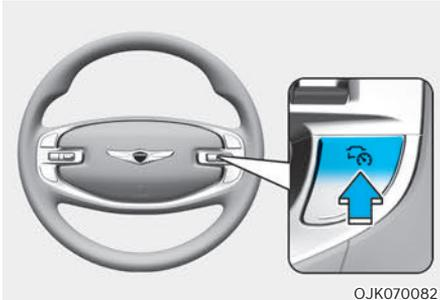
Press the Driving Assist (Ⓜ) button to turn Manual Speed Limit Assist off. The Speed Limit (ⓂLIMIT) indicator will go off.
