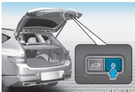
Press the power tailgate lock button while carrying the smart key. The tailgate closes and locks with a warning sound. Additionally, all doors will lock.
