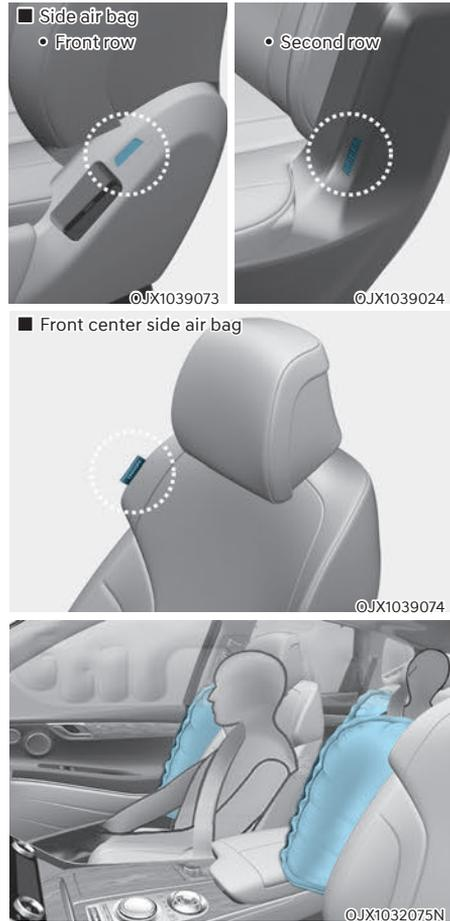
Your vehicle is equipped with a side air bag in each front and outboard second row seat. Additionally, a front center side air bag is provided in the inboard side of the driver seatback. The purpose of the air bag is to provide the vehicle's additional protection than that offered by the seat belt alone.
