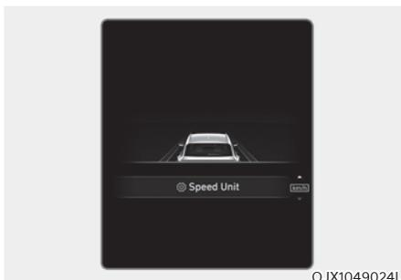
When the Speed Unit menu is selected, press the OK switch on the steering wheel. You can change the speed unit setting between km/h and MPH for the cluster.
