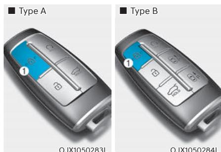
You can still control the window movement with the engine turned off by pressing the Door Lock button (1) for more than 3 seconds. The window moves up, as long as you press the door lock button. The window movement stops, when you release the door lock button. The hazard warning lights blink 3 times, when the window is completely closed.
