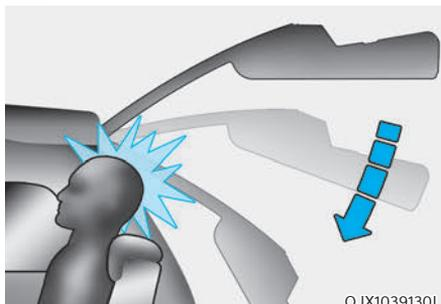
Be careful when closing the tailgate with passenger's seated on the third row seat. If the passenger's head is not properly against a adjusted headrest or a tall person is seated, the tailgate may hit the passenger's head, which could cause injury.
