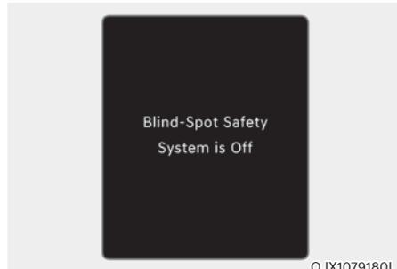
When the engine is restarted with Blind-Spot Collision Warning off, the 'Blind-Spot Safety System is Off' message will appear on the cluster.
