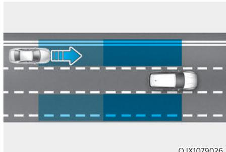
Blind-Spot Collision Warning helps detect and inform the driver that a vehicle is approaching at high speed from the blind spot area.
