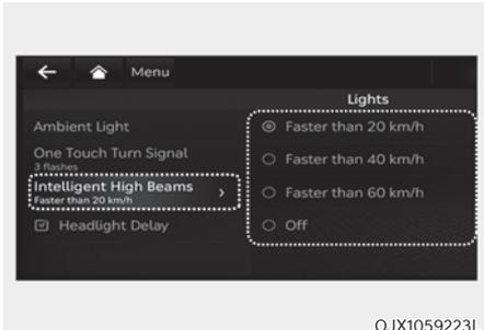
With the Engine Start/Stop button in the ON position, select 'Lights → Intelligent High Beams (or Smart High Beam)' from the Settings menu to turn on Intelligent Front-Lighting System and deselect to turn off the system.
