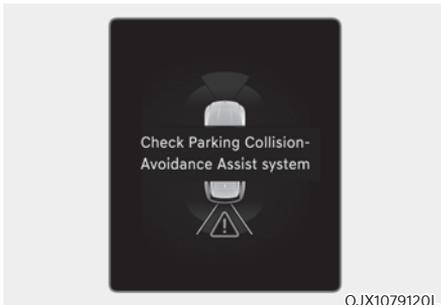
When Reverse Parking Collision-Avoidance Assist or other related functions are not working properly, the 'Check Parking Safety system' warning message will appear on the cluster, and Reverse Parking Collision-Avoidance Assist will turn off automatically. We recommend that the vehicle be inspected by an authorized retailer of Genesis Branded products.
