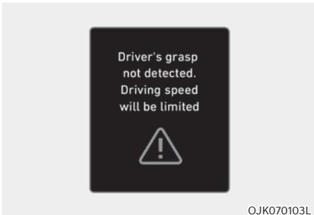
When Highway Driving Assist is cancelled by the hands-off warning, The driving speed will be limited. While Driving Speed Limit function is operating, the 'Driver's grasp not detected. Driving speed will be limited' warning message will appear on the cluster, and an audible warning will sound continuously.
