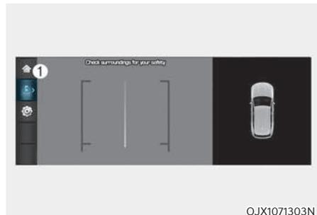
When you touch the icon (1), the top view is displayed on the screen and shows the distance from the vehicle in the back of your vehicle while parking.
