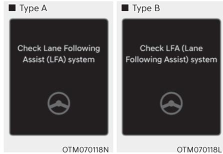
When Lane Following Assist is not working properly, the ‘Check Lane Following Assist (LFA) system’ (or ‘Check LFA (Lane Following Assist) system’) warning message will appear for several seconds, and the master (⚠️) warning light will illuminate on the cluster. If this occurs, we recommend that the vehicle be inspected by an authorized retailer of Genesis Branded products.
