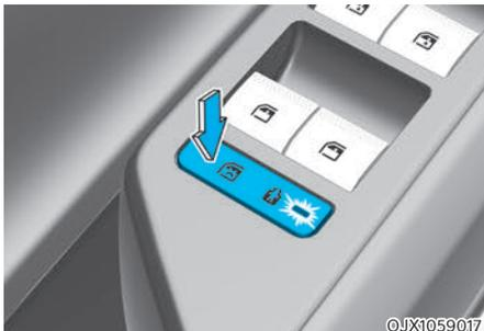
In addition, when the electronic child safety lock button is in the LOCK position and an approaching vehicle from the rear area is detected, the electronic child safety lock button will not unlock even if the driver presses the button to prevent the rear doors from opening.
