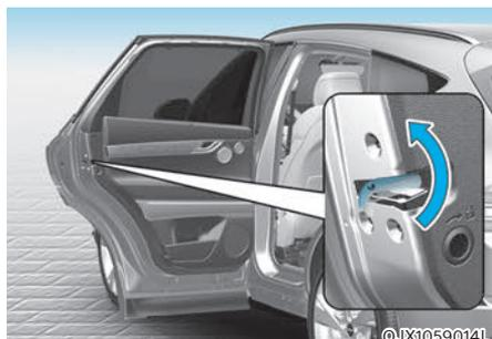
In case of emergency such as when the battery is discharged, the only way to lock the door(s) with the mechanical key from the outside key hole.
