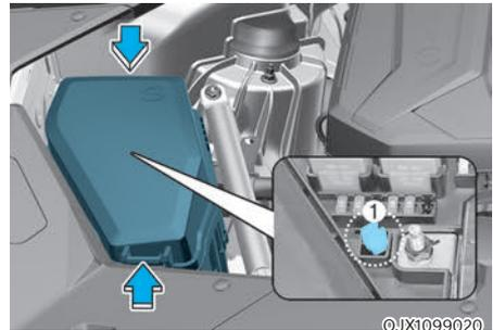
5. Pull the suspected fuse straight out. Use the removal tool (1) provided in the engine compartment fuses panel.
