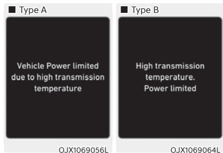
This message is displayed when the transmission oil temperature is high. Drive at steady speed or stop the vehicle at a safe place with the engine on. When the oil temperature returns to normal, the message will disappear.
