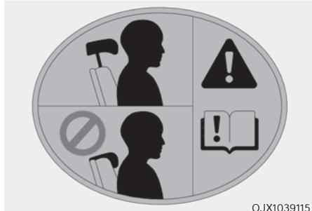
When sitting on the rear seat, do not adjust the height of the headrest to the lowest position.
