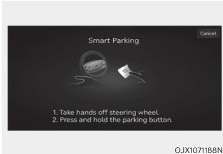
**If Remote Smart Parking Assist cannot activate Remote Smart Parking function, only the Smart Parking guide will be displayed on the infotainment system screen.**
