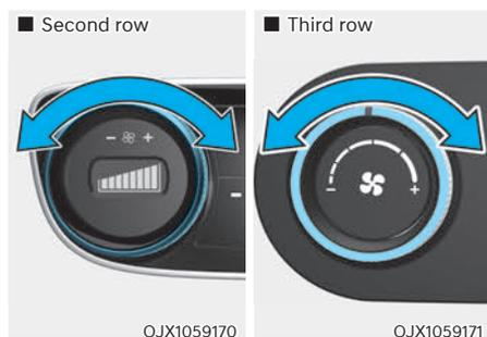
The fan speed can be set to the desired speed by touching the or icon, or by turning the fan speed control knob.
