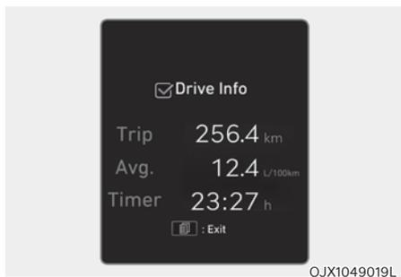
2. Use the  $\wedge$ ,  $\vee$  (UP, DOWN) switch to change items, and press the OK switch to select or deselect the item.
