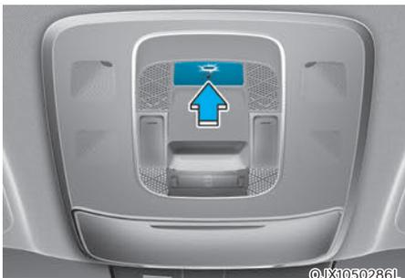
Using the Built-in Cam manual recording button, the driver can record situations before and after the button is pressed.
