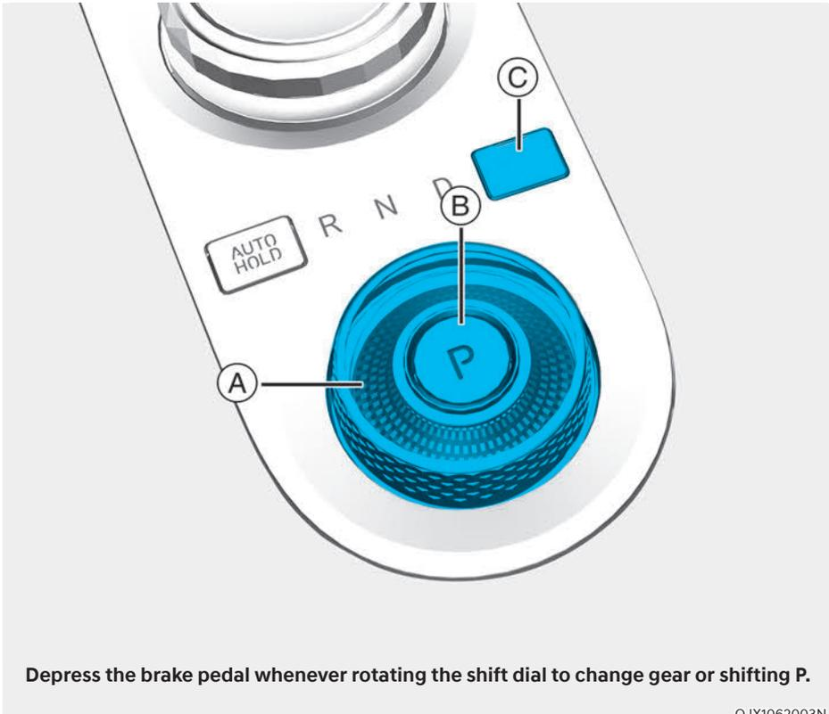
**Depress the brake pedal whenever rotating the shift dial to change gear or shifting P.**
