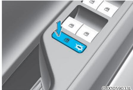
The driver can disable the power window switches on the rear passenger doors by pressing the power window lock button. When the power window lock button is pressed:
