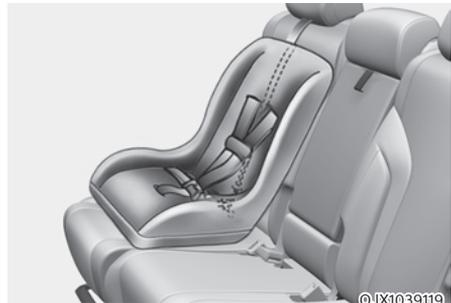
1. Route the Child Restraint System top-tether strap over the seatback. Placing the top tether strap, follow the instructions of the Child Restraint System manufacturer.
