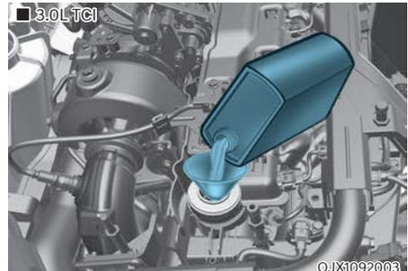
If the level is in the D range, add enough engine oil to bring the level up to the C range.
