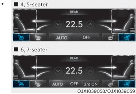
You can also adjust the rear air ventilation seat from the front seats. With the engine running, touch the air ventilation seat icon on the climate control system screen.
