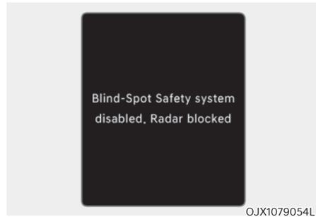
When the rear bumper around the rear corner radar or sensor is covered with foreign material, such as snow or rain, or installing a trailer or carrier, it can reduce the detecting performance and temporarily limit or disable Blind-Spot Collision Warning.
