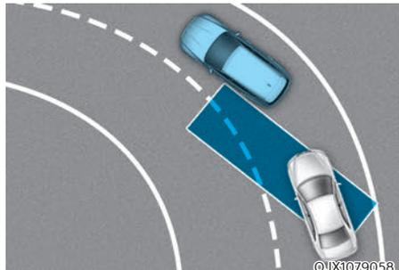
**Blind-Spot Collision Warning may not operate properly when driving on the curved road. The function may recognize the vehicle in the same lane.**
