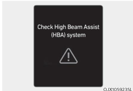
When High Beam Assist is not working properly, the 'Check High Beam Assist (HBA) system' warning message will appear and
