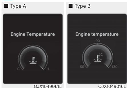
For 8-inch instrument cluster, you can check the engine coolant temperature in the Utility view on the cluster.
