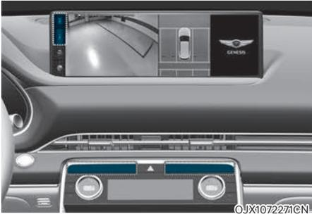
Surround View Monitor will assist in parking by allowing the driver to see around the vehicle.
