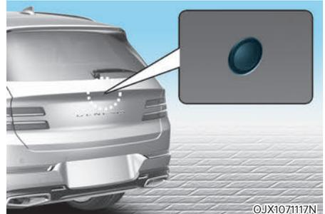
The wide-rear view camera is used as a detecting sensor to detect pedestrians. If the camera lens is covered with foreign material, such as snow or rain, it may adversely affect camera performance and Reverse Parking Collision-Avoidance Assist may not operate properly. Always keep the camera lens clean.
