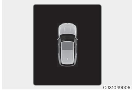
If the driver turns off the engine when the sunroof is not fully closed, the warning chime will sound for several seconds and the sunroof open warning will appear on the cluster LCD display. Close the sunroof securely when leaving your vehicle.
