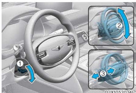
To adjust the steering wheel angle and height:
