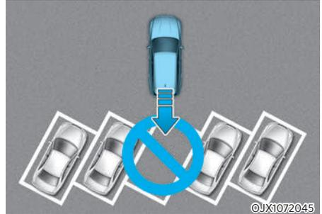
Remote Smart Parking Assist does not provide diagonal parking. Even if your vehicle was able to enter the parking space, do not use Remote Smart Parking Assist because the function cannot operate properly.
