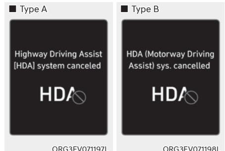
If the driver still does not have their hands on the steering wheel after the hands-off warning, the 'Highway Driving Assist (HDA) cancelled' (or 'HDA (Motorway Driving Assist) cancelled') warning message will appear and Highway Driving Assist and Lane Change Assist will be automatically cancelled.
