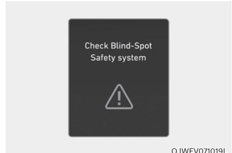
When **Safe Exit Assist** is not working properly, the 'Check Blind-Spot Safety system(s)' warning message will appear on the cluster for several seconds, and the master (⚠) warning light will illuminate on the cluster. If this occurs, we recommend that the vehicle be inspected by an authorized retailer of Genesis Branded products.
