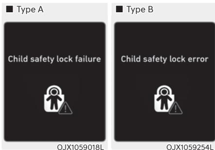
When electronic child safety lock does not work even though the button is pressed, the message will be displayed and an alarm will sound. If this occurs, we recommend that the vehicle be inspected by an authorized retailer of Genesis Branded products.
