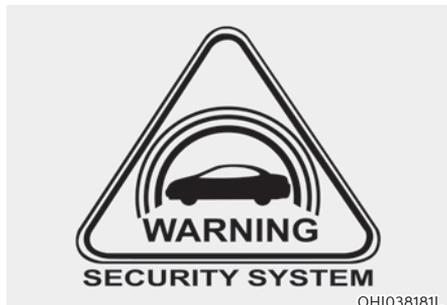
Vehicles equipped with a theft alarm system will have a label attached to the vehicle with the following words:
