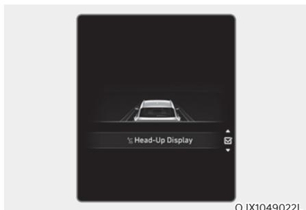
When Head-Up Display menu is selected, press the OK switch on the steering wheel. You can select or deselect head-up display by pressing the OK switch.
