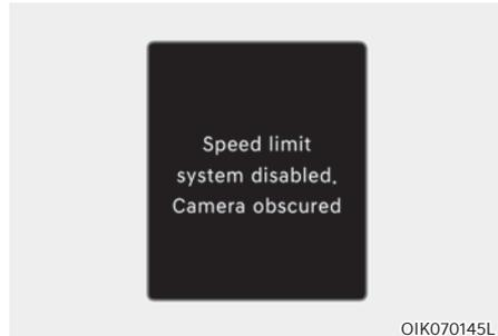
When the front windshield where the front view camera is located is covered with foreign material, such as snow or rain, it can reduce the detecting performance and temporarily limit or disable Intelligent Speed Limit Assist. If this occurs, the 'Speed limit system disabled. Camera obscured' warning message will appear on the cluster.
