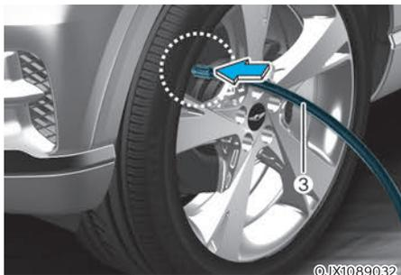
2. Connect the filling hose (3) directly into the tire valve.
