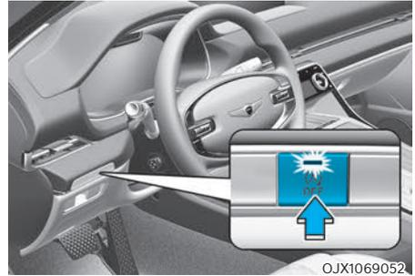
Press the ISG OFF button to turn off ISG system. The ISG OFF button indicator will illuminate. To use the system, press the ISG OFF button again.
