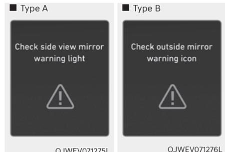
When the outside rearview mirror warning light is not working properly, the 'Check side view mirror warning light' (or 'Check outside mirror warning icon') warning message will appear on the cluster for several seconds, and the master (⚠) warning light will illuminate on the cluster. If this occurs, we recommend that the vehicle be inspected by an authorized retailer of Genesis Branded products.
