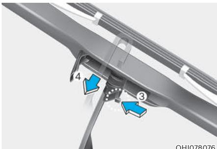
4. While pushing the lock (3), pull down the wiper blade (4).
