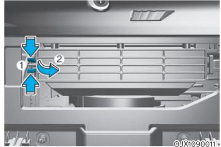
3. Press and hold the lock (1) on the left side of the cover.
