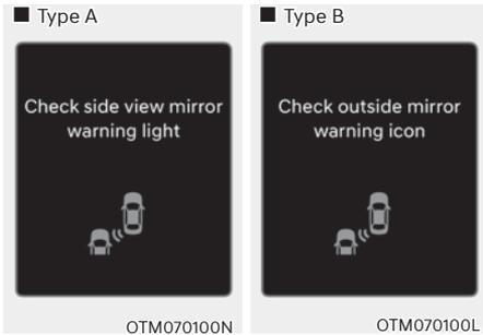
When the outside rearview mirror warning light is not working properly, the 'Check side view mirror warning light' (or 'Check outside mirror warning icon') warning message will appear on the cluster. We recommend that the vehicle be inspected by an authorized retailer of Genesis Branded products.
