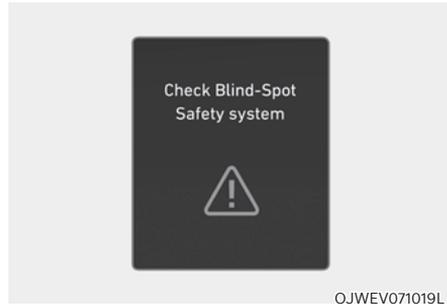
When Safe Exit Warning is not working properly, the 'Check Blind-Spot Safety system(s)' warning message will appear on the cluster for several seconds, and the master (⚠) warning light will illuminate on the cluster. If this occurs, we recommend that the vehicle be inspected by an authorized retailer of Genesis Branded products.
