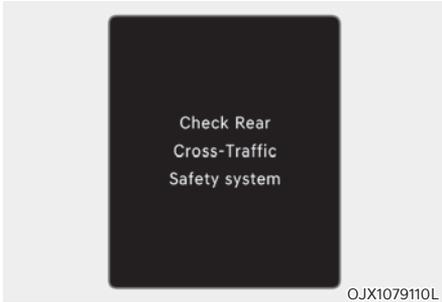
When Rear Cross-Traffic Collision Warning is not working properly, the 'Check Rear Cross-Traffic Safety system' warning message will appear on the cluster, and the function will turn off automatically, or the function will be limited. We recommend that the vehicle be inspected by an authorized retailer of Genesis Branded products.
