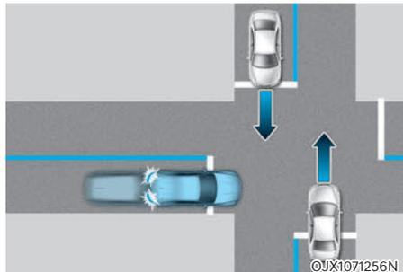
Junction Crossing function can help avoid a collision with oncoming vehicles on the left or right side when crossing an intersection by applying emergency braking.
