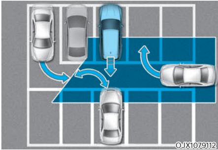
**Rear Cross-Traffic Collision Warning** may detect vehicles which are parking or pulling out near your vehicle (for example: a vehicle leaving beside your vehicle, a vehicle parking or pulling out in the rear area, a vehicle approaching your vehicle making a turn, etc.). If this occurs, the function may unnecessarily warn the driver. Always check your surroundings while backing up.
