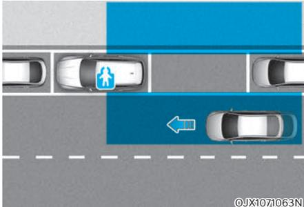
After the vehicle stops, when an approaching vehicle from the rear area is detected after a passenger opens the door, Safe Exit Assist will warn the driver with a warning message and an audible warning to help prevent a collision.
