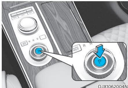
To shift the gear to P (Park), press the P button while depressing the brake pedal. If you turn the engine off in R (Reverse), N (Neutral) or D (Drive), the gear will automatically shift to P (Park).
