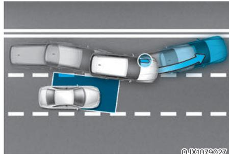
When changing lanes by detecting the lane ahead, if Blind-Spot Collision-Avoidance Assist judges that there is a collision risk with an approaching vehicle in the blind spot, it can help avoid collision by applying the brake.
