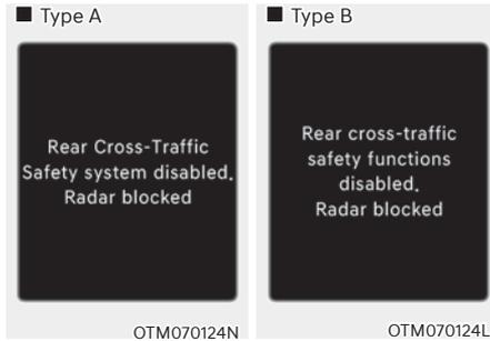
When the rear bumper around the rear-side radar or sensor is covered with foreign material, such as snow or rain, or installing a trailer or carrier, it can reduce the detecting performance and temporarily limit or disable Rear Cross-Traffic Collision-Avoidance Assist.
