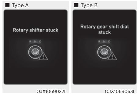
This message is displayed when the shift dial does not return back to its normal position after rotating it.
