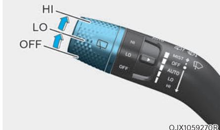
The rear window wiper and washer switch is located at the end of the wiper and washer switch lever. Turn the switch to the desired position to operate the rear wiper and washer.
