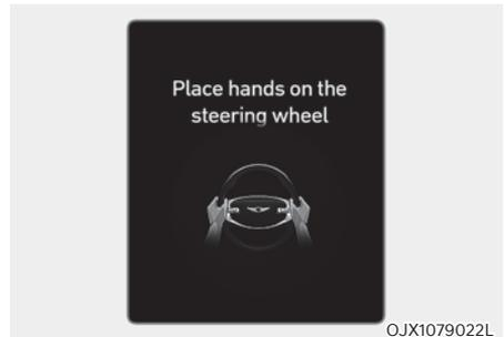
If the driver takes their hands off the steering wheel for several seconds, the 'Keep hands on the steering wheel' warning message will appear and an audible warning will sound in stages.
