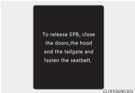
To release EPB, close the doors, hood and tailgate and fasten the seatbelt
