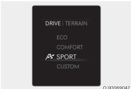
The mode changes whenever the DRIVE/TERRAIN knob is rotated.
