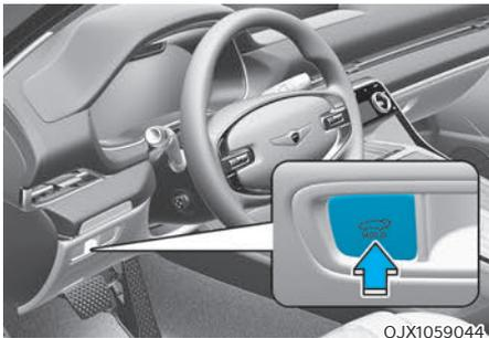
Press the power tailgate open/close button for 1 second. The tailgate opens or closes with a warning sound.
