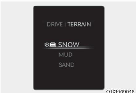
Press the DRIVE/TERRAIN button to change from Drive mode to Multi terrain mode. After the button is pressed, rotate the knob within 4 seconds to select SNOW, MUD or SAND. When the DRIVE/TERRAIN button is pressed again, the previous Drive mode will be reselected.
