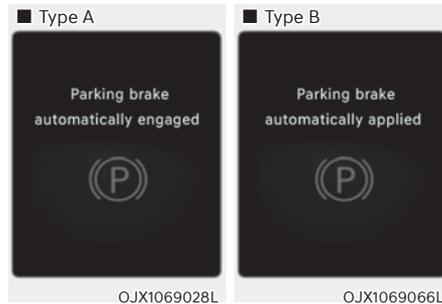
**Parking brake automatically engaged / Parking brake automatically applied**
