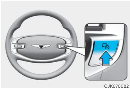
Press the Driving Assist button to turn Cruise Control off. The Cruise (CC) indicator will go off.
