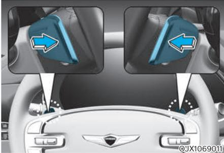
The paddle shifter allows the driver to shift gears without taking one's hands off the steering wheel.
