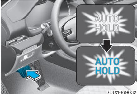
2. When you stop the vehicle completely by depressing the brake pedal, Auto Hold maintains the brake pressure to hold the vehicle stationary. The indicator changes from white to green.
