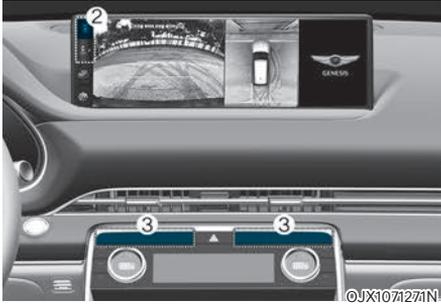
The front image is displayed on the screen when the gear is in N (Neutral) or D (Drive) to assist in parking. The front view has a top view/front view/side view/3D view.
