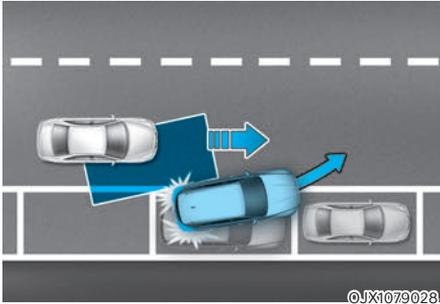
When you are driving forward out of a parking space, if Blind-Spot Collision-Avoidance Assist judges that there is a collision risk with an approaching vehicle in the blind spot, it can help avoid collision by applying the brake.
