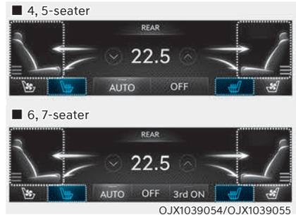
You can also adjust the rear seat warmers from the front seats. With the engine running, touch the seat warmer icon on the climate control system screen.
