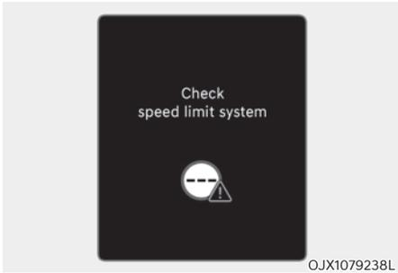
When Intelligent Speed Limit Assist is not working properly, the 'Check speed limit system' warning message will appear on the cluster for several seconds, and the master (⚠) warning light will illuminate on the cluster. If this occurs, we recommend that the vehicle be inspected by an authorized retailer of Genesis Branded products.
