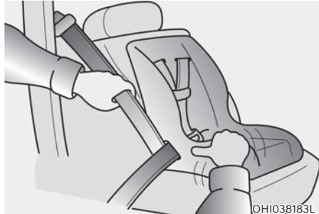
3. Remove as much slack from the belt as possible by pushing down on the Child Restraint System while feeding the shoulder belt back into the retractor.
