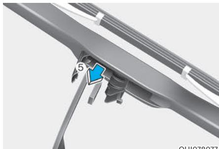
5. Remove the wiper blade from the wiper arm (5).
