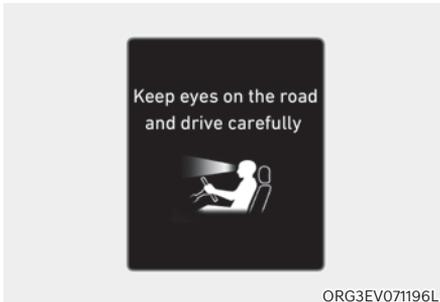
Forward Attention Warning determines whether the driver is focused on the road depending on information, such as the amount of time the driver is looking elsewhere, the amount of time the eyes are closed, how frequently the driver yawns, etc. If Forward Attention Warning judges the driver is not focused, the 'Keep eyes on the road and drive careful' warning message will appear on the cluster, and an audible warning will sound.
