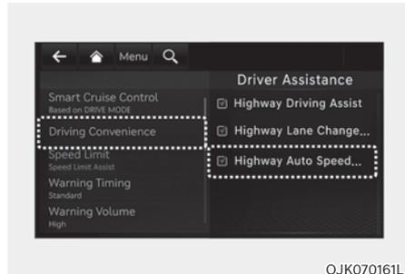
With the vehicle on, select 'Driver Assistance → Driving Assist → Highway Auto Speed Change' from the Settings menu to turn on Navigation-based Smart Cruise Control and deselect to turn off the function.
