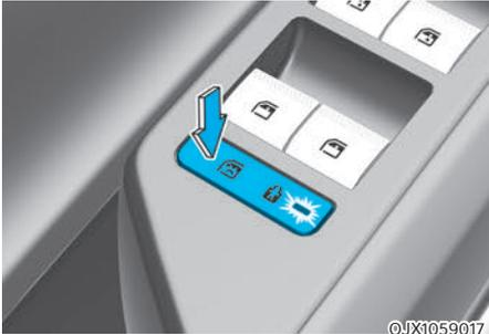
When the electronic child safety lock button is pressed and the indicator light on the button illuminates, the rear doors cannot be opened from inside the vehicle.
