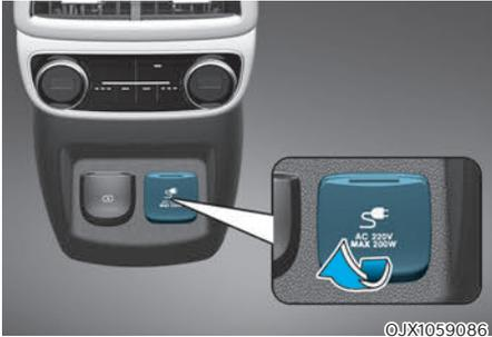
The AC inverter supplies 220 volts/200 watts (or 115 volts/150 watts) electric power to operate electric accessories or equipment.
