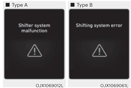
This message is displayed when the transmission or the shift button does not properly operate in the P (Park) position.
