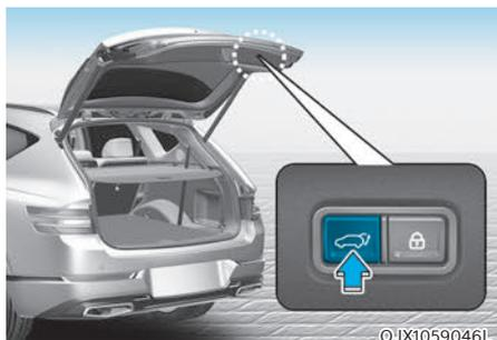
Press the power tailgate open/close button. The tailgate opens or closes with a warning sound.
