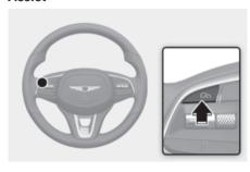
Press the Driving Assist ((2) button to turn Manual Speed Limit Assist off. The Speed Limit (() indicator will go off.
