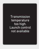
A warning message will pop up on the cluster display if the transmission fluid temperature is above a certain level while using Launch Control. Also, Launch Control will be automatically deactivated.
