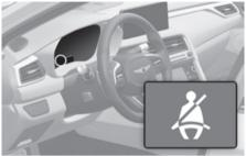
As a reminder to the driver, the seat belt warning light will illuminate for about 6 seconds each time the Engine Start/Stop button is in the ON position regardless of seat belt fastening.
