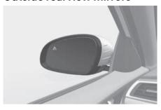
Your vehicle is equipped with both left-hand and right-hand outside rearview mirrors. The mirrors can be adjusted remotely with the remote switch. The outside rearview mirrors can be folded to help prevent damage when going through an automatic car wash or when passing through a narrow street.
