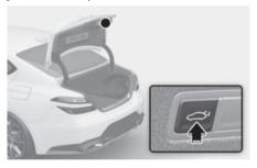
Press the power trunk close button. The trunk will close with a warning sound. While the trunk is closing, press the button to stop power trunk operation.
