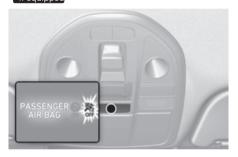
Insert the key or a similar rigid device into the passenger's front airbag ON/OFF switch and turn it to the OFF position. The passenger airbag OFF indicator (※2) will illuminate and stay on until the passenger's front airbag is reactivated.
