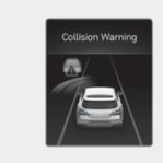
To warn the driver of a collision, the "Collision Warning" warning message appears and the warning light blinks on the cluster with a warning sound and the steering wheel vibrates (if equipped).
