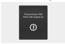
Repeated sudden acceleration and quick start may overheat the transmission. If the transmission is overheated, the self protection mode alarms the driver with an audible sound warning message.
