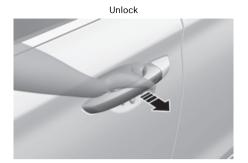
Put your hand in the front outside door handle while carrying the smart key with you or press the Door Unlock button on the smart key, all doors will unlock.
