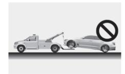
• Do not tow with sling-type equipment. Use wheel lift or flatbed equipment.
