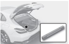
Place the triangle reflector on the road to warn oncoming vehicles during emergencies, such as when the vehicle is parked by the roadside due to problems.
