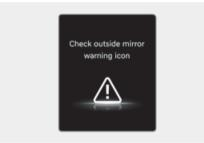
When the outside rearview mirror warning light is not working properly, the "Check side view mirror warning light" (or "Check outside mirror warning icon") warning message will appear on the cluster for several seconds, and the master (△) warning light will illuminate on the cluster. If this occurs, we recommend that the vehicle be inspected by an authorized retailer of Genesis Branded products.
