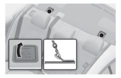
Top-tether anchorages for Child Restraint Systems are located on the package tray.
