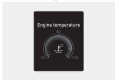
Engine coolant temperature gauge display shows the temperature of the engine coolant when the engine is running.
