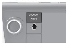
The mode selection, fan speed, air intake and air conditioning will be controlled automatically by the temperature setting you select.
