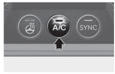
Touch the A/C icon to manually turn the air conditioning on (indicator light will illuminate) and off.
