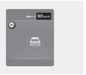
Manual Speed Limit Assist or Smart Cruise Control assists the vehicle to adjust its speed according to the speed limit. When the cruising speed is set as same as the speed limit, the vehicle automatically adjusts its speed if the speed limit changes. The function operates on the road which has a speed limit of 70 km/h (44 mph) or higher. When the function is active, the cruising speed on the instrument cluster appears in green.
