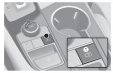
Press the Parking/View button (1) to turn on Rear View Monitor.
