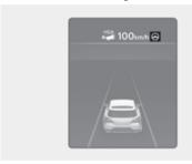
If the vehicle ahead and/or both lane markings are detected and your vehicle speed is below 200 km/h (120 mph), the green indicator light illuminates on the cluster, and Lane Following Assist helps center the vehicle in the lane by assisting the steering wheel.
