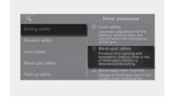
With the engine on, select **Setup** (**Settings**) > **Vehicle** > **Driver assistance** > **Driving safety** > **Blind-spot safety** in the infotainment system to set whether to use each function.
