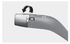
The position light, license plate lamp and instrument panel lamp are turned ON.
