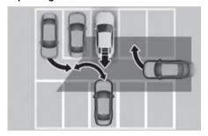
Rear Cross-Traffic Collision-Avoidance Assist may detect vehicles which are parking or pulling out near your vehicle (example, a vehicle leaving beside your vehicle, a vehicle parking or pulling out in the rear area, a vehicle approaching your vehicle making a turn, etc.). If this occurs, the function may unnecessarily warn the driver and control the brake.
