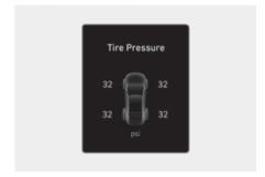
The tire pressure of each tire appears. For more information, refer to the "Tire Pressure Monitoring System (TPMS)" section in chapter 8.
