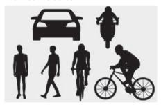
The illustration above shows the image the front view camera and front radar are capable of detecting as a vehicle, powered two-wheeler, and pedestrian and cyclist.
