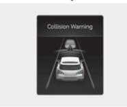
To warn the driver of a collision, the "Collision Warning" warning message appears, and the warning light blinks on the instrument cluster with a warning sound and the steering wheel vibrates (if equipped).
