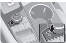
Press the ISG OFF button to turn off ISG system. The ISG OFF button indicator will illuminate. To use the system, press the ISG OFF button again.
