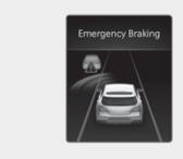
To warn the driver that emergency braking will be assisted, the "Emergency Braking" warning message appears and the warning light blinks on the cluster with a warning sound and the steering wheel vibrates (if equipped).
