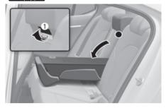
Additional cargo space is provided to accommodate long/narrow cargo (skis, poles, etc.) not able to fit properly in the tailgate when closed.
