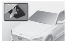
Auto defogging helps reduce the possibility of fogging up the inside of the windshield by automatically sensing the moisture on inside the windshield.
