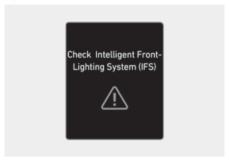
When Intelligent Front-Lighting System is not working properly, the "Check Intelligent Front-Lighting System (IFS)" warning message will come on for a few second on the cluster. After the message disappears, the AFS and \( \frac{1}{2} \) will illuminate on the cluster. We recommend that the system be inspected by an authorized retailer of Genesis Branded products.
