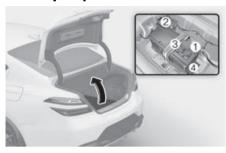
When replacing the battery, disconnect the negative (-) cable (1) and remove the positive (+) battery fuse box (2). Remove the trunk (or tailgate) panel and spare wheel. Place the spare wheel on the floor with the finished side up so as not to damage. Then remove the spare wheel bracket (3) followed by the battery hold down mounting bracket (4).
