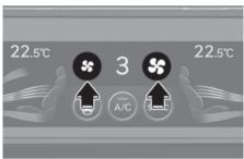
Touch the icon button to increase fan speed and airflow. Touch the left icon to decrease fan speed and airflow.
