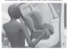
4. Push and pull on the Child Restraint System to confirm that the seat belt is holding it firmly in place.
