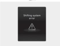
This message appears when the transmission or the shift button does not properly operate in the P (Park) position. We recommend that you have the vehicle inspected by an authorized retailer of Genesis Branded products.
