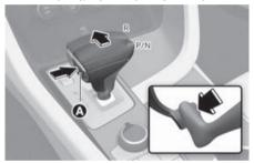
To move the shift lever to R (Reverse), press the **UNLOCK** button [A] while depressing the brake pedal and then move the shift lever forward.
