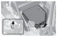
5. Push in a new fuse of the same rating, and make sure it fits tightly in the clips. If it does not fit tightly, we recommend that you consult an authorized retailer of Genesis Branded products.
