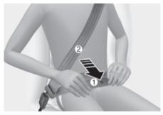
The seat belt automatically adjusts to the proper length after the lap belt portion is adjusted manually so that it fits snugly around your hips. If you lean forward in a slow, easy motion, the belt will extend and move with you.
