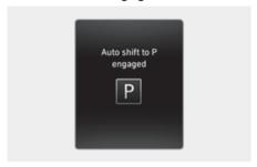
The message appears on the cluster display when the gear shifts to P (Park) automatically.
