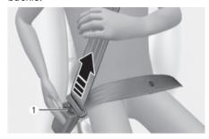
When it is released, the belt should automatically draw back into the retractor. If this does not happen, check the belt to be sure it is not twisted, then try again.
