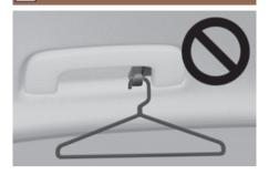
Do not hang other objects such as hangers or hard objects except clothes. Also, do not put heavy, sharp or breakable objects in the clothes pockets. In an accident or when the curtain airbag is inflated, it may cause vehicle damage or personal injury.
