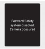
When the front windshield where the front view camera is located, or sensor is covered with foreign material, such as snow or rain, it can reduce the detecting performance and temporarily limit or disable Lane Keeping Assist.
