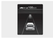
The status of Manual Speed Limit Assist, Smart Cruise Control, Lane Following Assist, Highway Driving Assist, etc. appears when Driving Assist view is selected.
