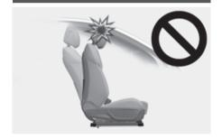
If you recline the seatback towards the front with the headrest and seat cushion raised, the headrest may come in contact with the sunvisor or other parts of the vehicle.
