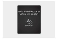
The SCR ( ) warning light and "Refill urea in 000 km or vehicle will not start/Refill urea in 000 km. Otherwise vehicle will not start" warning message appears on the instrument cluster when urea solution tank is nearly empty. Refill immediately.
