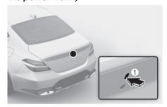
When the trunk is closed, press the power trunk open button to open the trunk.
