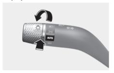
After selecting **Intelligent front-lighting** in the Settings menu, Intelligent Front-Lighting System will operate by following the procedure below.
