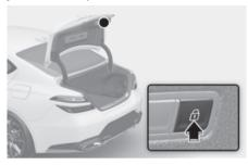
Press the power trunk lock button while carrying the smart key. The power trunk will close and lock with a warning sound. Additionally, all doors will lock.
