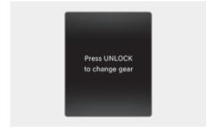
The message appears on the cluster display when the **UNLOCK** button is not pressed while shifting the gear.
