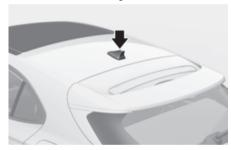
The shark fin antenna will receive AM, FM broadcast signals and transmit data.
