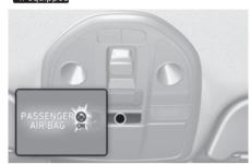
Insert the key or a similar rigid device into the passenger's front airbag ON/OFF switch and turn it to the ON position. The passenger airbag ON indicator (③) will illuminate and go off after about 60 seconds.
