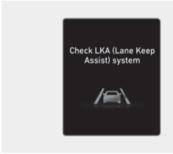
When Lane Keeping Assist is not working properly, the "Check Lane Keeping Assist (LKA) system" (or "Check LKA (Lane Keeping Assist) system") warning message will appear and the yellow indicator light will illuminate on the cluster. If this occurs, we recommend that the vehicle be inspected by an authorized retailer of Genesis Branded products.
