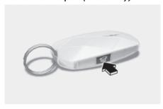
When the trunk is closed, press the power trunk open button for 1 second. The trunk will open with a warning sound.
