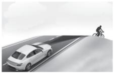
Forward Collision-Avoidance Assist may not detect a vehicle, a powered two-wheeler, and a pedestrian or a cyclist in front of you while driving uphill or downhill, adversely affecting the performance of the sensors.
