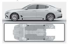
Insert the jack handle into the jack and turn it clockwise, raising the vehicle until the tire clears the ground. Make sure the vehicle is stable on the jack.
