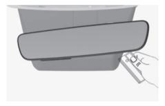
3. While the HomeLink indicator light (5) is flashing orange, press and hold the handheld remote button. Continue pressing the handheld remote button until the HomeLink indicator light (5) light changes from orange to green. You may now release the handheld remote button.
