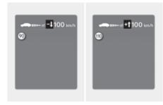
If the speed limit of the road changes during the operation of Manual Speed Limit Assist or Smart Cruise Control, an arrow in the direction of up or down apears to inform the driver that the set speed needs to be changed. At this time, the driver can change the set speed according to the speed limit by using the + or - switch on the steering wheel.
