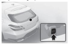
When the tailgate is closed, press the power tailgate open/close button to open the tailgate.
