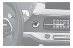
Whenever the front door is opened, the Engine Start/Stop button will illuminate and will go off 30 seconds after the door is closed.
