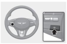
With the engine on, shortly press the Lane Driving Assist (/@\) button located on the steering wheel to turn on Lane Following Assist. The grey or green and indicator light will appear on the instrument cluster.
