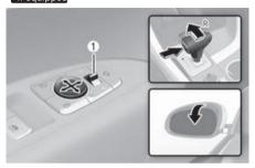
When the gear is shifted to the R (Reverse) position, the outside rearview mirror(s) will rotate downwards to aid with driving in reverse.
