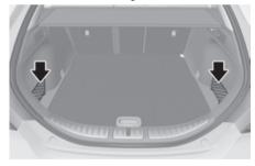
To keep items from shifting in the cargo area, you can use the 4 holders located in the luggage board to attach the luggage net.
