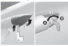
In order to operate door lock by using mechanical key, turn the key after removing the cover.
