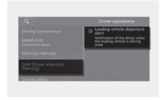
With the engine on, select or deselect Setup (Settings) > Vehicle > Driver assistance > DAW (Driver Attention Warning) from the Settings menu to set whether to use each function.
