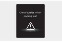
When the outside rearview mirror warning light is not working properly, the "Check side view mirror warning light" (or "Check outside mirror warning icon") warning message will appear on the cluster for several seconds, and the master (A) warning light will illuminate on the cluster. If this occurs, we recommend that the vehicle be inspected by an authorized retailer of Genesis Branded products.
