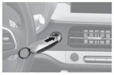
If the smart key battery is weak or the smart key does not work correctly, you can start the engine by pressing the Engine Start/Stop button with the smart key in the direction of the illustration above.
