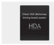
When Highway Driving Assist or Highway Lane Change function is not working properly, the "Check Highway Driving Assist (HDA) system" or "Check HDA (Motorway Driving Assist)"warning
