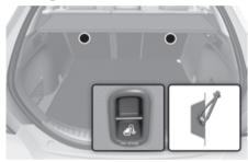
Top-tether anchorages for Child Restraint System are located on the back of the rear seatbacks.
