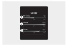
This mode displays information related to your engine such as engine oil temperature(1), current torque(2) and turbo boost pressure(3).
