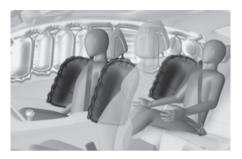
Your vehicle is equipped with a side airbag in each front and outboard second row seat. Additionally, a front center side airbag is provided in the inboard side of the driver seatback. The purpose of the airbag is to provide the vehicle's additional protection than that offered by the seat belt alone.
