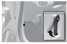
3. Go to the front of the vehicle, raise the hood slightly, push up the secondary latch (1) inside of the hood center and lift the hood (2).
