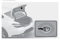
Your vehicle is equipped with an Emergency Trunk Safety Release lever located inside the vehicle. When someone is inadvertently locked in the trunk, the trunk can be opened by moving the lever in the direction of the arrow and pushing the trunk open.
