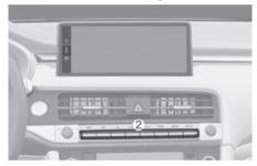
The driver is able to check the rear view on the screen while driving, it is to assist with backing up.
