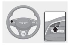
Press the Driving Assist button to turn Cruise Control off. The Cruise (CORUSE) indicator will go off.
