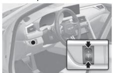
When the vehicle's position lights or headlights are on, press the illumination control switch to adjust the brightness of the instrument panel illumination.
