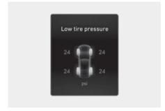
This warning message appears if the tire pressure is low. The corresponding tire on the vehicle will be illuminated.
