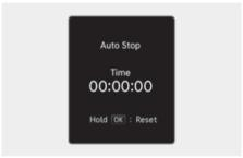
AUTO STOP display shows the elapsed time of engine stop by Idle Stop and Go system.
