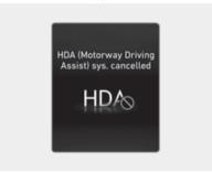
If the driver still does not have their hands on the steering wheel after the hands-off warning, "Highway Driving Assist (HDA) system canceled" or HDA (Motorway Driving Assist) sys. cancelled warning message will appear and Highway Driving Assist and Lane Change Assist will be automatically canceled.
