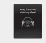
If the driver takes their hands off the steering wheel for several seconds, the "Keep hands on steering wheel or Place hands on the steering wheel" warning message will appear and an audible warning will sound in stages.
