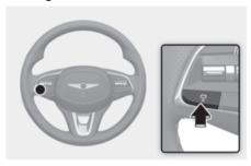
Press the button repeatedly to cycle through the headway settings from Distance  $4 \rightarrow$  Distance  $3 \rightarrow$  Distance  $2 \rightarrow$  Distance  $1 \rightarrow$  Distance 4.
