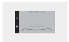
If Rear view reference lines (Rear View Parking Lines) is selected, the rear view parking guide lines and rear top view guide lines appear on the Rear View Monitor screen.
