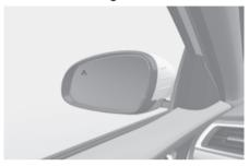
To warn the driver a vehicle is detected, the warning light on the outside rearview mirror illuminates.
