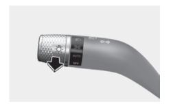
To flash the high beam headlight, pull the lever towards you, then release the lever. The high beams will remain ON as long as you hold the lever towards you.
