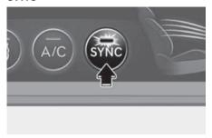
Adjusting the driver and passenger side temperature equally
