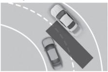
Blind-Spot Collision-Avoidance Assist may not operate properly when driving on a curved road. The function may not detect the vehicle in the next lane.
