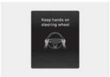
If the driver takes their hands off the steering wheel for several seconds, the "Place hands on the steering wheel" (or "Keep hands on steering wheel") warning message will appear and an audible warning will sound in stages.
