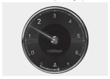
The tachometer indicates the approximate number of engine revolutions per minute (rpm).
