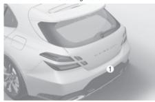
(1) Wide-rear view camera Refer to the illustration above for the detailed location of the detecting sensor.
