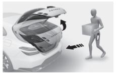
On a vehicle equipped with a smart key, the trunk (or tailgate) can be opened with hands-free activation using the smart trunk (or tailgate) system.
