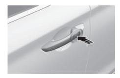
4. Make sure the doors are locked by pulling the door handle.
