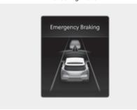
To warn the driver that emergency braking will be assisted, the "Emergency Braking" warning message appears and the warning light blinks on the cluster with a warning sound and the steering wheel vibrates (if equipped).
