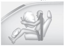
A fully inflated airbag, in combination with a properly worn seat belt, slows the driver's or the front passenger's forward motion, reducing the risk of head and chest injury.
