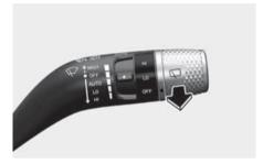
In the OFF (O) position, pull the lever gently toward you to spray washer fluid on the windshield and to run the wipers 1-3 cycles. The spray and wiper operation will continue until you release the lever. If the washer does not work, you may need to add washer fluid to the washer fluid reservoir.
