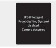
When the front view camera is covered with dirt, snow, or debris, Intelligent Front-Lighting System may temporarily not work properly. If this occurs, a warning message will appear on the instrument cluster.
