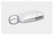
Press the Door Lock button (1) for more than 3 seconds. The window moves up, as long as you press the door lock button. The window movement stops, when you release the door lock button.  Press the Door Unlock button (2) for more than 3 seconds. The window moves down after the doors are unlocked, as long as you press the door unlock button. The window movement stops, when you release the door unlock button.
