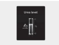
DEF (Diesel Exhaust Fluid) level gauge display shows the approximate amount of remaining urea solution inside the urea solution tank.
