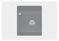
When driving at a speed higher than the displayed speed limit, the red speed limit indicator will blink and warning sounds.
