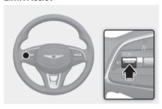
Press the IIO switch to temporarily pause the set speed limit. The set speed limit will turn off but the Speed Limit (SLMIT) indicator will stay on.
