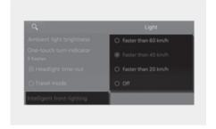
With the Engine Start/Stop button in the ON position, select **Setup (Settings)** > **Vehicle** > **Light** > **Intelligent front-lighting** from the Settings menu to turn on Intelligent Front-Lighting System and deselect to turn off the system.
