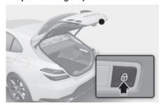
Press the power tailgate lock button whilst carrying the smart key. The tailgate closes and locks automatically. Additionally, all doors will lock.
