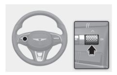
To change the trip mode, toggle the "^, witch on the steering wheel.
