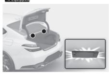
The trunk lamp comes on when the trunk is opened.
