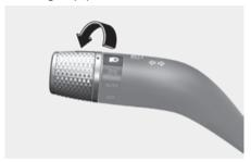
The headlight, position light, license plate lamp and instrument panel lamp are turned ON.
