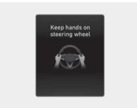
If the driver takes their hands off the steering wheel for several seconds, the "Place hands on the steering wheel" (or "Keep hands on the steering wheel") warning message appears on the cluster, and an audible warning sounds in stages.
