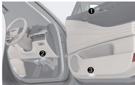
Inner door handle lamp (1) / Foot lamp (2) / Door courtesy lamp (Bulb type) (3)
