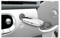
Press the Start/Stop button with the smart key to start the vehicle.
