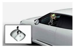
If a window senses any obstacle whilst it is closing automatically, it stops and lowers about 12 in. (30 cm) to allow the object to be cleared.
