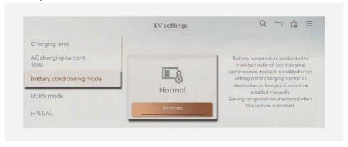
On the Home screen of the infotainment system, select **Electric vehicle** > ③ (EV settings) > **Battery conditioning mode** and select **Activate** to use manually.
