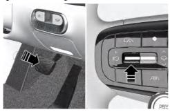
If the Smart Cruise Control feature has been temporarily turned off, it can be turned on again using one of the following methods:
