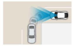
When a vehicle in front of you merges out of the lane, SCC may not immediately detect the new vehicle that is now in front of you. Always pay attention to road and driving conditions whilst driving.
