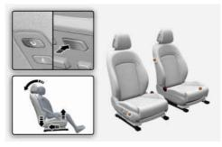
Press and hold the rear portion of the Relaxation mode switch with the Start/Stop button in the POWER ON or DRIVE READY position.
