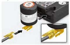
3 Unscrew the valve cap from the valve of the defective wheel and screw the filling hose of the sealant bottle onto the tyre valve.
