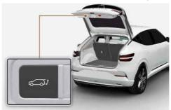
Press the power tailgate open/close button whilst carrying the smart key or digital key. The power tailgate opens or closes with a warning sound.
