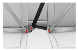
Insert the tongue plate into the buckle until an audible "click" is heard, indicating the latch is locked. Pull the shoulder portion of the belt to snug the belt across your hips and remove slack. Make sure the seat belt is not twisted.
