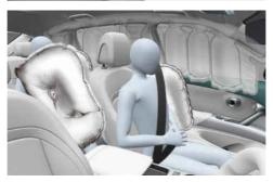
Side airbags are located in each front and outboard second row seat. Additionally, a front centre side airbag is located in the inboard side of the driver seatback.
