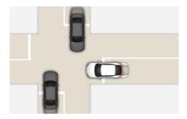
When crossing an intersection, Junction Crossing function helps avoid a collision with an oncoming vehicle on the left or right side by warning or applying emergency braking.
