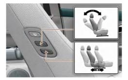
Passengers may use the switches to control the front passenger seat.
