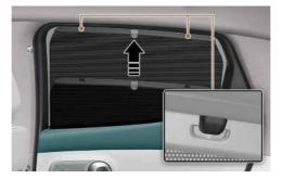
Use the rear side sunshade to block the light coming through the rear seat windows. Lift the rear side sunshade and hang the sunshade on both sides of the hook.
