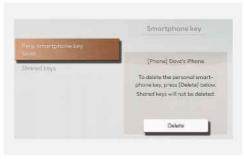
To delete only my registered digital key (smartphone), select **Setup** > **Vehicle** > **Digital key** > **Smartphone key** > **Pers. smartphone key** > **Delete** from the infotainment system.
