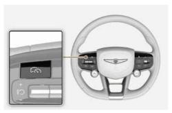
HDA operates when driving on the main road of highways, and turning on/off HDA by pressing the Driving Assist conduction.
