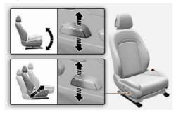
Push the front or rear portion of the control switch up or down to control the seat cushion angle or height.
