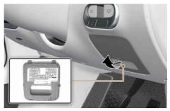
3 Pull the suspected fuse straight out. Use the removal tool provided in the motor compartment fuses panel.
