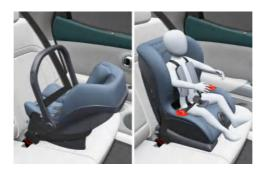
When not using the ISOFIX system, all Child Restraint Systems must be secured to a rear seat using the lap/shoulder belt.
