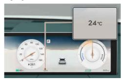
The outside ambient temperature appears in the lower portion of the cluster display. The temperature reads in Fahrenheit or Celsius depending on the units selected from the Settings menu in the infotainment system.
