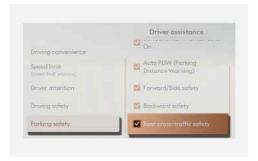
With the vehicle on, select or deselect **Setup** > **Vehicle** > **Driver assistance** > **Parking safety** from the Settings menu to set whether to use each function.
