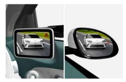
SEW warns the driver with a warning message and an audible warning. The warning light on the outside rearview mirrors (or digital side mirrors) also blinks to warn you.
