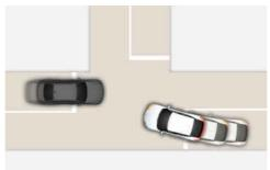
When turning right at a crossroad with the turn signal on, Junction Turning function helps avoid a collision with an oncoming vehicle or motorcyclist in an adjacent lane by warning or applying emergency braking.
