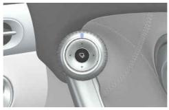
To fold or unfold the DSM cameras, press the DSM camera folding button.
