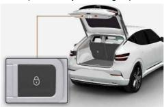
Press the power tailgate lock button whilst carrying the smart key or digital key. The power tailgate closes and locks automatically. Additionally, all doors will lock.
