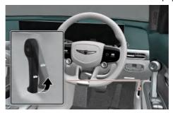
3 Go to the front of the vehicle, raise the bonnet slightly, push up the secondary bonnet release lever inside of the bonnet centre and lift the bonnet.
