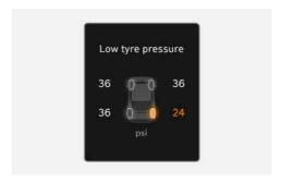
This warning message appears if the tyre pressure is low. The corresponding tyre on the vehicle is illuminated.
