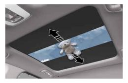
If the power sunshade senses any obstacle whilst it is closing automatically, it will reverse direction then stop at a certain position.
