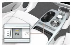
Press and hold the Parking Safety P button to turn the PCA on or off.
