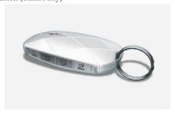
When using Remote Parking function, parking is supported whilst the 🖟 or 🖟 button is pressed, regardless of the button direction. When using the Remote Operation function, the vehicle moves in the direction of the 🖟 or 🖟 button whilst the button is pressed.
