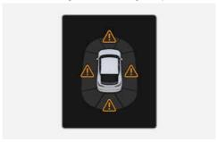
· When the Rear Cross-Traffic Collision-Avoidance Assist, Parking Distance Warning, and Reverse Parking Collision-Avoidance Assist is operating, if the function is not operating properly or the ultrasonic sensor is obscured, the A warning light may illuminate in the direction of the corresponding sensor.
