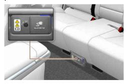
V2L (Vehicle to Load) is installed under the rear seat. V2L is a convenient feature which provides enough electricity to use diverse household electrical appliances in the vehicle. For more information, refer to the Using V2L function.
