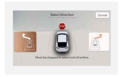
With the vehicle stopped by depressing the brake pedal, touch the infotainment system to select the desired exit direction.
