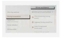
With the vehicle on, if **Setup > Vehicle > Driver assistance > Driving convenience > SCC (Smart Cruise Control)**) is selected in the infotainment system, you can change the vehicle distance, the acceleration, and the reaction speed manually.
