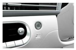
Whenever the front door is opened, the Start/Stop button illuminates and goes off a few seconds after the door is closed.
