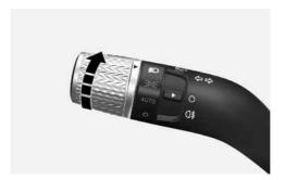
The headlight, position light, license plate light and instrument panel light are turned ON when you turn the knob to the  $\bigcirc$  position with the Start/Stop button in the POWER ON position.
