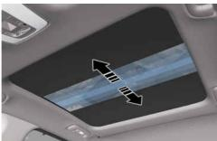
The power sunshade can only be operated when Start/Stop button is in the POWER ON or DRIVE READY position.
