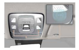
•  $\gg$ ,  $\searrow$ : Touch either icons to turn the map lamp on or off. This light produces a spot beam for convenient use as a map lamp at night or as a personal lamp for the driver and the front passenger.
