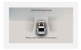
When RSPA is not working properly, the 'Check Parking Assist' warning message appears on the infotainment system. If the message appears, stop using RSPA, and we recommend that your vehicle be inspected by an authorised retailer of Genesis Branded products.
