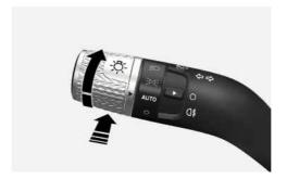
HBA automatically adjusts the headlights between high beam and low beam depending on the light detected from oncoming vehicles or vehicles in front using the front view camera.
