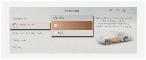
Set the charging current when using an AC charger.
