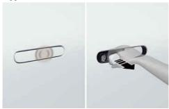
Touch the front door lock/unlock sensor (engraved part) on the front outside door handles.
