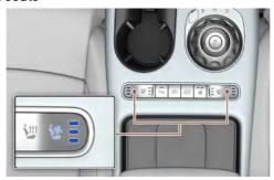
Whilst the vehicle is running, press the air ventilation switch to cool the driver's seat or front passenger's seat.
