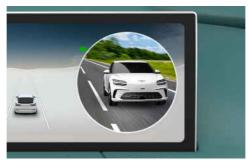
When the left or right side turn signal turns on, the image in that direction appears on the instrument cluster.
