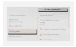
With the vehicle on, select **Setup > Vehicle > Driver assistance > Driving safety** from the settings menu in the infotainment system to set whether to use each function.
