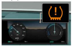
The TPMS Malfunction (1) Indicator illuminates after it blinks for about one minute when there is a problem with the TPMS. We recommend that the system be inspected by an authorised retailer of Genesis Branded products as soon as possible.
