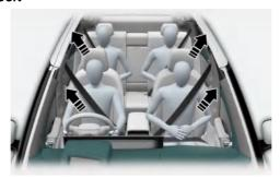
Your vehicle is equipped with driver's, front passenger's and rear passenger's pretensioner seat belts (retractor pretensioner). The pretensioner makes sure the seat belts fit tightly against your body in certain frontal or side collision(s). The pretensioner seat belts may be activated in crashes where the frontal or side collision(s) is severe enough, together with the airbags or sometimes it activate alone when wearing a seat belt.
