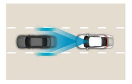
HDA function helps maintain the set speed and distance from the vehicle ahead, and helps centre your vehicle in the lane.
