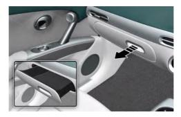
To open, pull the lever. Always close the glove box door after use.
