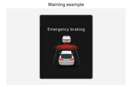
The warning lights of each operating system (Forward Safety ♣, Emergency Steering ₤, Lane Safety /♠\, Intelligent Speed Limit Assist ⊕, and Inattentive Driving ₺ warning light) also illuminates on the instrument cluster. For more information, refer to each system information in this chapter.
