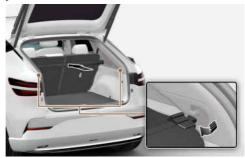
Pull the cargo security screen backward and up to release it from the guides.
