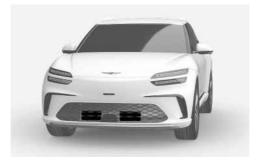
AAF system controls the air flap below the front bumper to cool the vehicle parts and improve energy efficiency.
