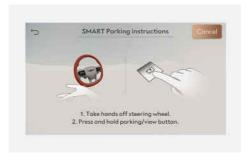
If RSPA cannot activate Remote Parking function, only the Smart Parking guide appears on the infotainment system.
