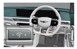
When pressing the illumination control button, the interior switch illumination intensity is also adjusted.
