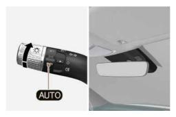
The position light and headlight are turned ON or OFF automatically depending on the amount of daylight as measured by the ambient light sensor at the upper end of the windscreen glass.
