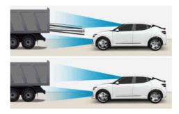
If the vehicle in front of you has cargo that extends rearward from the cab, or when the vehicle in front of you has higher ground clearance, additional special attention is required.
