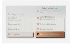
With the vehicle on, select Setup > Vehicle > Driver assistance > Parking safety > Rear cross-traffic safety from the settings menu in the infotainment system to turn on RCCA and deselect to turn off the function.
