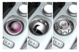
If the READY indicator is on and it cannot rotate normally in shift dial mode, try restarting the vehicle by pressing the start/stop button. If the same phenomenon repeats after
