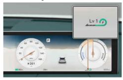
The selected regenerative braking level appears on the instrument cluster. When the vehicle is turned off and on again after the regenerative braking level is lowered to 0, the braking level changes to 1.
