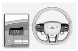
Press the Driving Assist (3) button briefly to turn on or off SCC.
