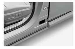
The vehicle certification label attached on the right front seat side centre pillar gives the VIN.
