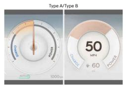
The CHARGE/POWER gauge displays the charging and discharging status of the electric energy produced by the regenerative braking and the energy consumption of the electric motor.
