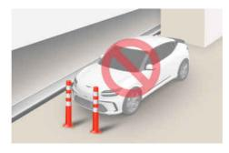
RSPA performance may be reduced or collision with an obstacle may occur when there is a narrow object, circular pillar, square pillar, or a pillar surrounded by objects such as a fire extinguisher, etc., near the parking space. Park or exit your vehicle manually.
