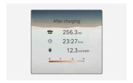
Trip distance, total driving time, average energy consumption, and instant energy consumption after the vehicle has been recharged are displayed.
