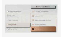
With the vehicle on, select **Setup > Vehicle > Driver assistance > Driving safety > Safe exit** from the Settings menu to turn on SEW and deselect to turn off the function.
