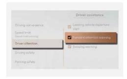
With the vehicle on, select **Setup > Vehicle > Driver assistance > Driver attention > Forward attention warning** in the infotainment system to set whether to use the function.
