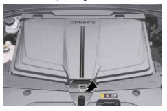
2 Remove the cover by pulling the front boot handle.
