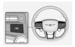
With the vehicle on, shortly press the Lane Driving Assist /
