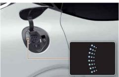
Check the State of Charge (SOC) of the high voltage battery via the charge indicator light inside the charging door with the vehicle door unlocked.
