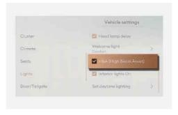
With the Start/Stop button in the DRIVE READY position, select **Setup** > **Vehicle** > **Lights** > **HBA** (**High Beam Assist**) from the Settings menu to turn on HBA and deselect to turn off the function.
