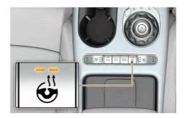
When the vehicle is running, press the steering wheel heater button to warm the steering wheel.
