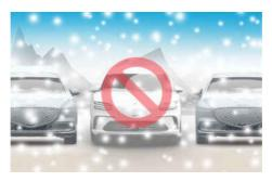
Snow may interfere with the operation of the ultrasonic sensor and wide view camera, or RSPA may cancel if the road is slippery whilst parking.
