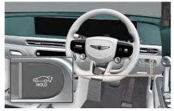
When the tailgate is open or closed, press the power tailgate open/close button for 1 second. The tailgate will open or close with a warning sound.
