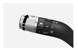
The position light, license plate light, and instrument panel light are turned ON when you turn the knob to the  $\ni \in$  position.
