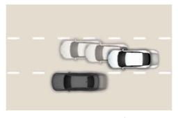
When your vehicle speed is above 40 mph (60 km/h), if a detected vehicle around you is driving at a close distance, your vehicle controls steering in the opposite direction of the vehicle to assist in safe driving. If there a detected vehicle in both sides of the lane that are driving close to you, the function does not veer to the opposite side of the lane.
