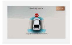
When the vehicle is stopped by depressing the brake pedal, the vehicle sensors detects the distance from nearby objects and check for space to exit.
