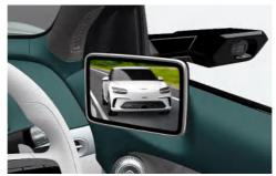
The digital side mirrors are a replacement for the outside rearview mirrors and help with changing lanes by displaying the rear view image on the monitors inside the vehicle.
