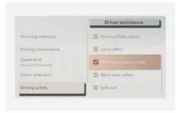
With the vehicle on, select Setup > Vehicle > Driver assistance > Driving safety and then enable Blind-spot view monitor in the infotainment system to turn on the BVM feature.
