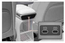
When in 'DRIVE READY', 'POWER ON' or utility mode, you can charge various devices such as smartphones and tablets by connecting them to the USB charging terminal.
