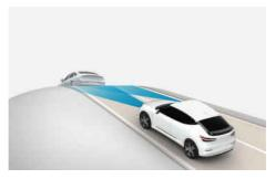
During uphill or downhill driving, the SCC may not detect a moving vehicle in your lane, and cause your vehicle to accelerate to the set speed. Also, vehicle speed rapidly decreases when the vehicle ahead is detected suddenly. Select the appropriate set speed on inclines and apply the brake pedal or accelerator pedal according to the road and driving conditions ahead.
