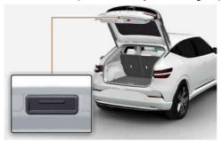
When the tailgate is closed, press the power tailgate open button to open the tailgate. If the vehicle is locked, press the power tailgate open button with the smart key or digital key in your possession.
