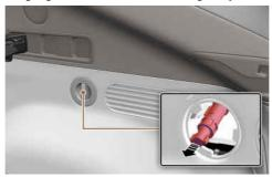
If the unlock button is not functioning properly due to a discharged battery or abnormal electrical wiring, the charging connector cannot be disconnected from the vehicle.
