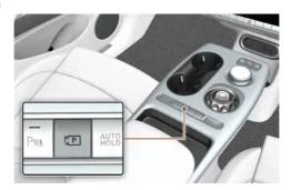
Press and hold the Parking/View TD button to turn on RSPA. Also, Parking Distance Warning (PDW) and Surround View Monitor (SVM) automatically turns on.
