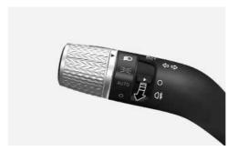
To turn on the rear fog light, turn the knob to the headlight position, and then turn the rear fog light switch to the rear fog light position.
