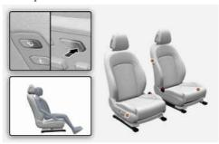
Press and hold the front portion of the Relaxation mode switch to return the seat to the original position.
