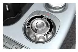
To shift the gear to N (Neutral), rotate the rotary gear shift dial to N (Neutral) whilst depressing the brake pedal.
