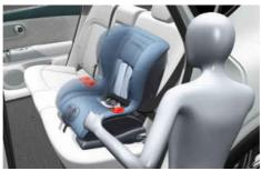
If your Child Restraint System manufacturer instructs or recommends you to use a top tether anchorage with the lap/shoulder belt, refer to the Securing a Child Restraint System seat with Top Tether Anchorage system.
