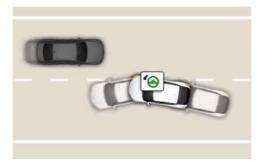
When changing lanes, Lane-Change Oncoming function helps avoid a collision with an oncoming vehicle or motorcyclist by warning or assisting the driver's steering.
