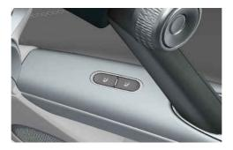
The IMS for the driver's seat is equipped on some models and allows the driver to store and recall the following memory settings with a simple button operation.
