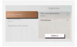
To delete all the registered digital key (smartphone), select **Setup** > **Vehicle** > **Digital key** > **Smartphone key** > **Delete all** from the infotainment system.
