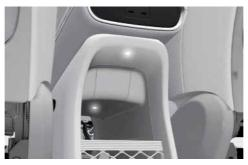
Console under tray lamp turns on when opening the door and turns off when turning off the vehicle and locking the door.
