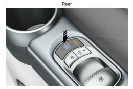
Whilst the vehicle is running, press the seat warmer switch to warm the seat.
