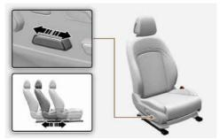
Push the control switch forward or rearward to adjust the seat to the desired position.
