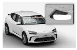
The rain sensor located on the upper end of the windscreen glass senses the amount of rainfall and controls the interval of the wiping cycle.
