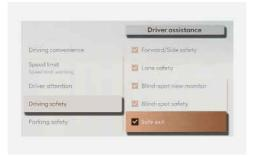
With the vehicle on, select Setup > Vehicle > Driver assistance > Driving safety > Safe exit from the Settings menu to turn on SEA and deselect to turn off the function.
