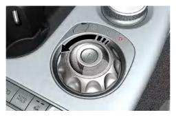
To shift the gear to D (Drive), rotate the rotary gear shift dial to D (Drive) whilst depressing the brake pedal.
