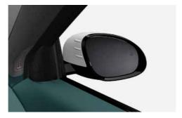
The mirrors can be adjusted with the mirror adjustment control switch. Adjust the outside rearview mirrors to your desired position before driving. The outside rearview mirrors can be folded to help prevent damage when going through an automatic car wash or when passing through a narrow street.
