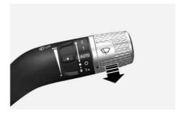
In the **O** position, pull the lever gently toward you to spray washer fluid on the windscreen and to run the wipers 2-3 cycles. The spray and wiper operation continues until you release the lever. If the washer does not work, you may need to add washer fluid to the washer fluid reservoir.
