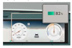
The SOC gauge shows the charging status of the high voltage battery.
