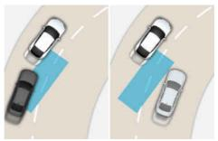
BCA may not operate properly when driving on a curved road. The function may not detect the vehicle in the next lane or the function may recognise a vehicle in the same lane.
