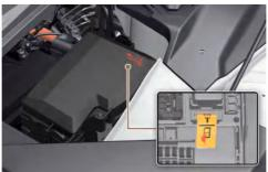
High voltage cut-off switch is a device located inside the motor compartment to block the battery's high voltage when your vehicle is inspected at an authorised retailer of Genesis Branded products.
