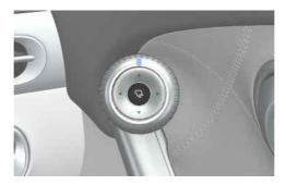
The outside rearview mirrors can be folded or unfolded by pressing the button.
