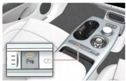
Press the Parking Safety P™ button to turn on PDW. Press the button again to turn off the function.
