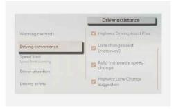
With the vehicle on, select **Setup > Vehicle > Driver assistance > Driving convenience > Auto motorway speed change** from the Settings menu to turn on NSCC or deselect to turn off the function.
