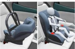
There are three main types of Child Restraint Systems: rearward-facing, forward-facing, and booster seat Child Restraint Systems.
