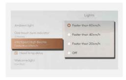
With the Start/Stop button in the DRIVE READY position, select Setup > Vehicle > Lights > Intelligent High Beams from the Settings menu to turn on Intelligent Front-Lighting System and deselect to turn off the system.
