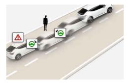
When there is a risk of collision with a subject ahead in the same lane, Evasive Steering Assist function helps avoid a collision by warning or assisting the driver's steering.
