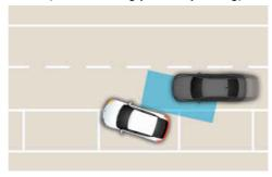
When the driver turns the steering wheel about one turn to exit the vehicle forward, if there is a risk of collision, warning (with warning light, warning message, warning sound, and steering wheel vibration) and braking activates under the following conditions:
