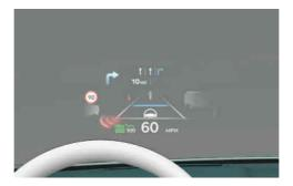
The HUD is an optional feature that allows the driver to view information projected onto a transparent screen whilst still keeping your eyes on the road ahead whilst driving.
