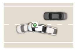
When changing lanes, Lane-Change Side function helps avoid a collision with the vehicle or motorcyclist ahead in the next lane by warning or assisting the driver's steering.
