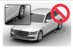
Never start or run the vehicle whilst an AWD vehicle is raised on a jack. The vehicle may slip or roll off of a jack causing serious injury or death.
