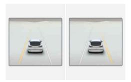
To warn the driver that the vehicle is departing from the projected lane in front without activating the turn signal, the green indicator light blinks on the instrument cluster, and the steering wheel makes adjustments to keep vehicle inside the lane.
