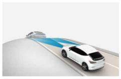
FCA may not detect a vehicle, motorcyclist, pedestrian, or cyclist in front of you whilst driving uphill or downhill, adversely affecting the performance of the sensors. This may result in no warning, braking assist or steering assist (if equipped) when necessary.
