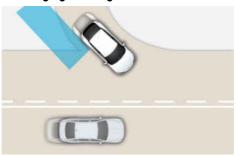
BCA may not operate properly when driving where the road merges or divides. The function may not detect the vehicle in the next lane.
