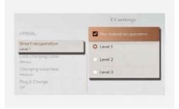
Select Electric vehicle > @ (EV settings) > Smart recuperation in the infotainment system and set the driver's distance level (Level 1/Level 2/Level 3) at the smart regenerative braking distance phase, and a distance from the leading vehicle is adjusted according to the setting.
