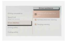
With the vehicle on, select **Setup** > **Vehicle** > **Driver assistance** > **Driver attention** and then enable **Leading vehicle departure alert** in the infotainment system to use the function.
