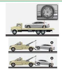
Notice: The use of wheel dollies or flatbed is recommended. Use a wheel lift or flatbed equipment.
