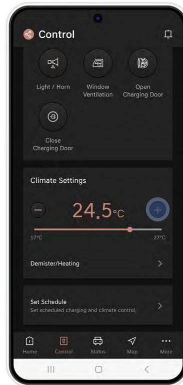
The temperature can be adjusted by pressing the (-) or (+) buttons or by the slide bar.
