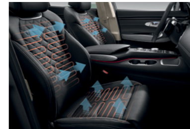
Front Seat Warming & Air Cooling Ventilation
