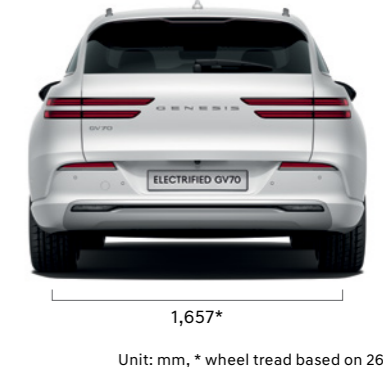
Unit: mm, * wheel tread based on 265/45R20 tyres
