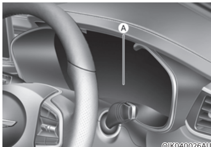
[A] : Interior view camera
