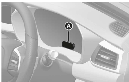
[A] Interior view camera
