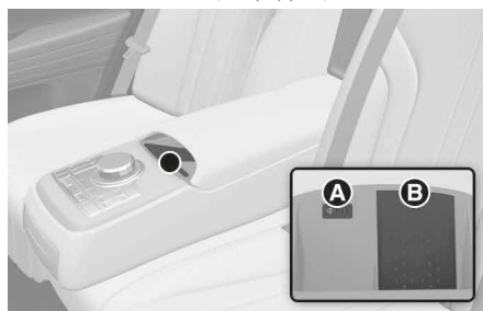
[A] Indicator light [B] Charging pad
