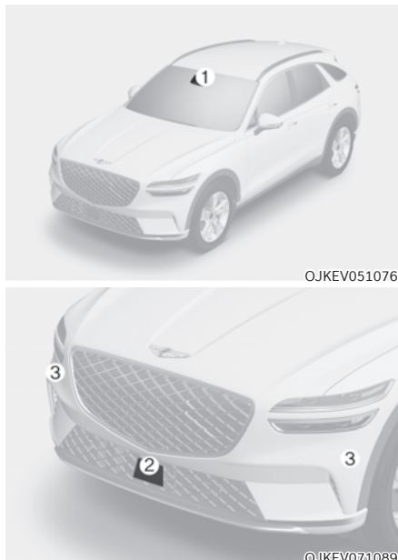
[1]: Front view camera, [2]: Front radar [3]: Front corner radar (if equipped)
