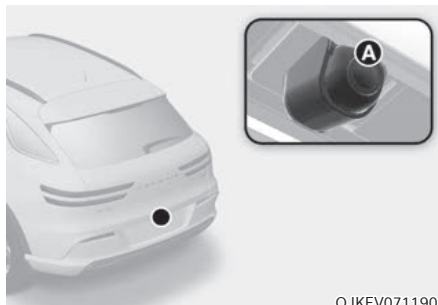
[A]: Wide angle-rear view camera
