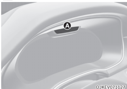
[A] : Interior view camera
