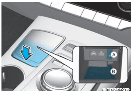
[A] : Indicator light, [B] : Charging pad
