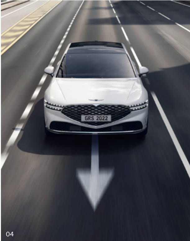
04. Lane Keeping Assist (LKA) system _ It warns the driver when the vehicle departs from its lane without the use of turn signals and automatically helps steering to keep the vehicle in its lane.
