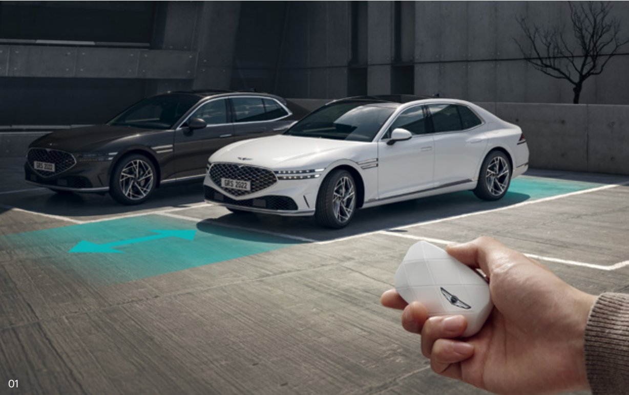
01. Remote Smart Parking Assist (RSPA) (Wide-Angle Camera-Based) The wide-angle camera based Remote Smart Parking Assist (RSPA) supports perpendicular parking, parallel parking and diagonal parking by recognizing parking lines.
