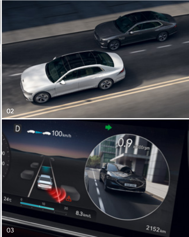
02. Blind-Spot Collision-Avoidance Assist (BCA) system _ When the turn signals are operated to change lanes, this system warns the driver if there is a collision risk with a vehicle in the back. If the collision risk increases after the warning, it applies emergency braking. If a possible collision is detected while the vehicle is leaving a parallel-parked position, the system automatically helps to activate the brakes. 03. Blind-Spot View Monitor (BVM) system _ When the turn signals are activated, video images of the respective side/rear view of the vehicle appear on the center cluster.
